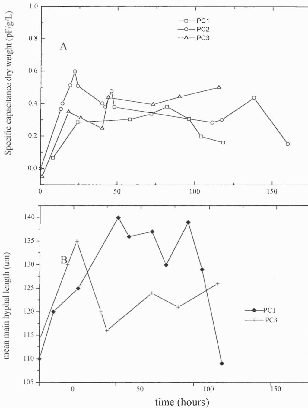
Figure 5.11: Specific capacitance dry weight (pF/g/L) and mean main hyphal length (μm) versus time *Penicillium chrysogenum* P1 5L fermentations PC1-3
