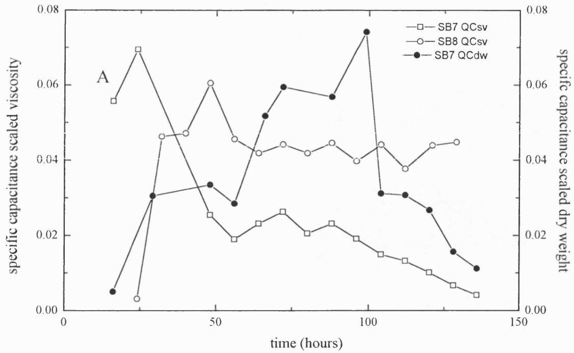
Figure 5.14: specific capacitance scaled viscosity and specific capacitance scaled dry weight versus time *Streptomyces sp* pilot scale fermentations SB7 and 8
