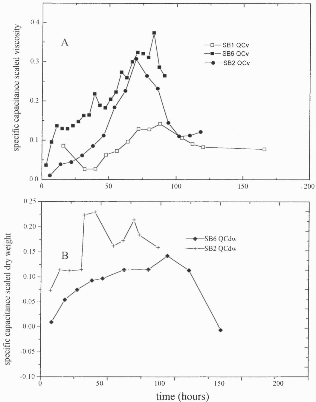
Figure 5.13: specific capacitance scaled dry weight and specific capacitance scaled viscosity versus time *Penicillium chrysogenum* laboratory and production scale fermentations SB1,2 and 6
