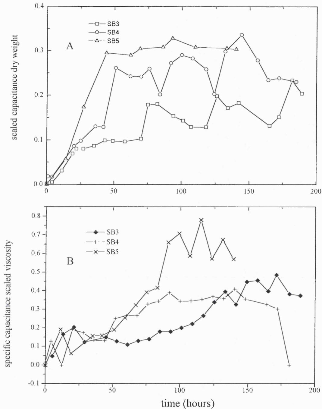
Figure 5.12: specific capacitance, scaled dry weight and scaled viscosity versus time *Penicillium chrysogenum* pilot scale fermentations SB3,4 and 5
