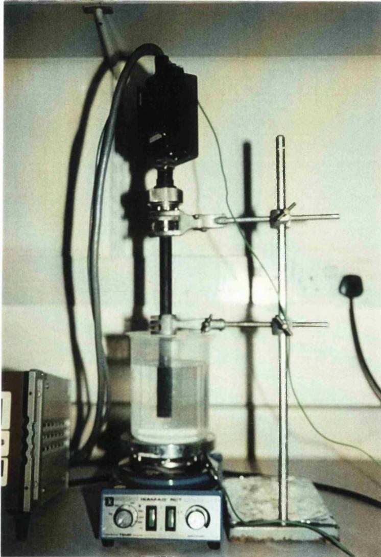
Figure 3.1a: Off-line set up of 19mm probe
