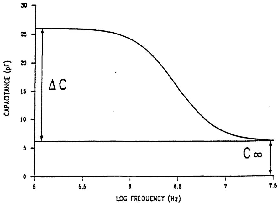
Figure 2.1: Idealised plot of capacitance (pF) versus log frequency (Hz) adapted from Davey (1991)
