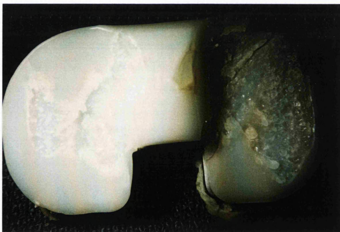
FIG.6 A retrieved delaminated tibial insert.
