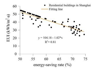
Fig. 6 Relationship between the EUI and the energy-saving rate for residential buildings in Shanghai.
