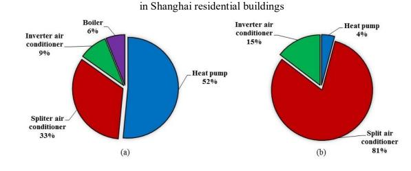
Fig. 11. HVAC systems of labeled residential buildings in Shanghai (a) buildings with EUI lower than 40 kWh/m<sup>2</sup>a; (b) buildings with EUI higher than 40 kWh/m<sup>2</sup>a.
