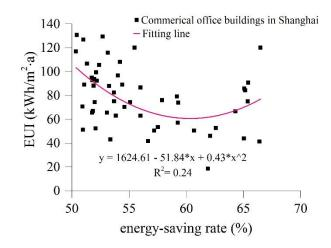
Fig. 5 Relationship between the EUI and the energy-saving rate for commercial office buildings in Shanghai.
