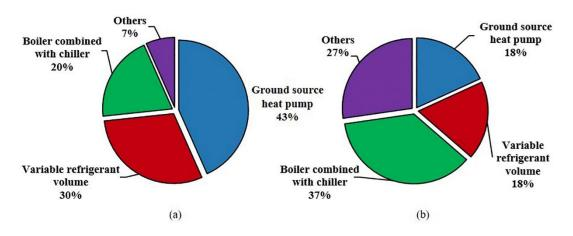
Fig. 9. HVAC systems of labeled commercial buildings in Shanghai (a) buildings with EUI lower than 80 kWh/m<sup>2</sup>a; (b) buildings with EUI higher than 80 kWh/m<sup>2</sup>a.
