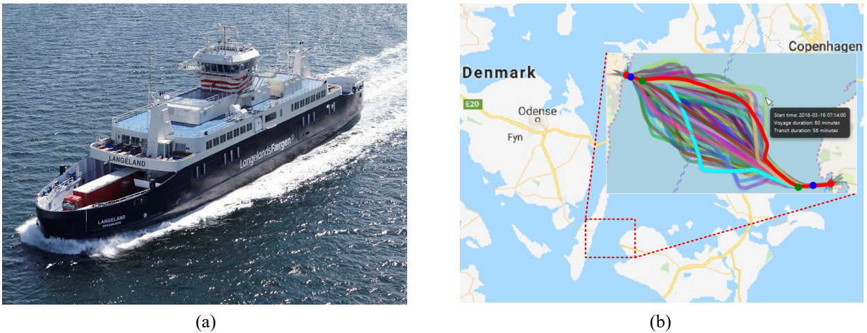
Figure 5: Candidate ship (a) and its route (b). The candidate ship is a passenger ferry with integrated full electric propulsion system, and operates between two fixed ports.
