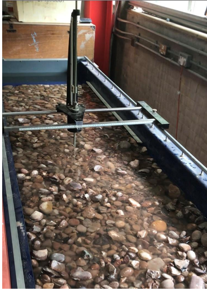
Figure 116 Water accumulated on top of the gravel bed
