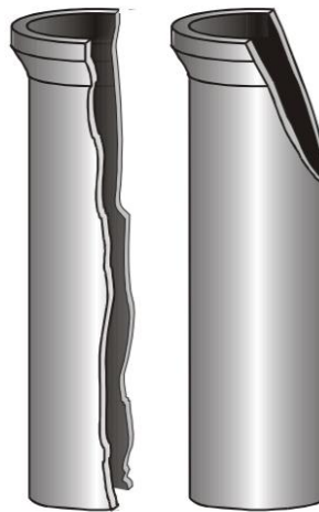
Figure 95 Failure Modes of large diameter cast-iron pipes (source: Makar et al., 2001) The left pipe indicates the longitudinal splitting failure and the right pipe indicates bell shearing failure
