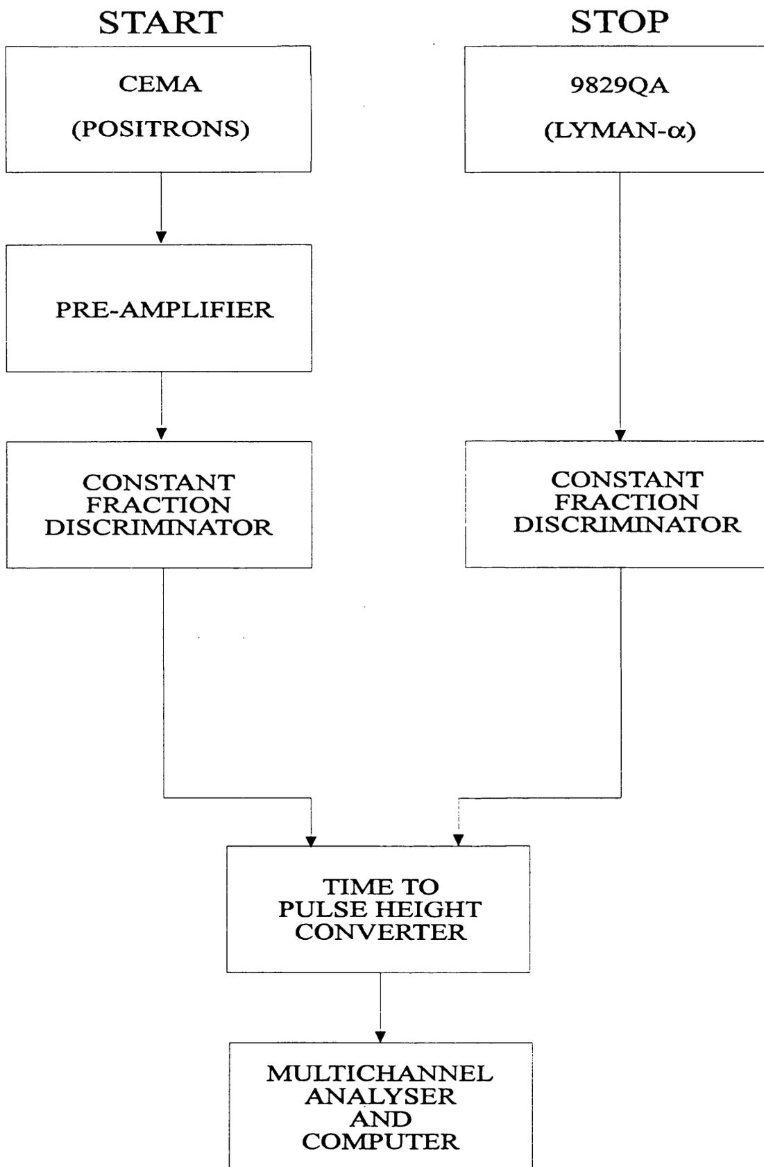
Figure 4.8 A block diagram of the timing electronics used in the radiative lifetime experiments.
