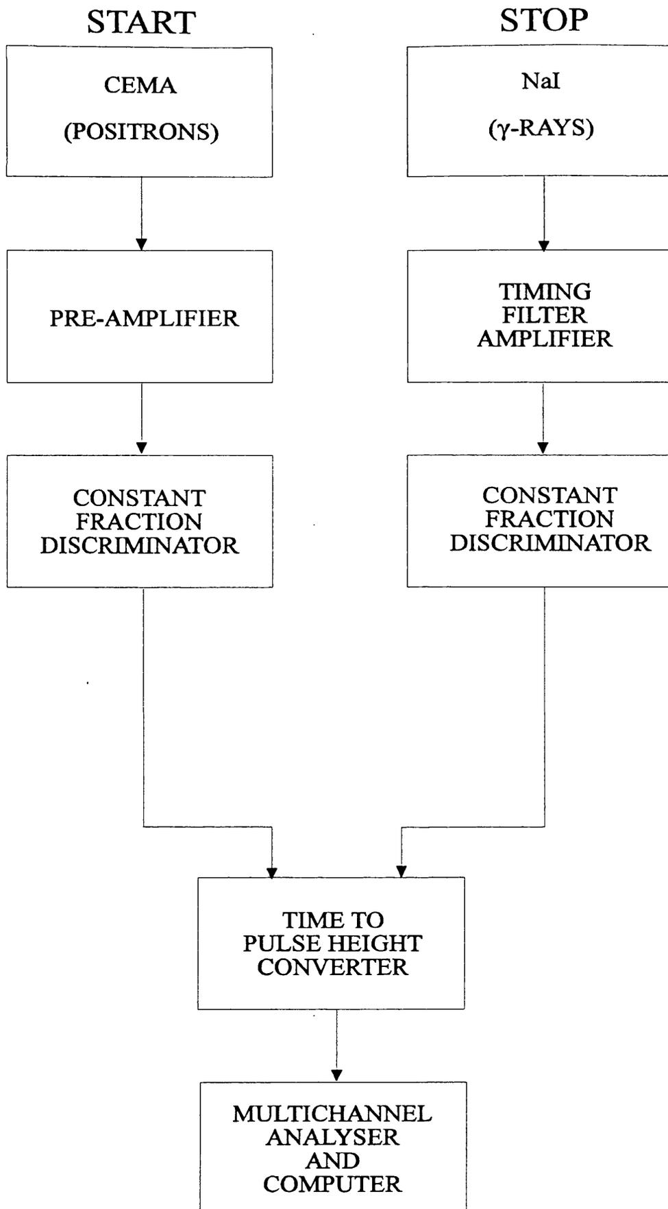
Figure 2.15 A block diagram of the timing electronics used to determine the CEMA detection efficiency.
