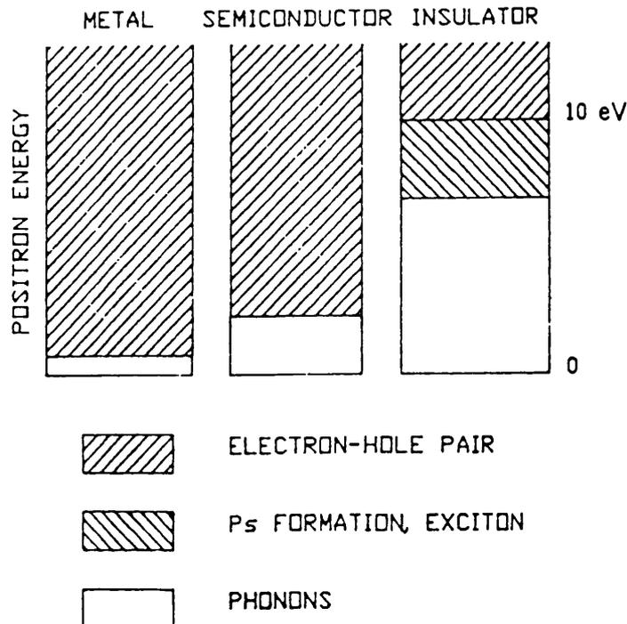
Figure 1.6 A schematic diagram showing the régime of positron energy loss processes in each class of solid (Schultz & Lynn (1988)).
