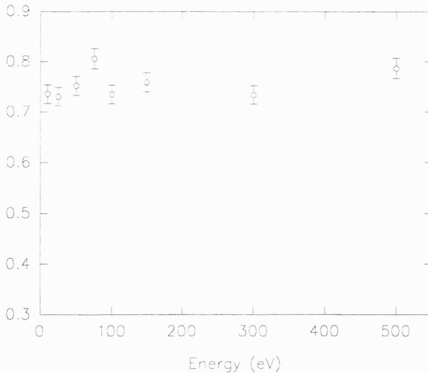
**Figure 3.31** The ratio of integrated counts in the 50-100nsec to the 100-1000nsec time regions, as a function of energy for positrons incident on the Be target.
