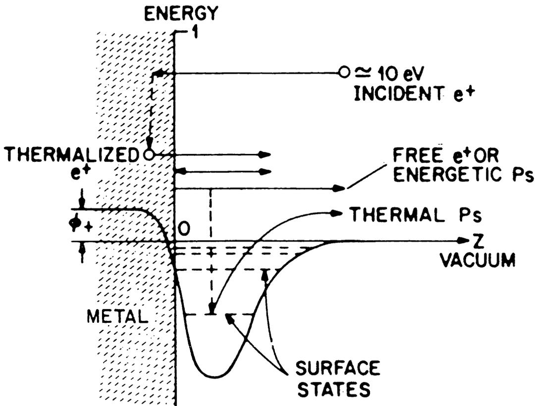
Figure 3.8 A schematic diagram of the surface potential as seen by a surface bound Ps atom.
