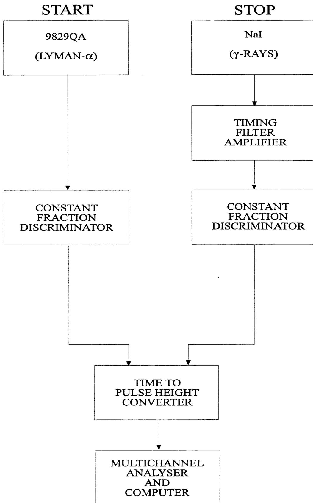
Figure 3.24 A block diagram of the timing electronics used in the  $Ps^*$  production experiments.
