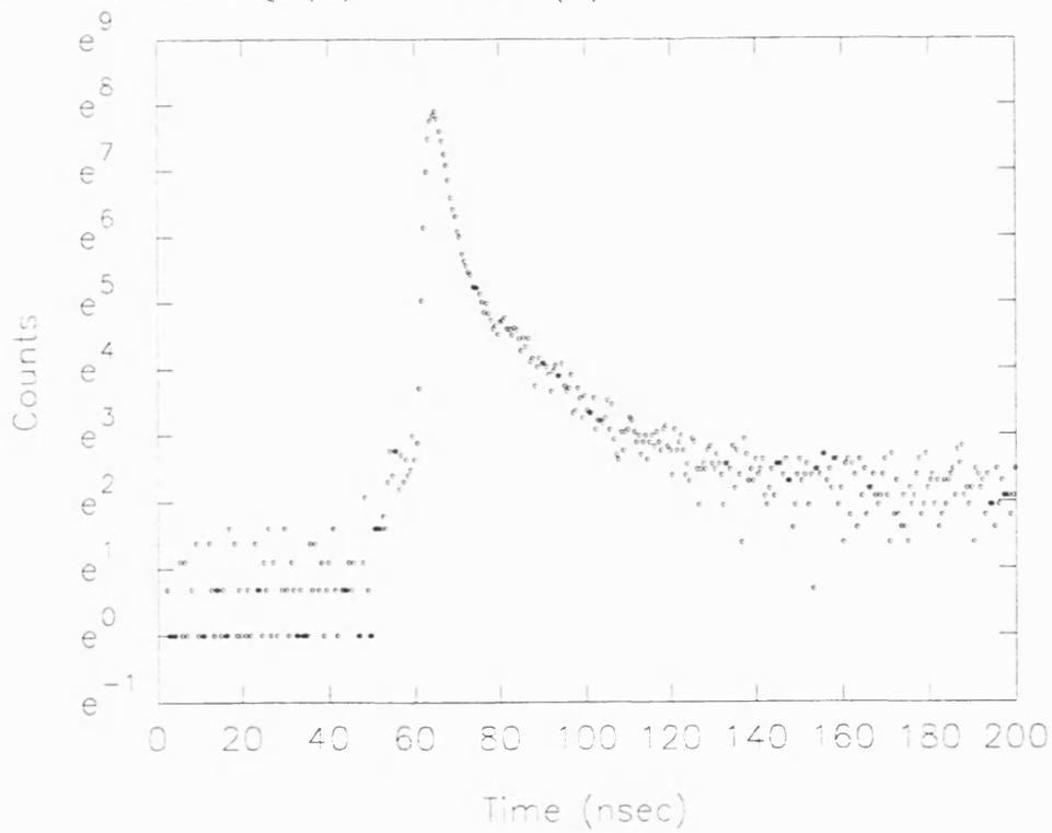
**Figure 4.11** Coincidence spectrum obtained by impacting 100eV electrons on MgO vanes with sphere in place.
