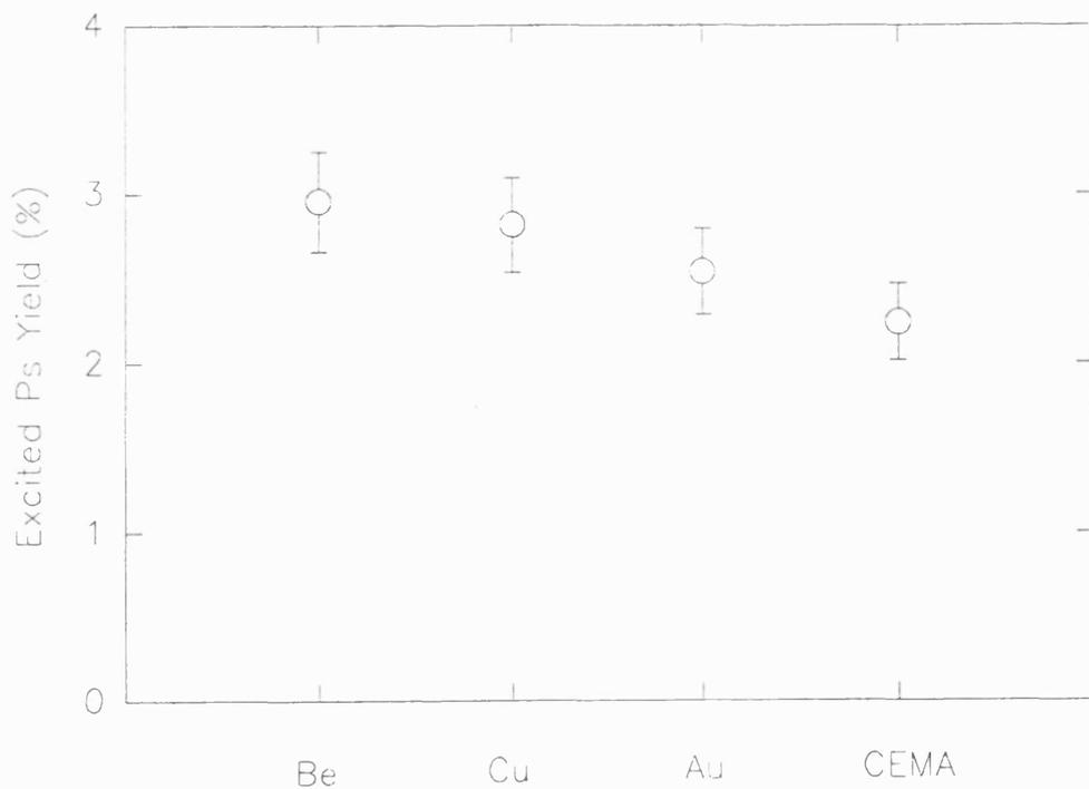
**Figure 3.33** Relative  $\text{Ps}^*$  yields for 100eV positrons incident on: Be, Cu, Au and a channel plate.
