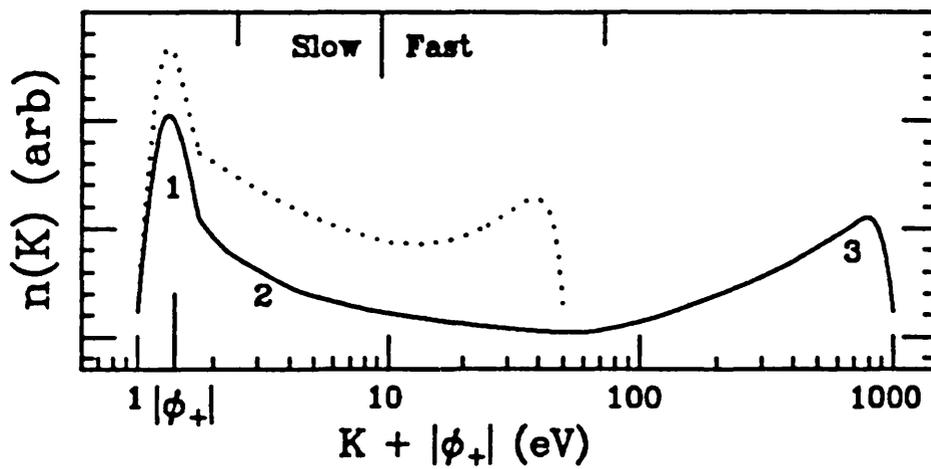
Figure 3.20 A composite curve showing the calculated energy distribution of positrons incident on a metal target at 1keV (—) and 50eV (·····) and subsequently re-emitted, after Fischer *et al* (1986).
