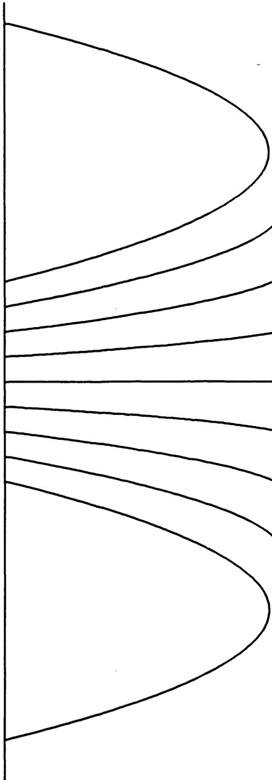
**Figure 3.36** SIMION simulation of 100eV positrons with angular deviations of up to  $20^\circ$  (in steps of  $5^\circ$ ), subject to retardation to 10eV at a target.
