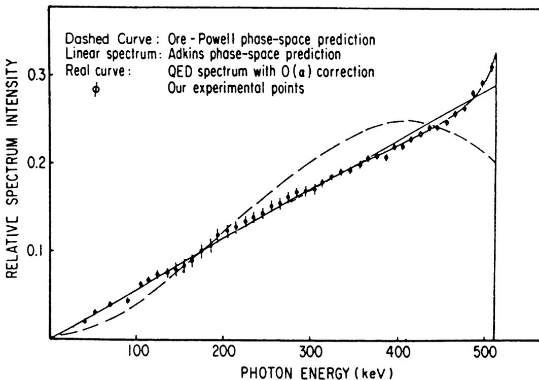
Figure 1.2 The energy distribution of  $\gamma$ -rays resulting from o-Ps decay (Ore and Powell (1949), Chang *et al* (1982,1985)).
