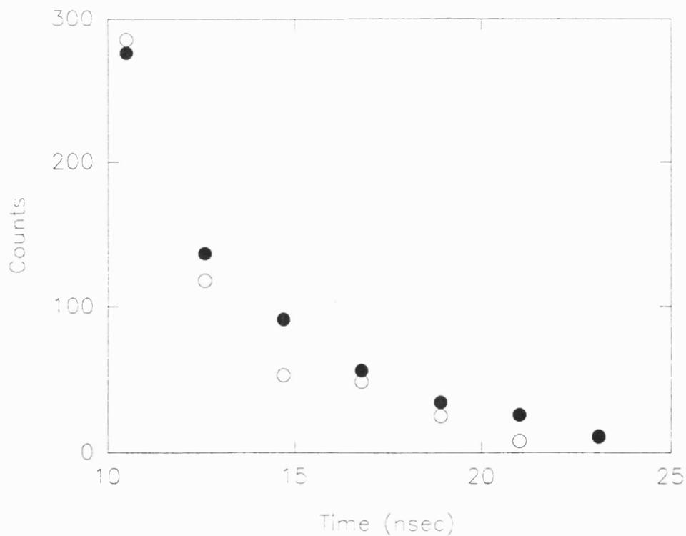
Figure 4.13 A composite coincidence spectrum obtained by impacting 100eV positrons on CuBe vanes with background light sources suppressed, with aluminium shutter in (○) and (●)out.
