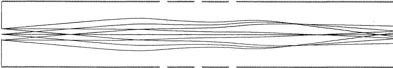
**Figure 2.9** A SIMION simulation of the 4-element lens operating at 100eV, for positrons at  $0^\circ$  and  $10^\circ$  to the beam axis.
