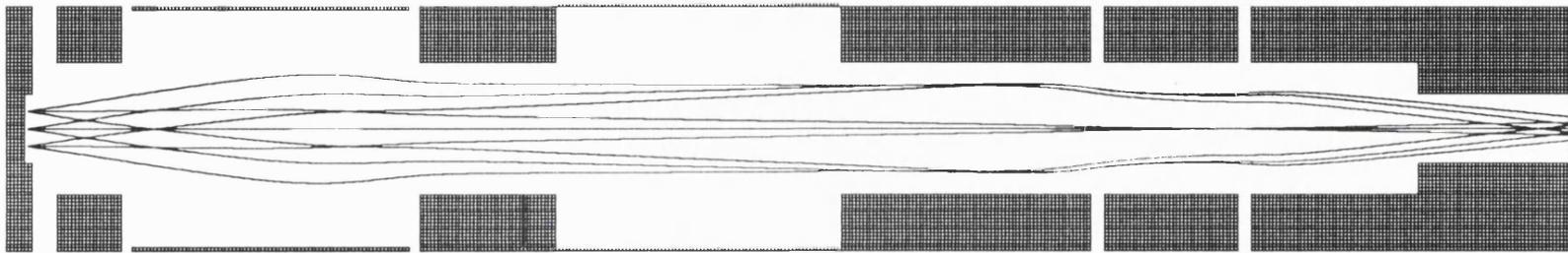
**Figure 2.5** A SIMION simulation of the Soa gun and 3-element lens operating at 100eV, for positrons at  $0^\circ$  and  $10^\circ$  to the beam axis.
