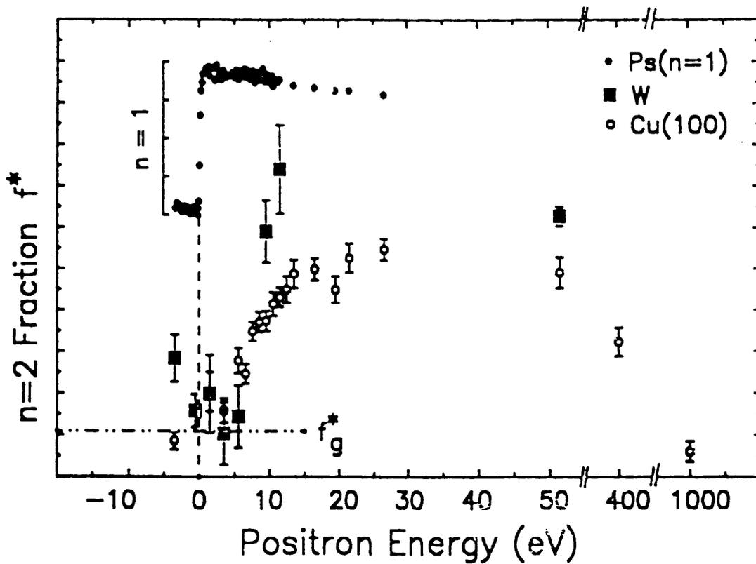
Figure 3.16 Measured Ps' fractions as a function of incident positron energy, from clean Cu and W surfaces (Schoepf *et al* (1992)).
