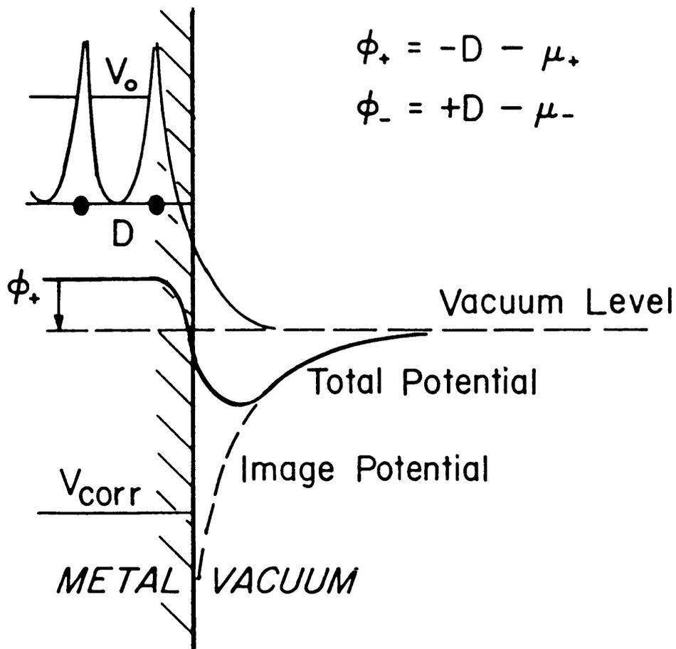
Figure 1.8 A schematic diagram of the potential energy as seen by a positron at a negative workfunction surface (Schultz & Lynn (1988)).
