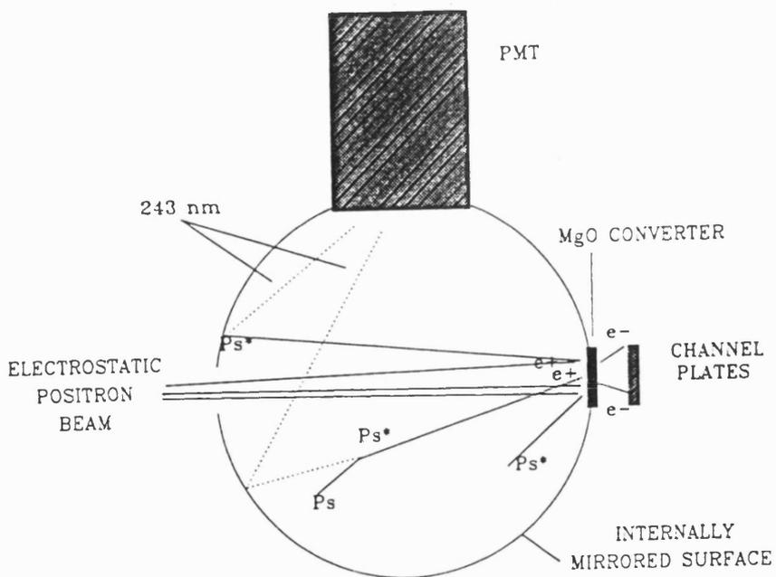
Figure 4.6 A schematic diagram of the reflective sphere and detector arrangement used in the radiative lifetime experiments.
