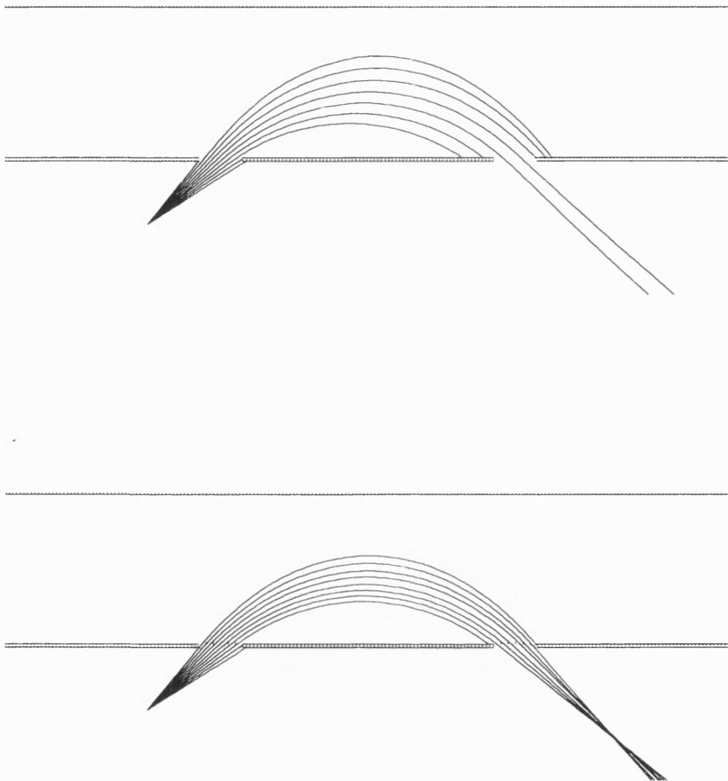
**Figure 2.8** SIMION simulation of the CMA operating at 100eV, for positrons with divergences of up to  $\pm 10^\circ$  from the 'magic angle' (in steps of  $2^\circ$ ). Without meshes over the input and output (top), and with meshes in place (bottom).
