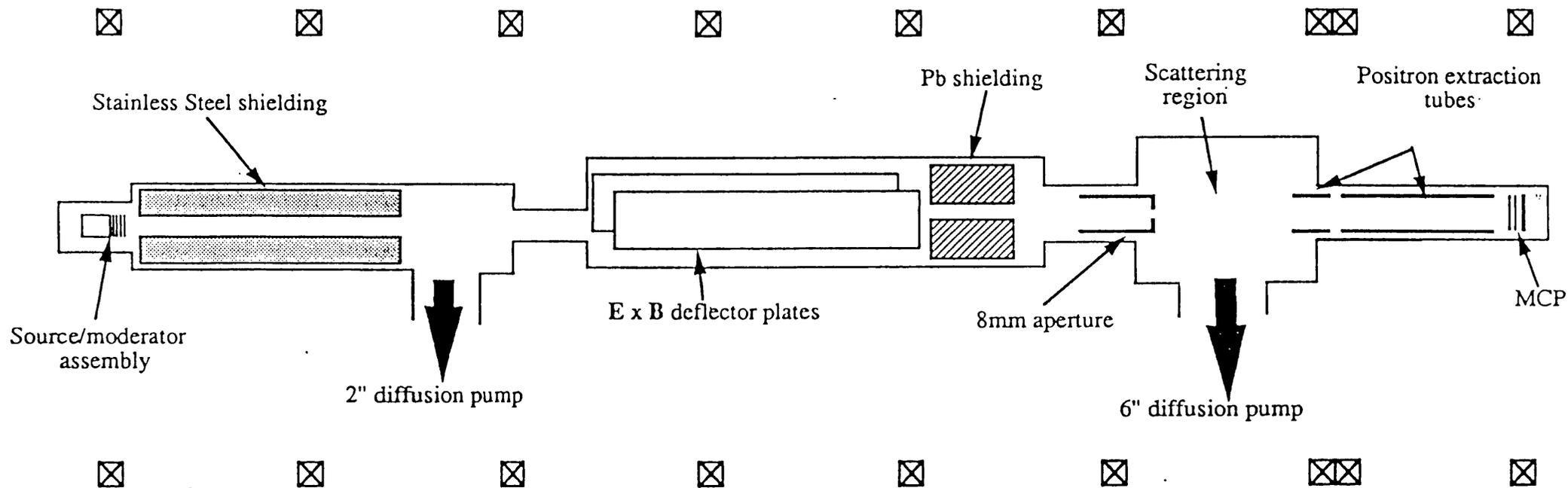
Figure 1.11 A schematic diagram of a typical magnetically guided positron beam.
