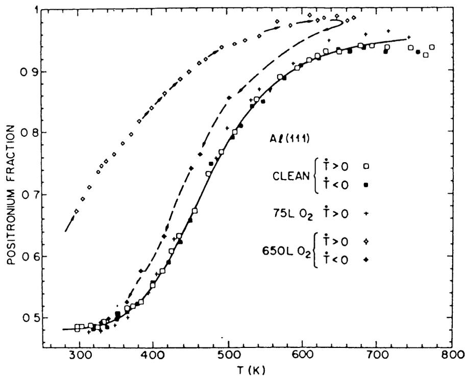
Figure 3.9 The temperature dependence of the Ps formation fraction from a clean aluminium surface (□, ■) (Mills & Pfeiffer (1985)).
