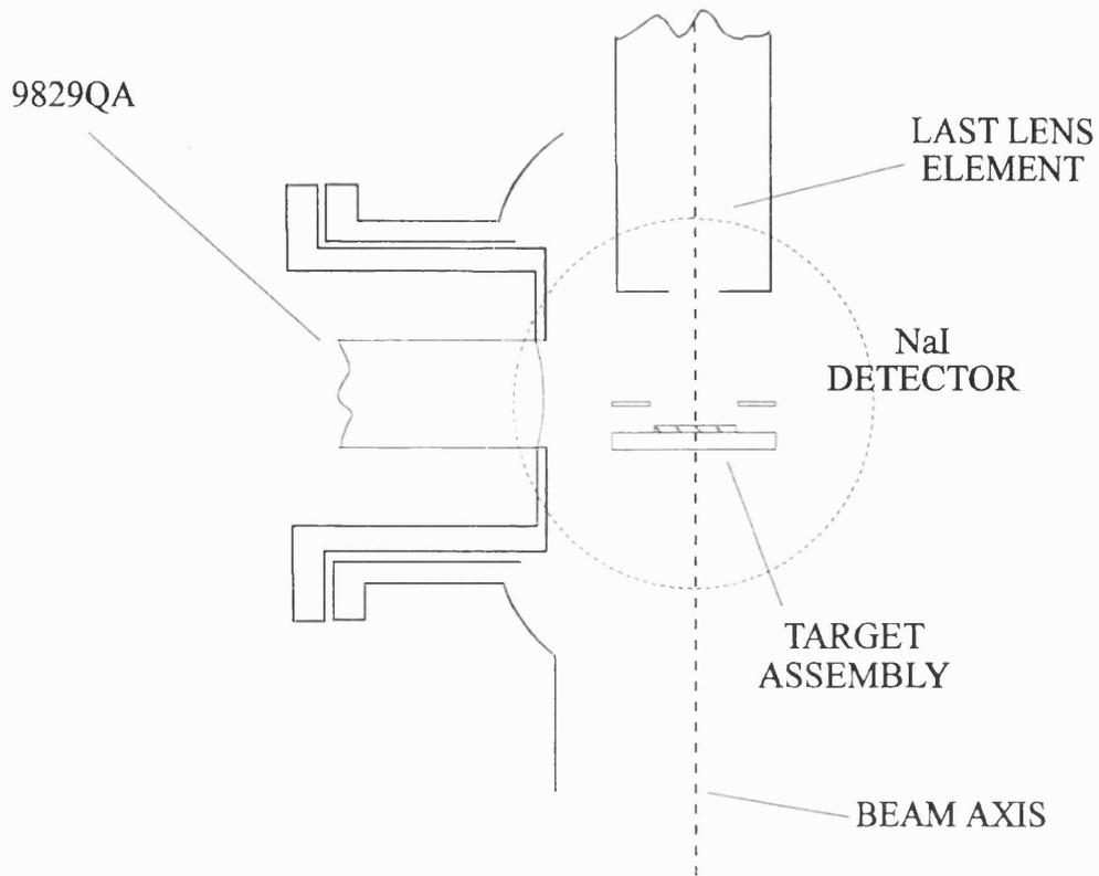
Figure 3.21 A schematic diagram of the interaction region in the  $Ps^*$  production experiments.
