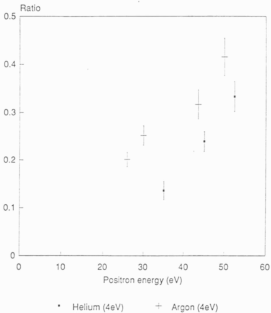
**Figure 3.7** The ratio of measured  $n=2$  to  $n=1$  Ps yield by positron impact with helium (■) and argon (+) for Ps in the 4eV kinetic energy region (Zafar *et al* (1991)).
