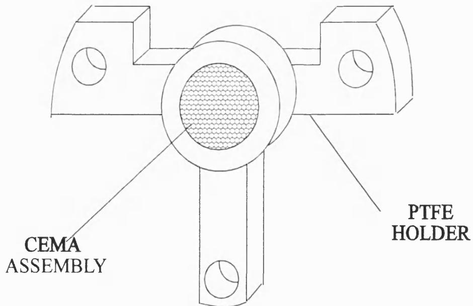
Figure 2.13 The CEMA arrangement and mount.
