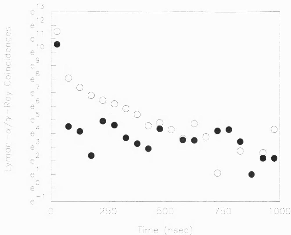
**Figure 3.25** Lyman- $\alpha$ / $\gamma$ -ray coincidence spectra for 100eV positrons incident on a Cu target with borosilicate slide in (●) and out (○).
