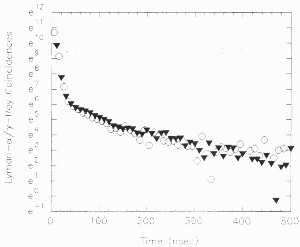
**Figure 3.30** A composite plot of the coincidence spectra obtained from positrons incident on Be at 25eV (O) and 300eV (▼).
