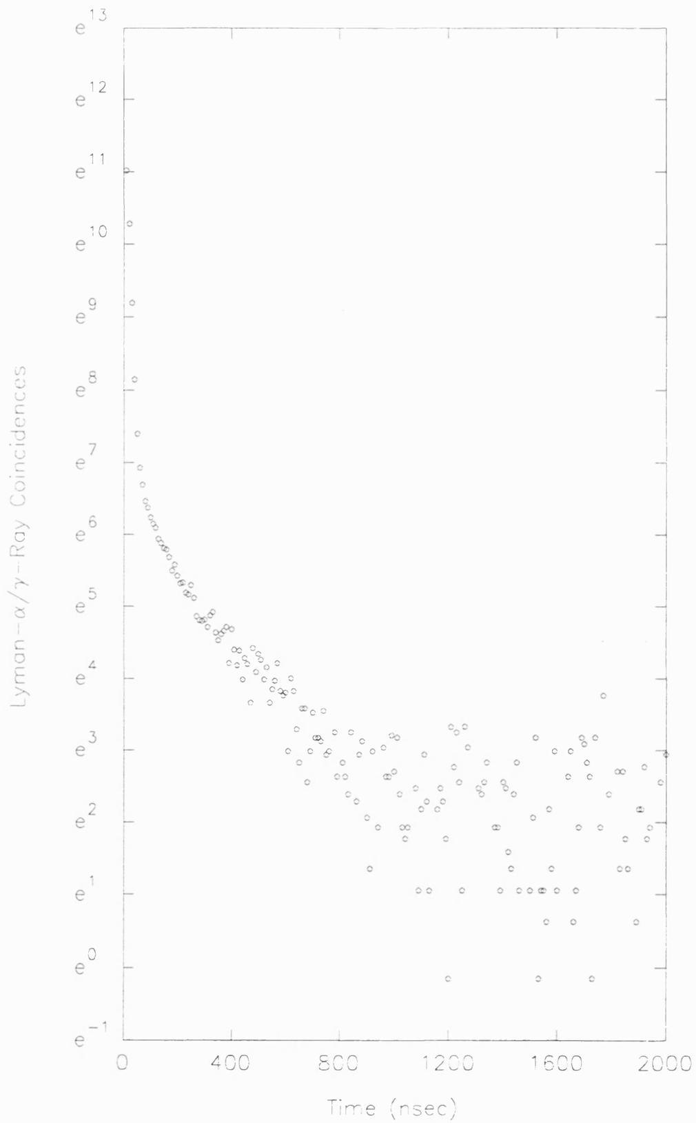
**Figure 3.28** An example of a typical coincidence spectrum, in this case 100eV positrons incident on Be. The data have been summed into ten channel bins and the background has been removed.
