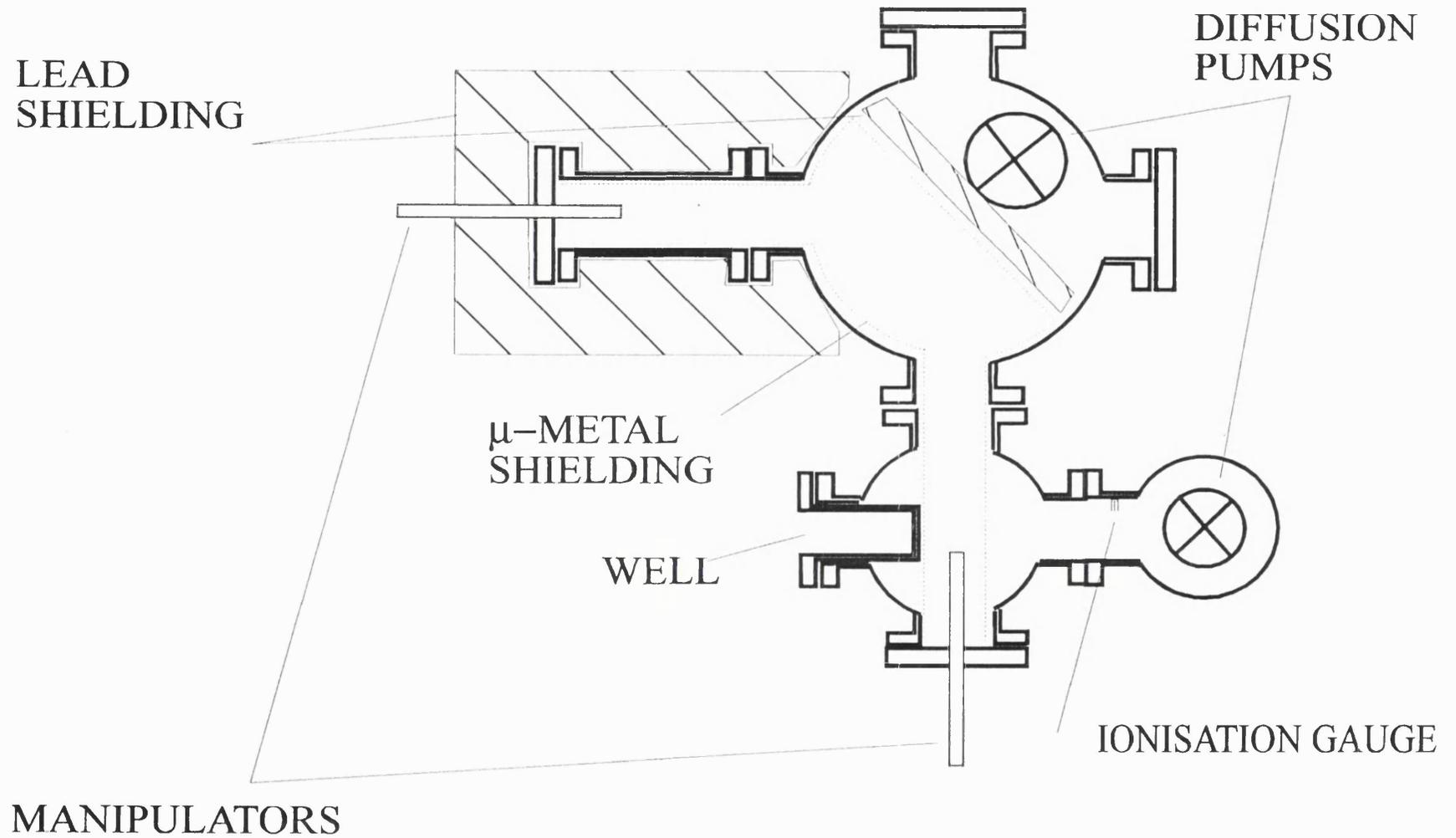
Figure 2.11 A schematic plan view of the vacuum chamber and lead shielding.
