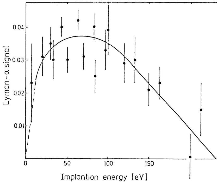
Figure 3.14 The Lyman- $\alpha$  count rate, as a function of energy, for positrons incident on a molybdenum target (Ley et al (1990)).
