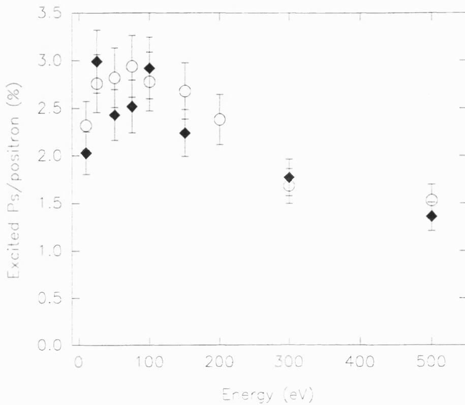
**Figure 3.32** Absolute  $\text{Ps}^*$  yields as a function of energy for positrons incident on Be (◆) and Cu (○) targets. The error bars are statistical only.
