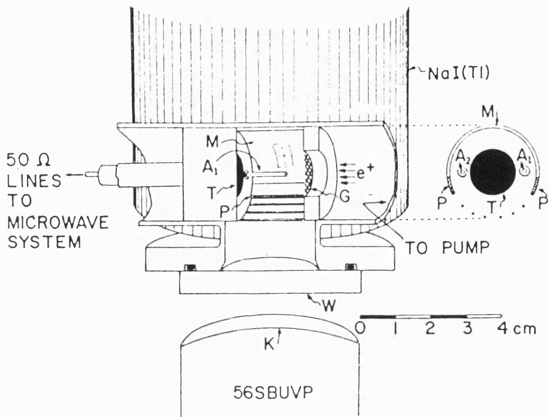
Figure 4.4 A schematic diagram of the apparatus used by Mills *et al* (1975) to measure the positronium  $2^3P_2$ - $1^3S_1$  fine structure interval.
