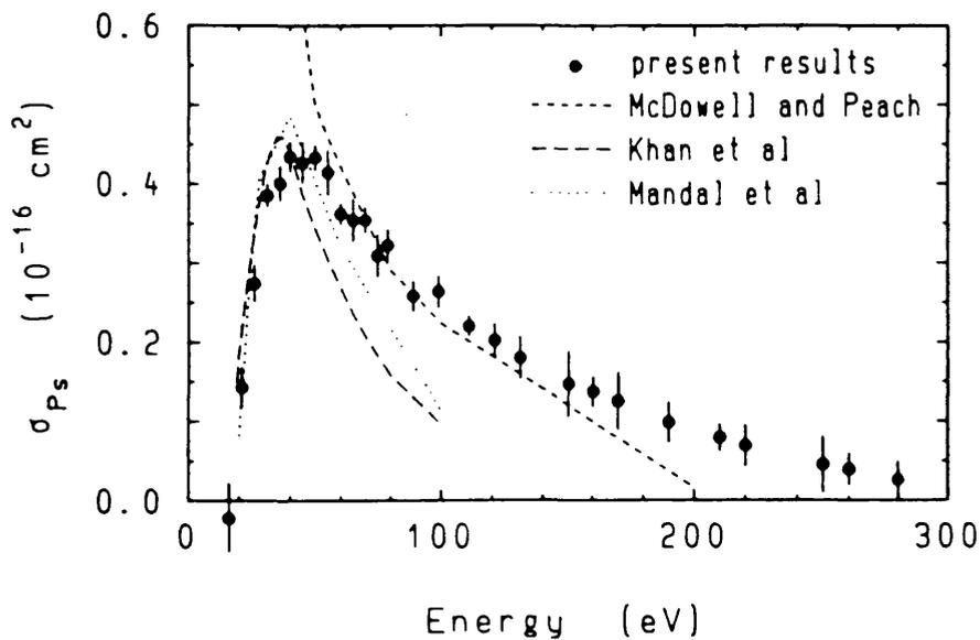
Figure 3.6 The Ps formation by positron impact with helium measurements of Fromme *et al* (1986) along with the theoretical treatments of Mandal *et al* (1979), Khan *et al* (1985) and McDowell and Peach (1985).
