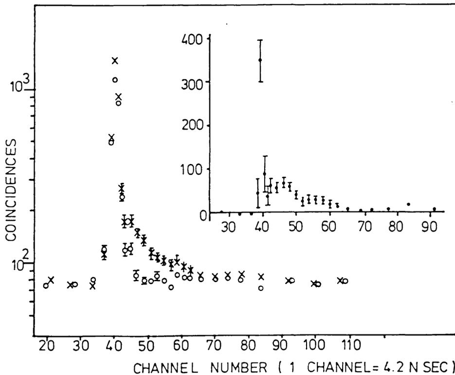
Figure 3.3 Timing spectra obtained by placing a Lyman- $\alpha$  detector in coincidence with a  $\gamma$ -ray detector (Canter *et al* (1975)).
