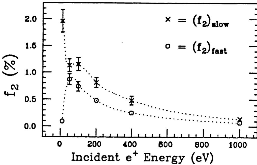
Figure 3.19 The summed fast and slow  $\text{Ps}^+$  components for all targets, plotted against positron impact energy (Steiger *et al* (1992)).
