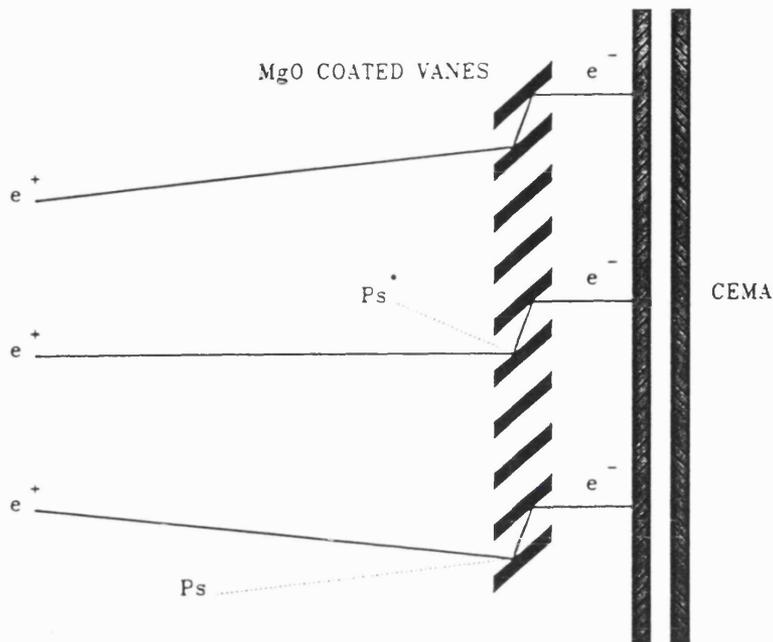
Figure 4.5 A schematic diagram of the positron timing arrangement used in the radiative lifetime experiments.
