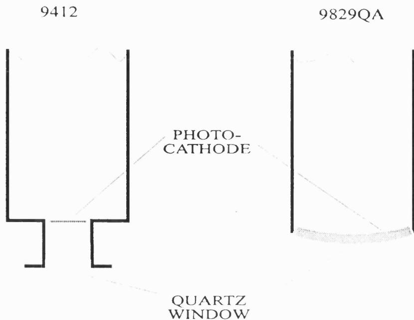
Figure 4.7 Schematic diagrams of the EMI 9412 and EMI 9829QA photomultiplier tubes.
