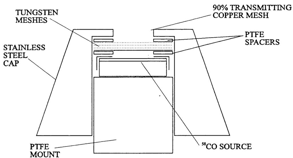
Figure 2.4 A schematic diagram of the source/moderator cap.
