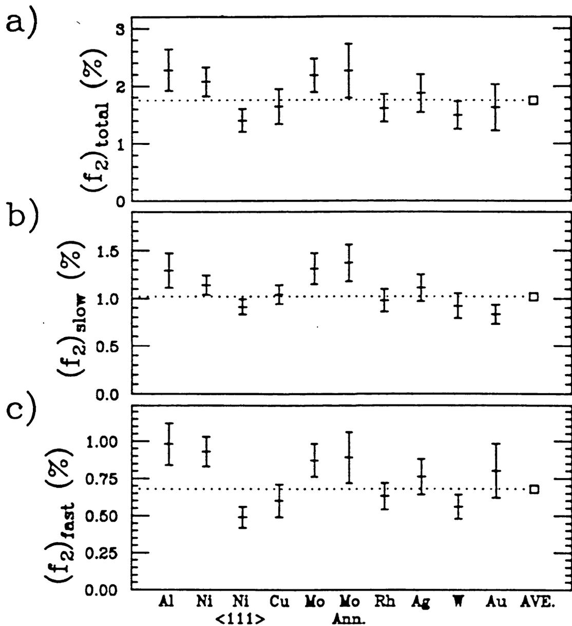
Figure 3.18 Total (a), slow (b) and fast (c) Ps\* yields from a range of targets subject to positron impact at 100eV (Steiger *et al* (1992)).
