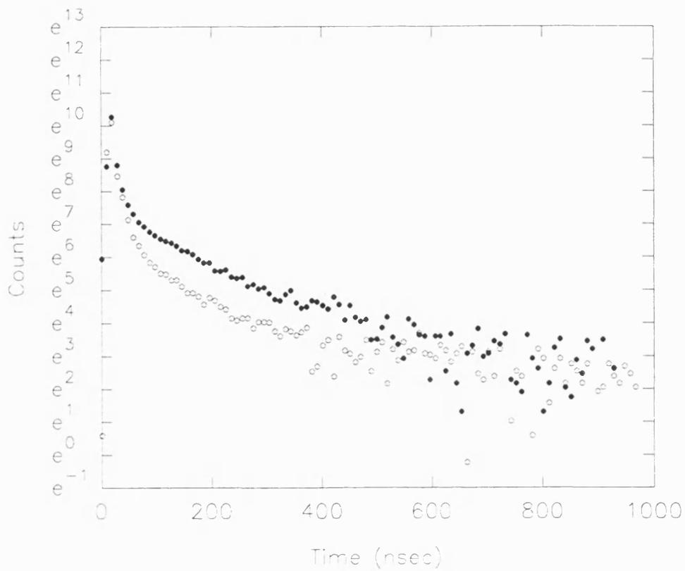
**Figure 4.10** Coincidence spectra obtained by impacting 100eV positrons on MgO vanes with the sphere in place. CEMA/EM19829QA (○) and CEMA/Nal (●).
