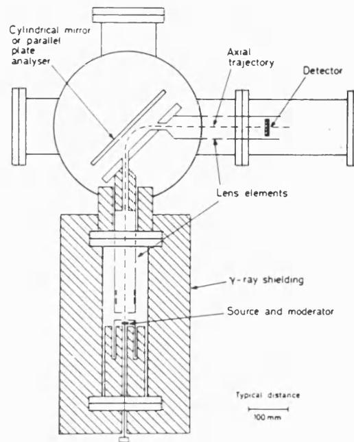
Figure 2.1 A typical electrostatically guided positron beam.
