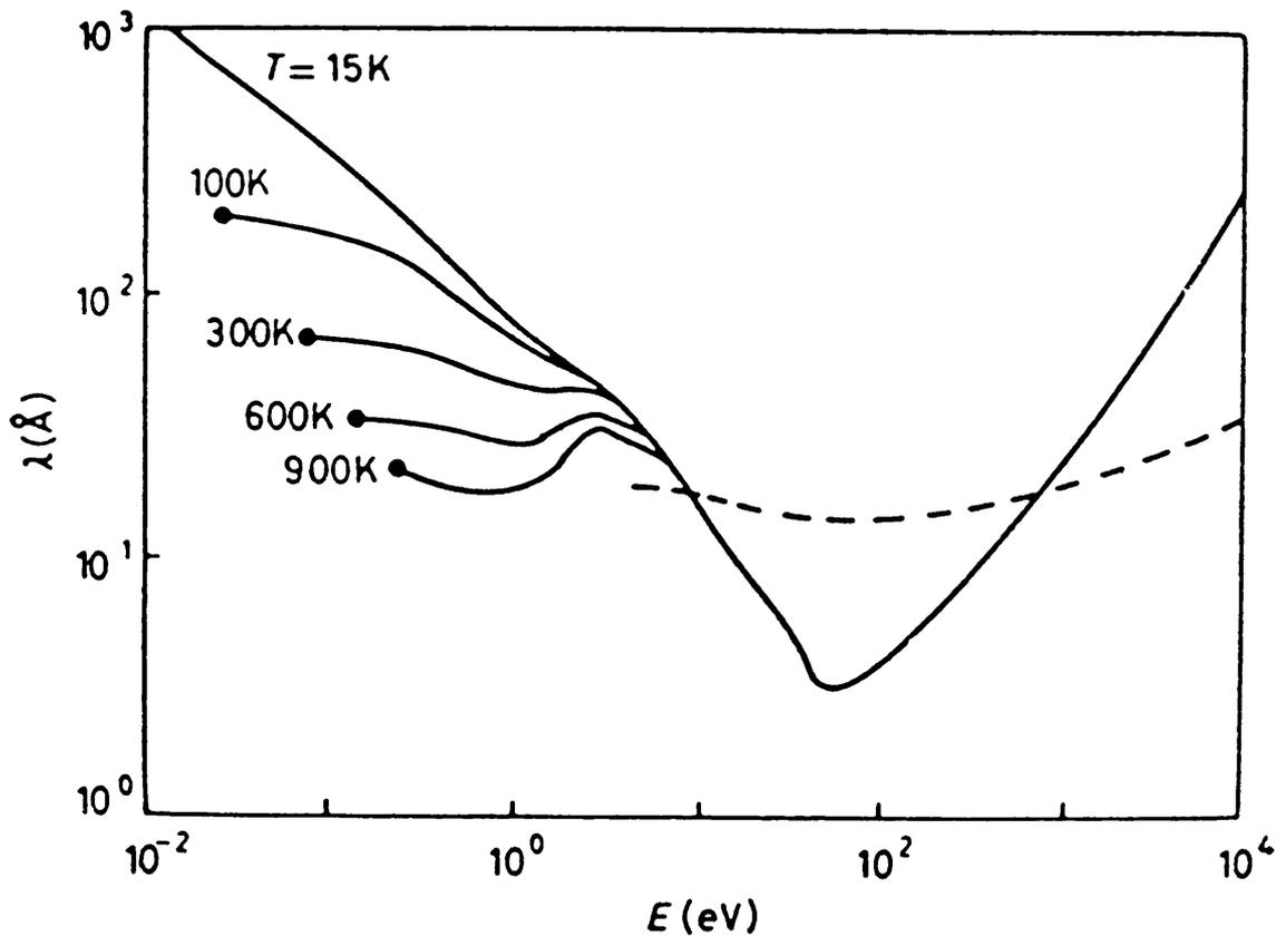
**Figure 3.10** The positron mean free path in aluminium as a function of positron energy (Nieminen and Oliva (1980)).
