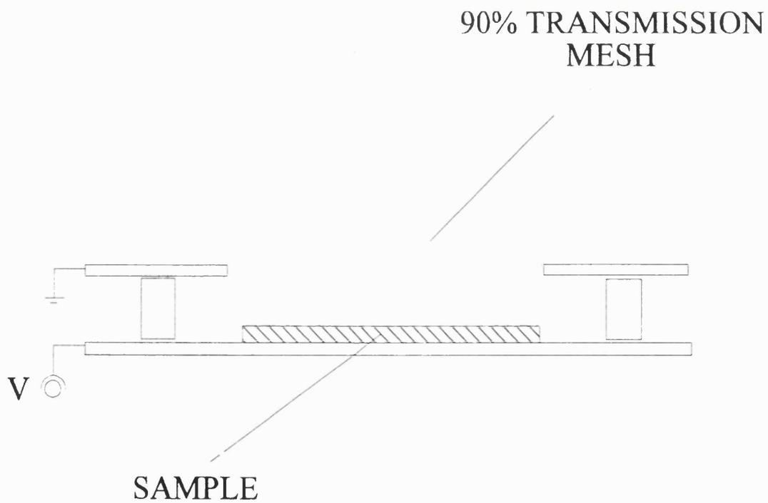
Figure 3.22 A schematic diagram of the target holder.
