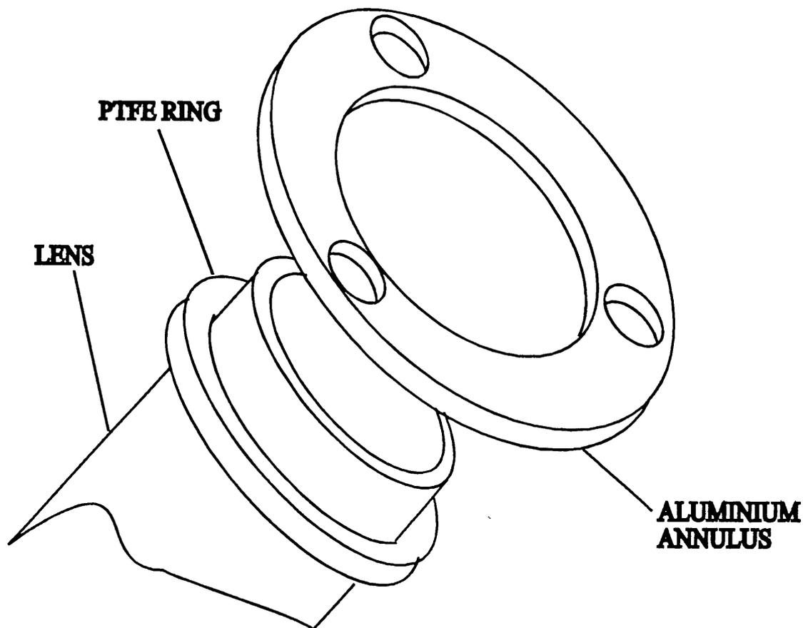
Figure 2.10 A schematic diagram of the lens mount, with tripod omitted for clarity.
