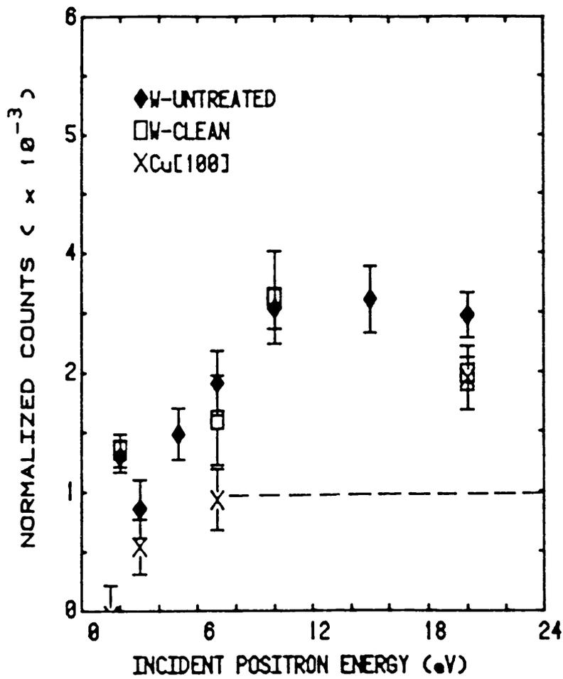
Figure 3.13 The  $\text{Ps}^*$  yield from a W target before and after cleaning, and from an untreated Cu(100) target (Schoepf et al (1982)).
