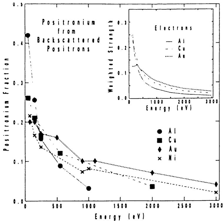
Figure 3.12 The backscattered positronium yield from a number of materials as a function of incident positron energy. Also inset, backscattered electron yields from the same materials after correcting for the  $1/E$  positronium formation cross-section (Howell *et al* (1986)).
