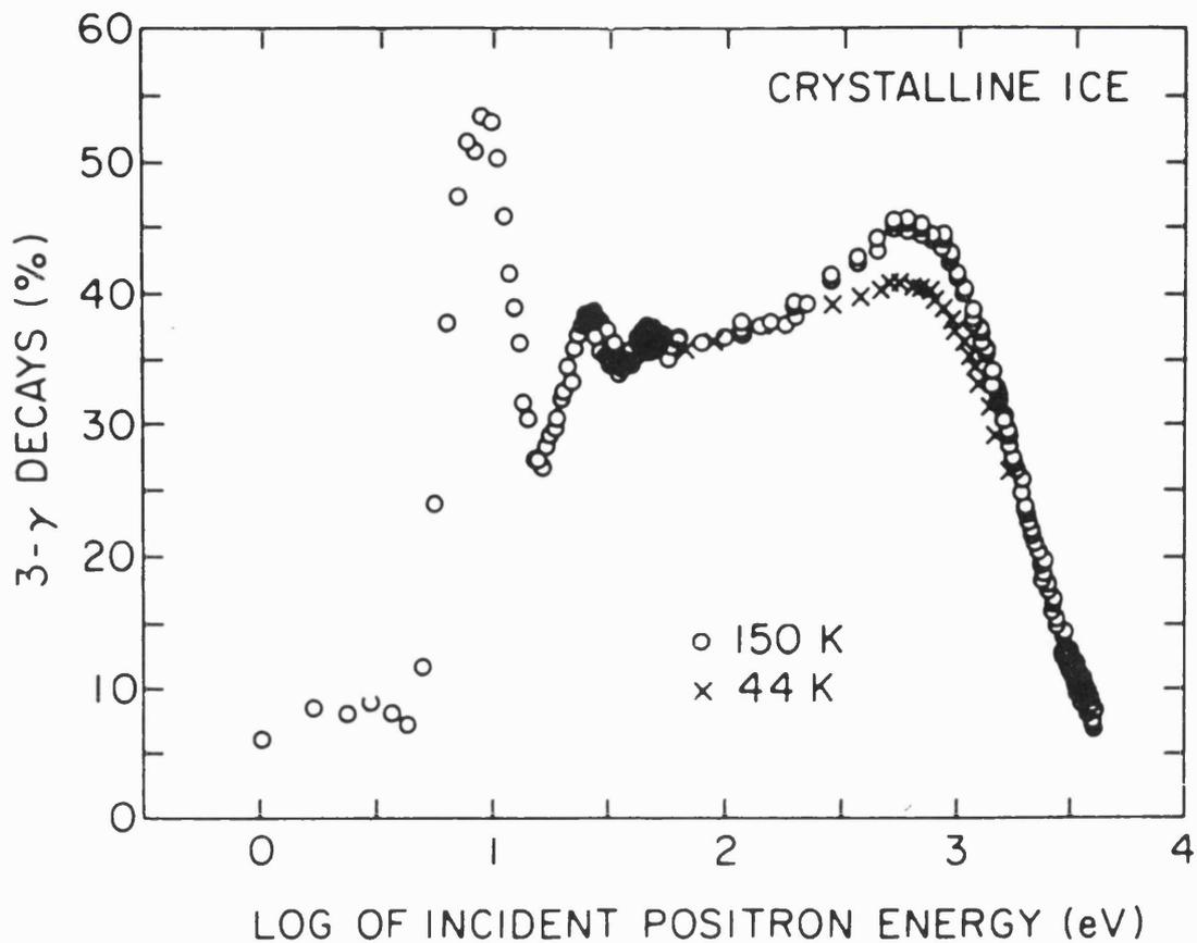
Figure 3.4 The positronium yield from positrons implanted into ice as a function of positron energy (Eldrup *et al* (1983)).
