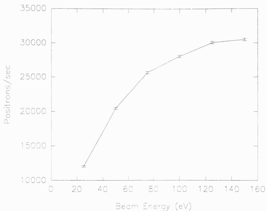
**Figure 2.16** The relative intensity of the electrostatic positron beam as a function of transport energy.
