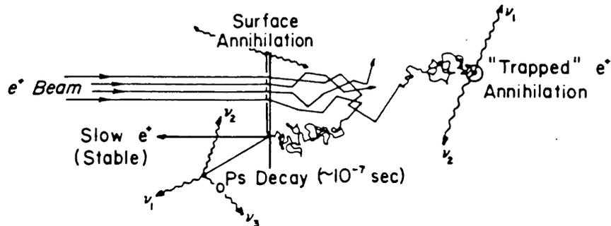
Figure 1.7 The interaction of a positron beam of energy  $< 100\text{keV}$  with the near surface region of a solid (Schultz & Lynn (1988)).
