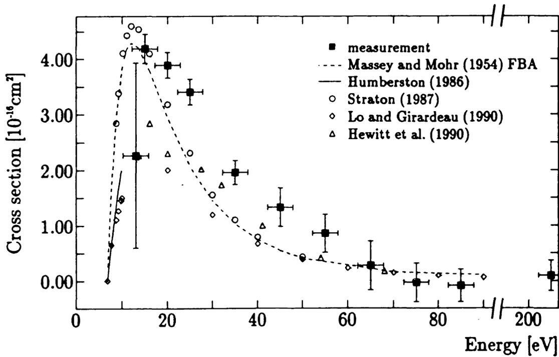
Figure 3.5 The Ps formation by positron impact with atomic hydrogen measurements of Sperber *et al* (1992), along with the theoretical treatments of Massey and Mohr (1959), Humberston (1986), Straton (1987), Lo and Girardeau (1990) and Hewitt *et al* (1990).
