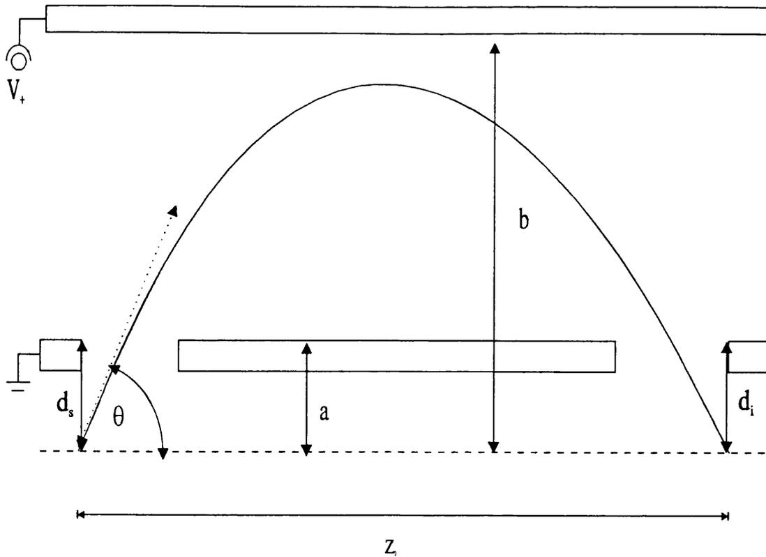
**Figure 2.6** The parameters of interest when designing a CMA.
