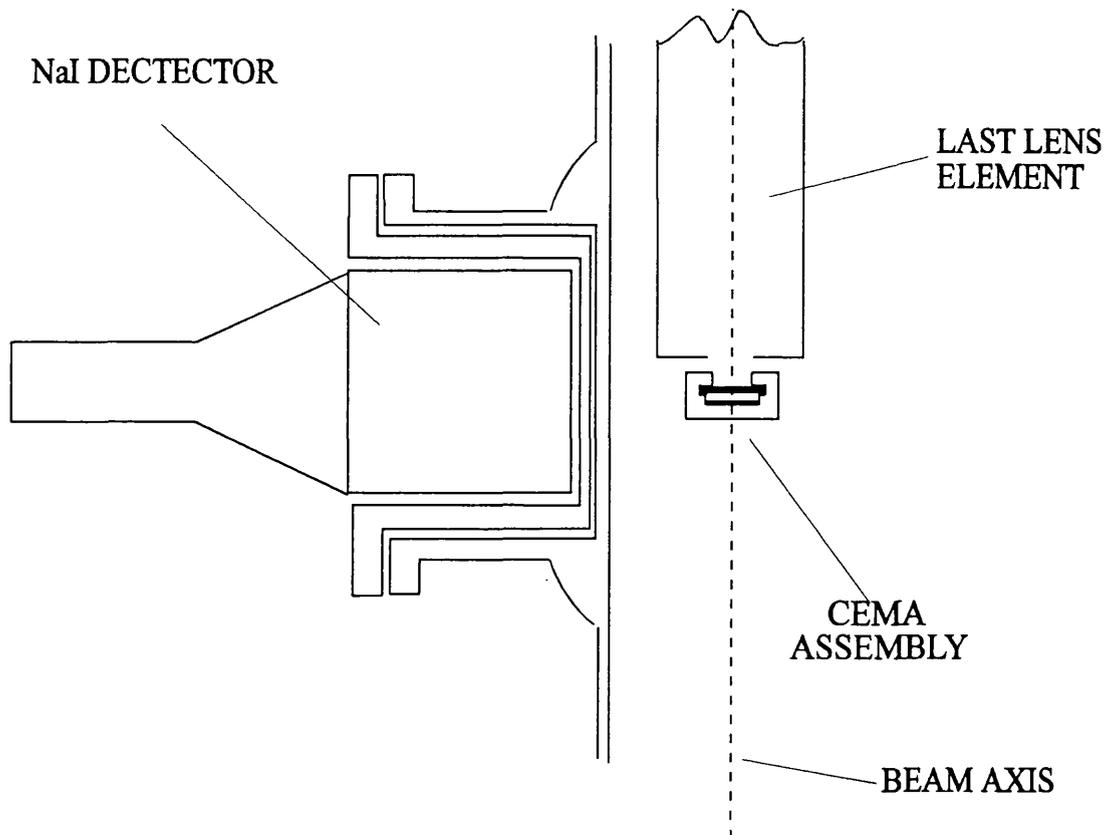
**Figure 2.14** A schematic diagram of the detector arrangement used to determine the CEMA detection efficiency.
