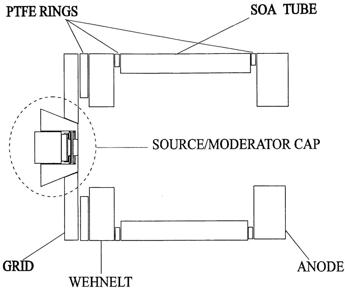
Figure 2.3 A schematic diagram of the modified Soa gun.
