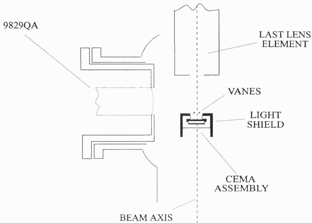
Figure 4.12 A schematic diagram of the interaction region used in the radiative lifetime experiments.
