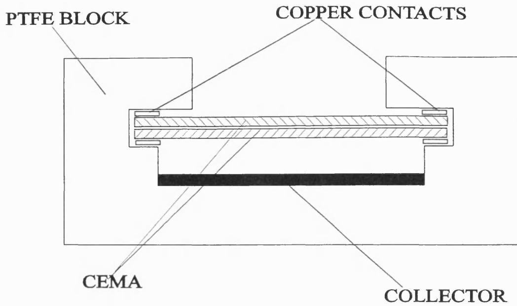
Figure 2.12 A schematic diagram of the CEMA holder.
