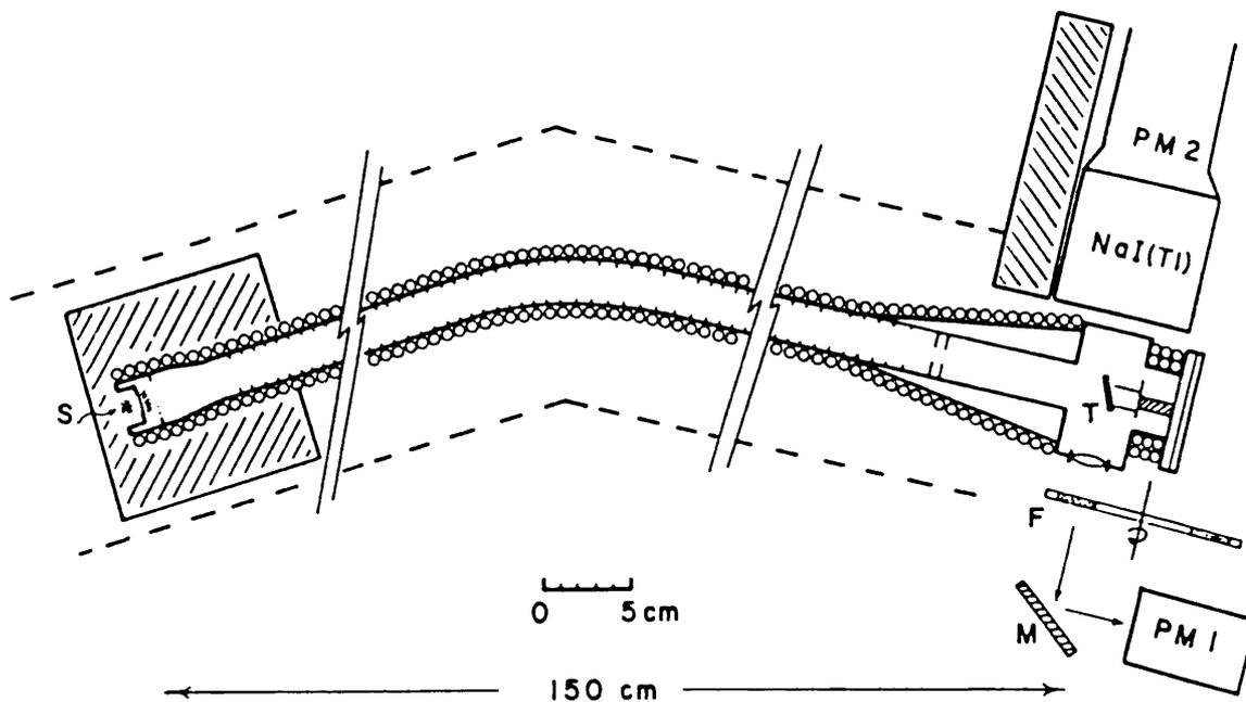
Figure 3.1 A schematic diagram of the experimental arrangement of Canter *et al* (1975).
