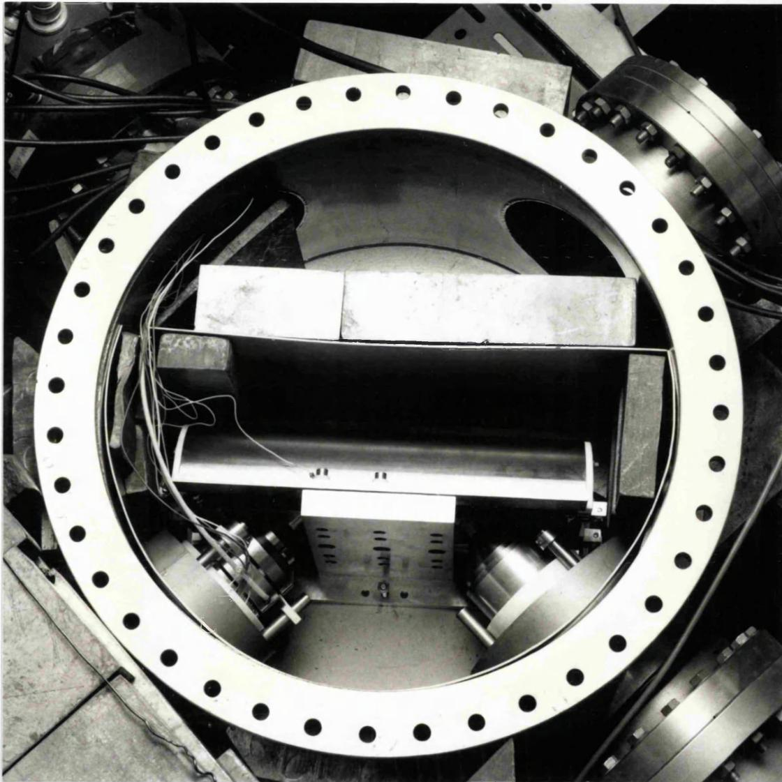
**Figure 2.7** A photograph of the CMA, with the input and output lens stacks clearly in view.
