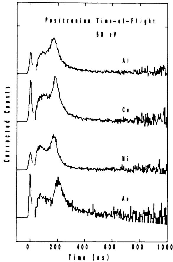
Figure 3.11 Positron time of flight spectra for a number of materials subject to positron bombardment at 50eV (Howell *et al* (1986)).
