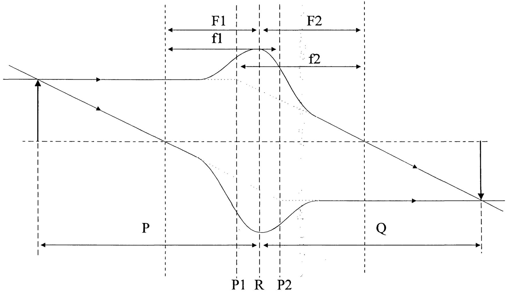
Figure 2.2 The design parameters of a simple electrostatic lens.
