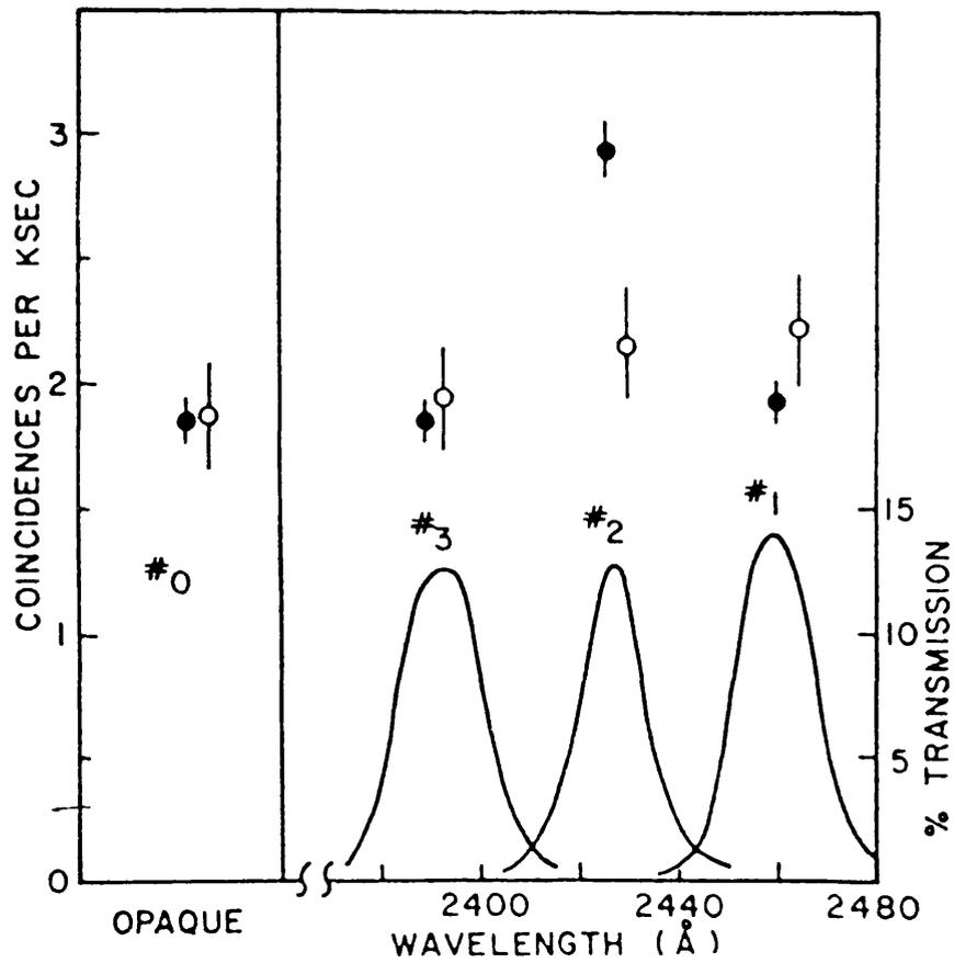
Figure 3.2 The total Lyman- $\alpha$ / $\gamma$ -ray coincidence rate for filters centred on 200nm, 240nm, and 280nm (Canter *et al* (1975)).
