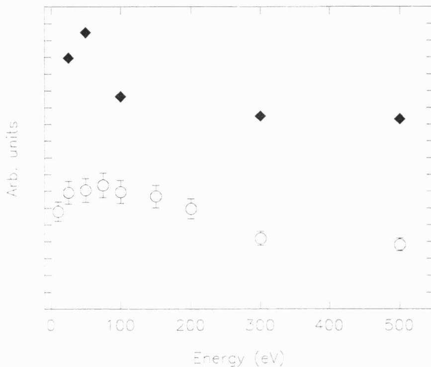
**Figure 3.35** The relative yield of positrons re-emitted from a Au target with energies  $\leq 15\text{eV}$ , as a function of incident positron energy ( $\blacklozenge$ ). The relative  $\text{Ps}^*$  yield as a function of energy, for positrons incident on a Cu target ( $\circ$ ).
