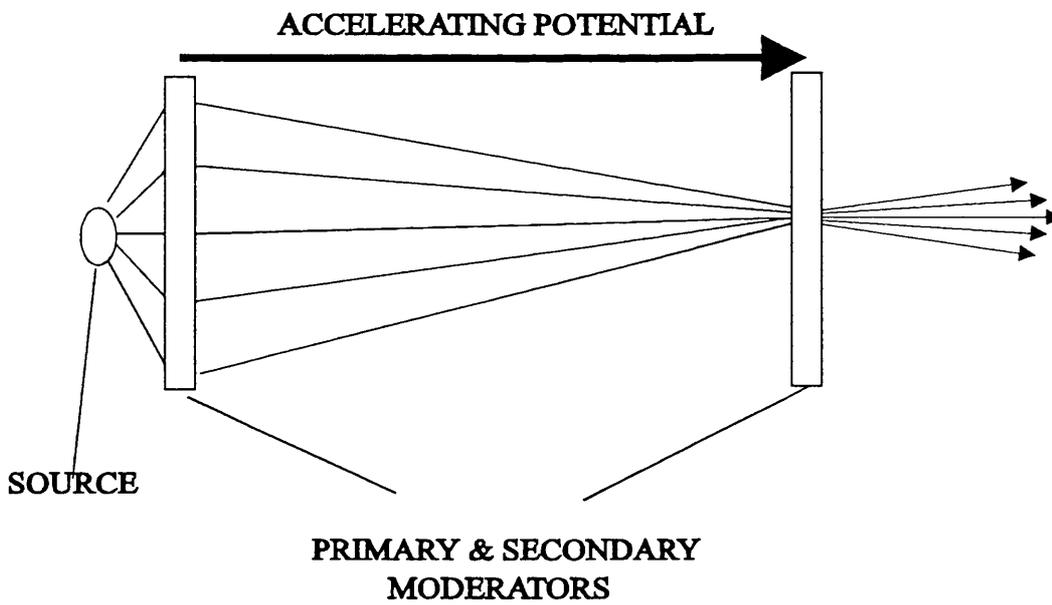
Figure 1.13 A schematic diagram depicting the process of brightness enhancement.
