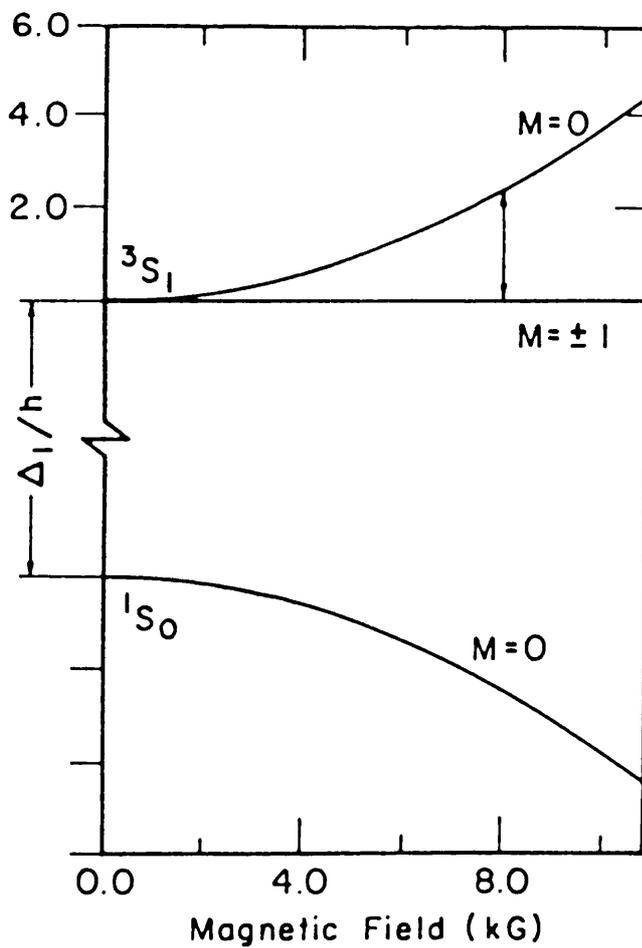
Figure 4.2 The splitting of the  $m=0$  ground state energy levels of positronium, as a function of applied magnetic field
