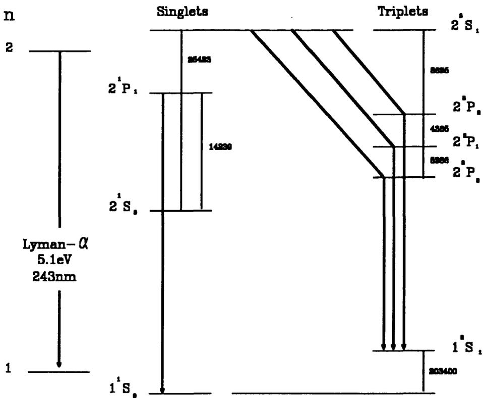
Figure 4.1 The  $n=1$  and  $n=2$  energy levels of hydrogen (top) and positronium (bottom). All intervals in MHz.
