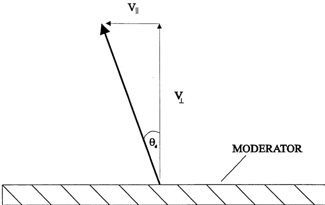
Figure 1.12 A schematic diagram showing the velocity components of a re-emitted thermalised positron, after leaving the moderator surface.
