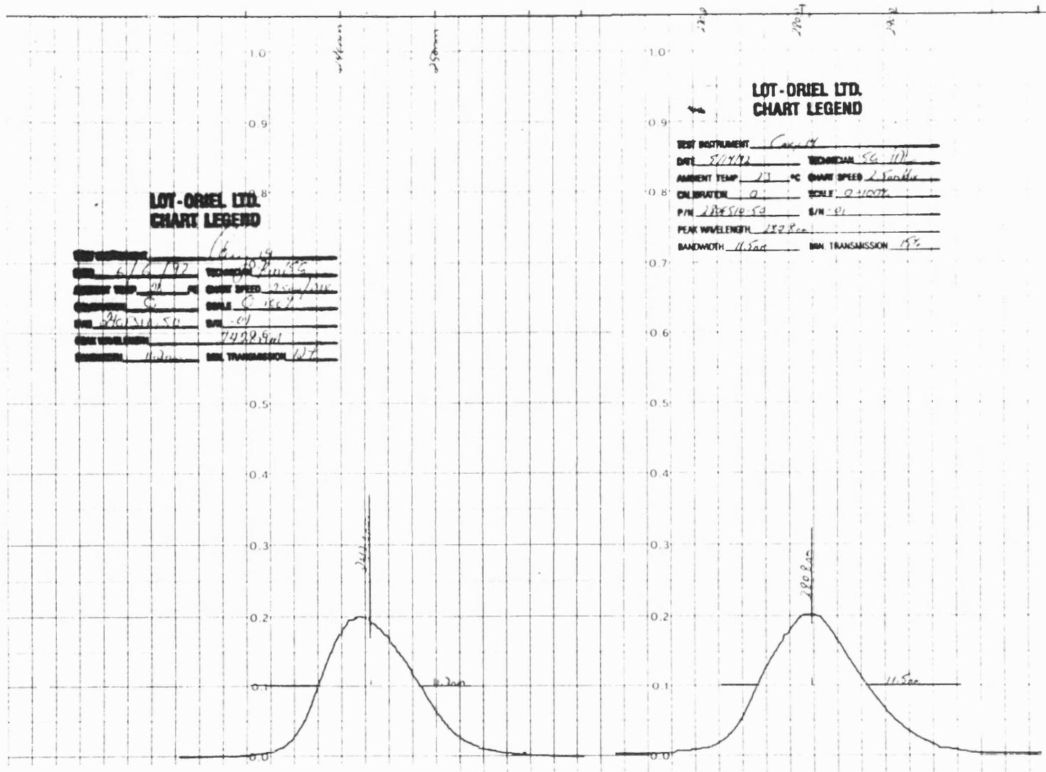
Figure 3.26 The measured optical properties of the 240nm filter (left) and the 280nm filter (right).
