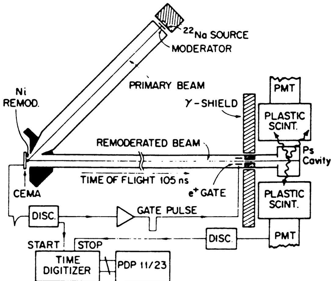
Figure 4.3 A schematic diagram of the apparatus used by Nico *et al* (1992) to measure the positronium  $1^3S_1$  vacuum decay rate.
