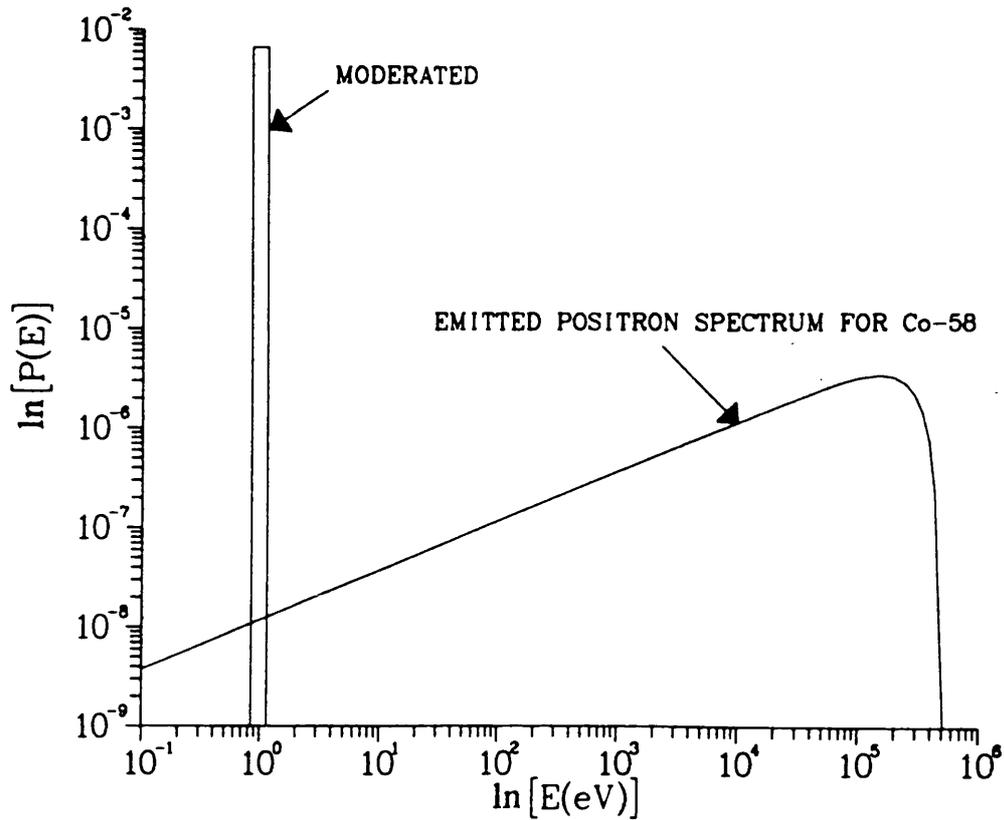
Figure 1.4 A comparison of the calculated slow positron yield from a W(110) moderator with the primary  $\beta^-$ 's in the same energy range directly emitted by a  $^{58}\text{Co}$  source (Schultz and Lynn (1988)).
