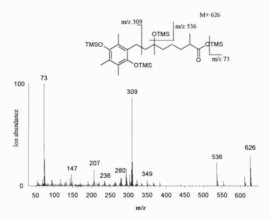
Figure 4.11. Spectrum of oxidised  $\alpha$ -CMBHC (retention time = 28.7 mins) showing possible fragmentations.
