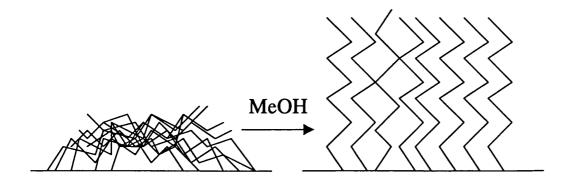
Figure 2.1. A The structure of silanol based SPE cartridges. Changes in the R group affect retention and elution characteristics. B Priming the cartridges with an organic solvent such as methanol stops aggregation of the hydrophobic sidechains and thereby increases retention of molecules with hydrophobic areas.
