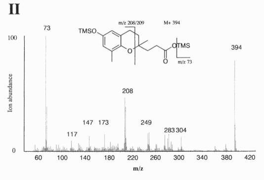
Figure 2.13. Mass spectra of  $\gamma$ -CEHC-TMS (I) and  $\delta$ -CEHC-TMS (II).
