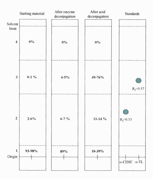
**Figure 4.12.** Thin layer chromatograms of radiolabelled rat urine extracts, showing percentage of total radiolabel in each section (1-4) of the chromatogram (n = 2).
