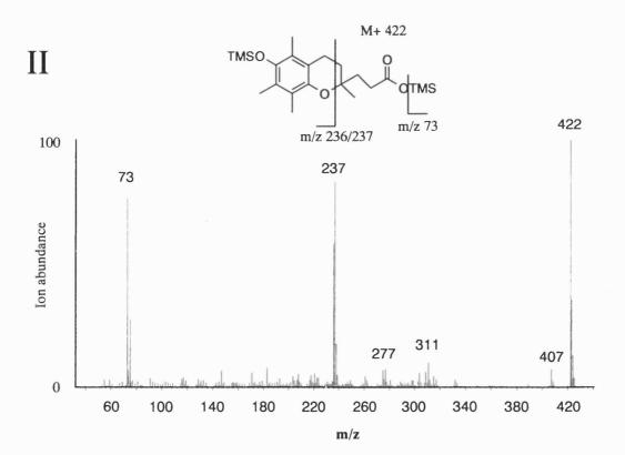
Figure 2.11. Mass spectra of  $\alpha$ -tocopheronolactone-TMS (I) and  $\alpha$ -CEHC-TMS (II) with fragment and molecular ions shown.
