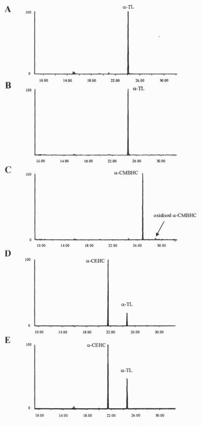
Figure 5.1. GC-MS of synthetic conjugated standards after enzymatic deconjugation. A  $\alpha$ -tocopheronolactone-glucuronide, B  $\alpha$ -tocopheronolactone-sulphate, C  $\alpha$ -CMBHC-sulphate, D  $\alpha$ -CEHC-glucuronide and E  $\alpha$ -CEHC-sulphate.
