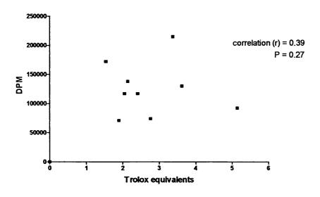
Table 4.4. Recovery of radioactivity in the final derivatised fraction and the correlation between radioactivity in this fraction and the amount of  $\alpha$ -tocopherol metabolites as measured by GC-MS.
