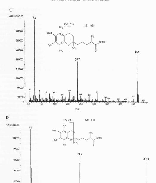
**FIG. 4.** Spectra of  $d_0$  TMS- $\alpha$ -CMBHC (compound C) and  $d_6$  TMS- $\alpha$ -CMBHC (compound D).
