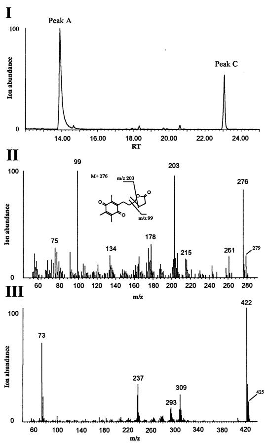
Figure 2.6. Total ion chromatogram of  $d_3$ - $\alpha$ -tocopheronolactone standard (I) with spectra of peak A (II) and peak C (III).
