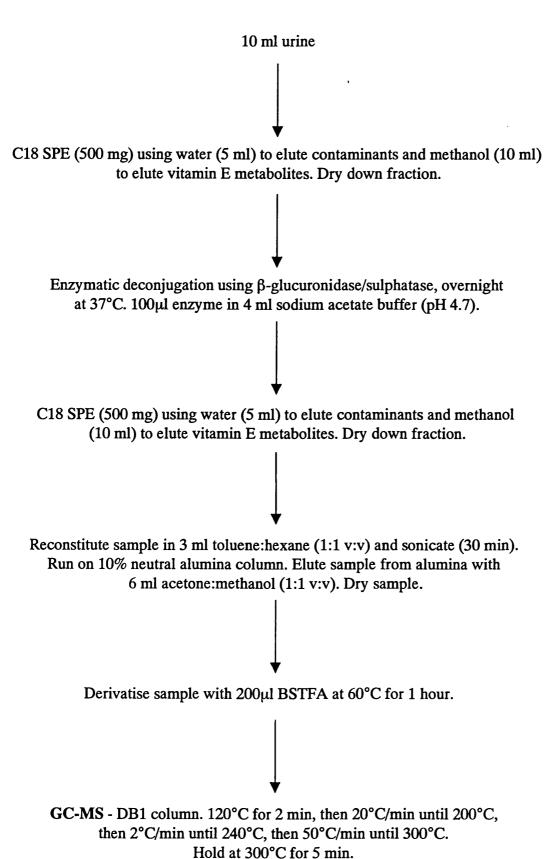
Figure 2.4. Method used as starting point for method development.
