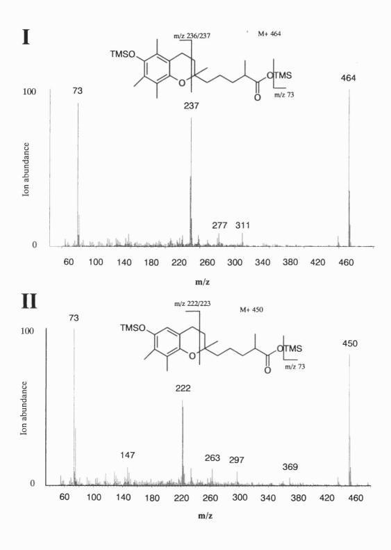
Figure 2.12. Mass spectra of  $\alpha$ -CMBHC-TMS (I) and  $\gamma$ -CMBHC-TMS (II).
