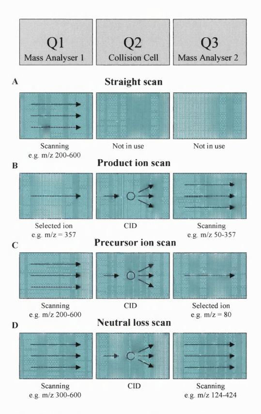
**Figure 6.3.** Examples of possible analysis using a triple quadrupole mass spectrometer. See text for details. CID = Collision induced dissociation
