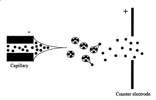
Figure 6.2. (A) Features of an ESI source and (B) schematic of the ionisation process in negative ion mode.
