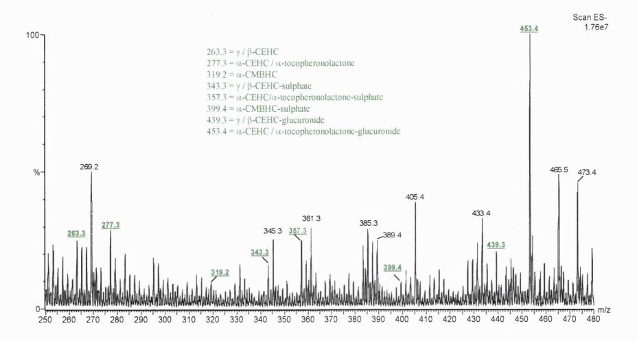
**Figure 6.4.** Negative ion ESI-MS of a urine sample after oral supplementation with  $\alpha$ -tocopheryl acetate (1000 mg/d for 3 wk) Peaks corresponding to masses of vitamin E metabolites are underlined and in green.
