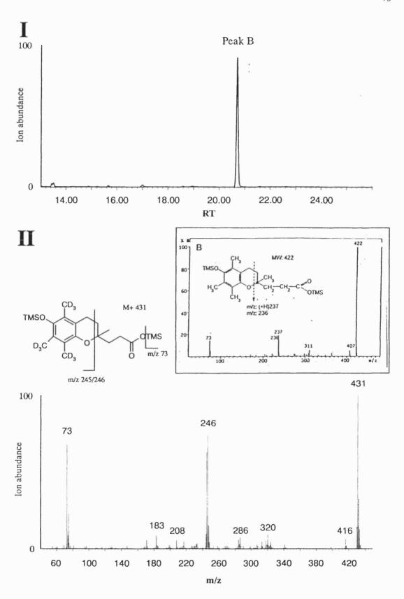
Figure 2.5. Chromatogram of  $d_9$ - $\alpha$ -CEHC standard (I) and the corresponding mass spectrum (II). The inset shows the spectrum of  $d_0$ - $\alpha$ -CEHC reported by Schultz et al. (1995). The major fragment ion is produced by cleavage of the chroman ring.
