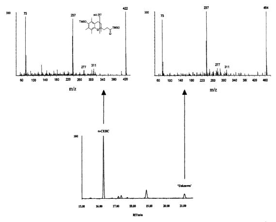
Figure 2. Gas chromatogram showing elution of the silyl derivatives of  $\alpha$ -CEHC and the 'unknown' metabolite with their corresponding mass spectra.
