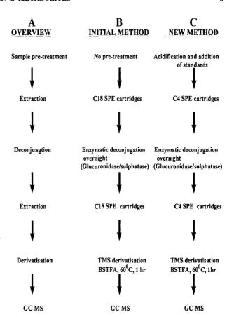
**FIG. 1.** A flowchart displaying the principal steps involved in the analysis of urinary vitamin E metabolites. SPE, solid phase extraction; TMS, trimethylsilyl; BSTFA, N,O-bis(trimethylsilyl)trifluoroacetamide; GC-MS, gas chromatography-mass spectrometry.
