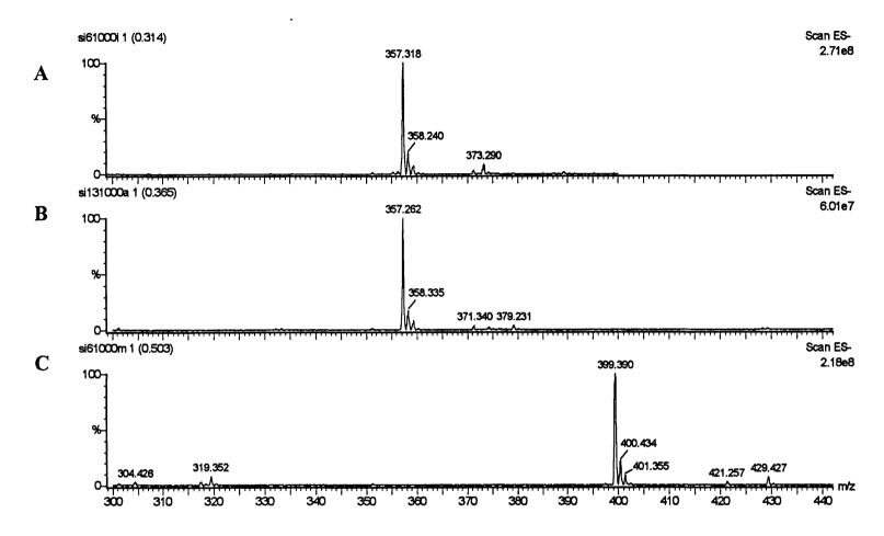
Figure 6.8. Negative ion ESI-MS of A  $\alpha$ -tocopheronolactone-sulphate, B  $\alpha$ -CEHC-sulphate and C  $\alpha$ -CMBHC-sulphate standards
