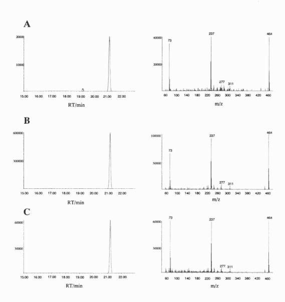
Figure 3.7. A and B show extracted ion chromatograms (m/z 464) and corresponding mass spectra of silyl derivatives of the urinary metabolite and  $\alpha$ -CMBHC standard, respectively. C shows the equivalent data for a mixture of  $\alpha$ -CMBHC standard and the urinary metabolite, showing co-elution of the two peaks and an identical mass spectrum.
