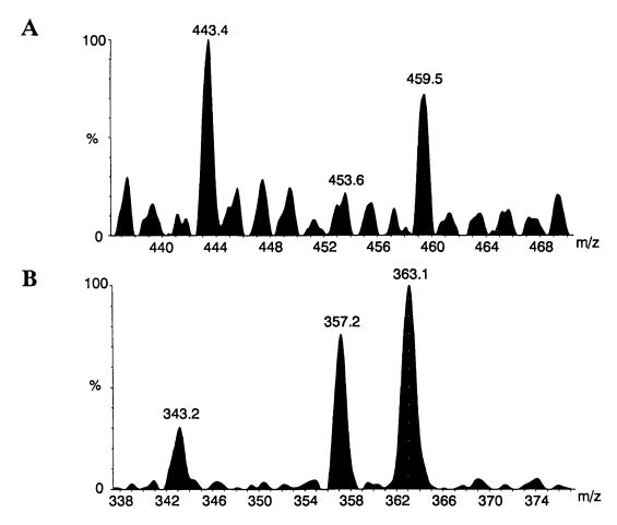
Figure 6.6. Negative ion ESI-MS/MS neutral loss and precursor ion spectra after oral  $d_6$ - $\alpha$ -tocopheryl acetate supplementation. A neutral loss of 176 (glucuronides) and B precursors of m/z 80 (sulphates). Additional peaks were present when compared to normal urine (figure 6.5). These peaks were greater in mass/charge ratio by 6 Da/e, confirming they were  $d_6$ -analogues of the natural  $\alpha$ -tocopherol metabolites.
