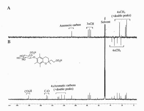
Figure A1.2. DEPT (distortionless enhancement by polarisation transfer)  $^{13}$ C NMR of  $\alpha$ -CEHC-glucuronide.
