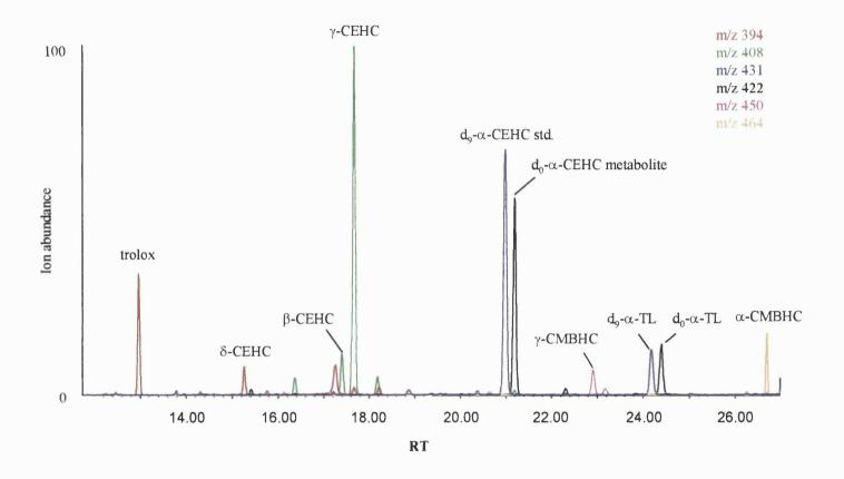
Figure 2.10. An extracted ion chromatogram showing the main urinary vitamin E metabolites.
