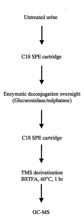
Figure 2.9. The initial procedure that was used in order to optimise the method.
