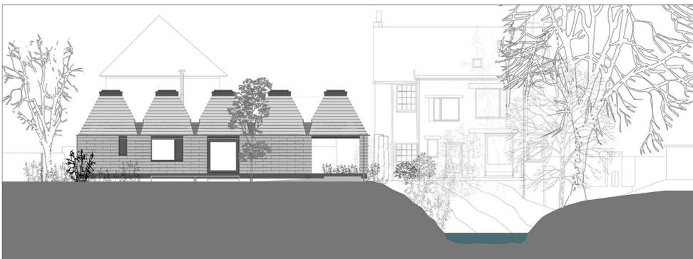
central bays provide living accommodation opening onto the garden. Skylights cast daylight into the spaces below and also open in summer to provide cooling stack ventilation. Interior fittings extend the material palette with oak, pine triply, untreated brass, and wool.
