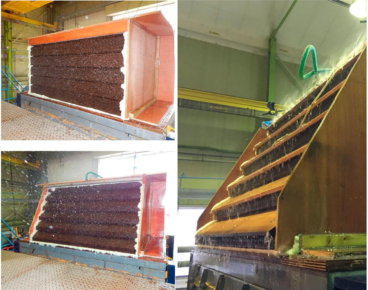
block faces to shed rainwater, and prevent it from gradually saturating cork blocks from above during periods of prolonged heavy rain. The weatherboarding is screw-fixed into insulation plugs in the cork to retain a relative ease of disassembly. A panel fabricated to the revised design was tested to the same rain penetration standard by BRE (Fig. 7). This time, the result was no water leakage, including at a high-pressure factor of over 175 Pa.
