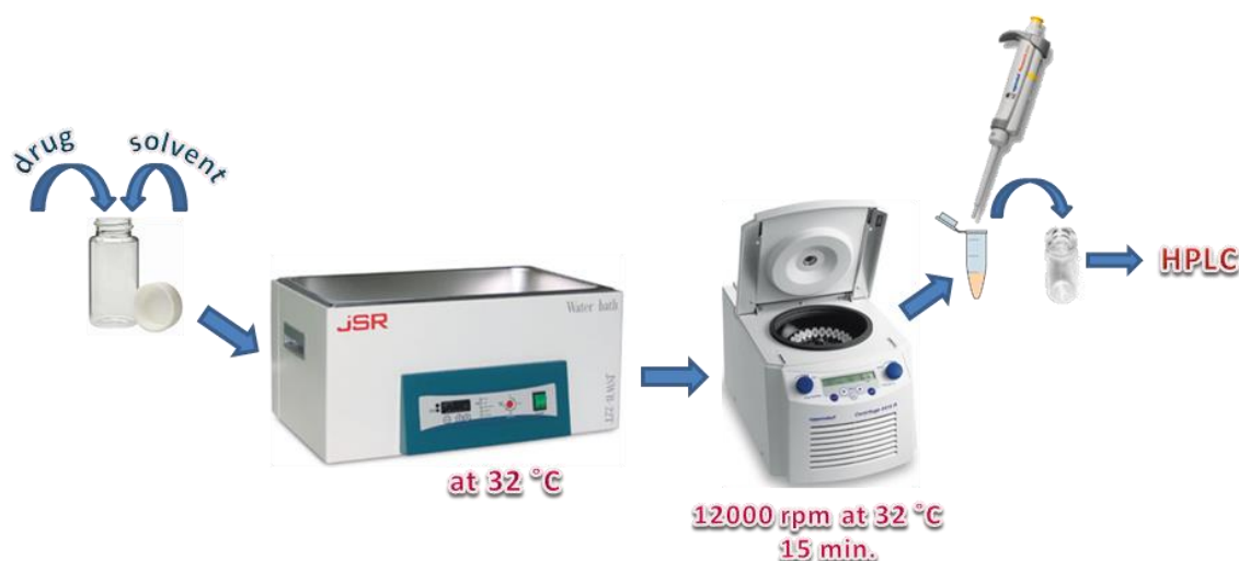
Figure 3-2 Determining the solubility of drug using the water bath method
