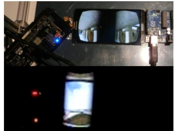
*Figure 2 - Disassembled HMD (upper) and a quick exposure close-up (lower) of the display showing a band of illuminated pixels during scanout.*
