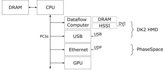
Figure 7 – VR System architecture. The dataflow computer takes the place of the GPU for the headset.
