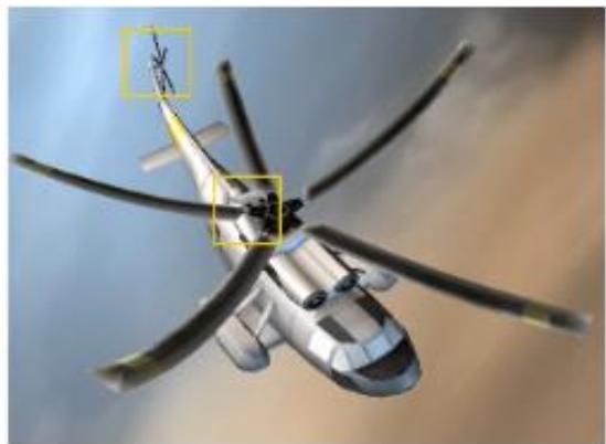
*Figure 12 - Non-linearly rasterised image. Traditionally such images would be produced by warping a linear rasterization. This would introduce artefacts in highly detailed areas such as the highlighted insets above, but the fragment-shader ray-traced image is pixel perfect.*
