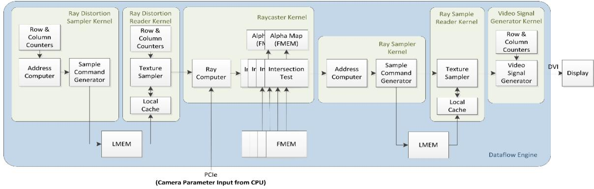
Figure 6 - Architecture of Low Latency Ray-caster
