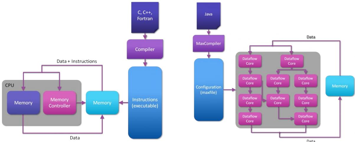
Figure 3 - Comparison of Control Flow (left) vs. Dataflow (right) Computing
