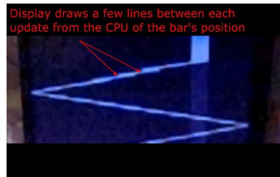
Figure 4 - Frameless image generator showing a white bar moving back and forth across a desktop display.
