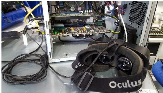
Figure 8 - Dataflow PCIe co-processor card connected to a DK2
