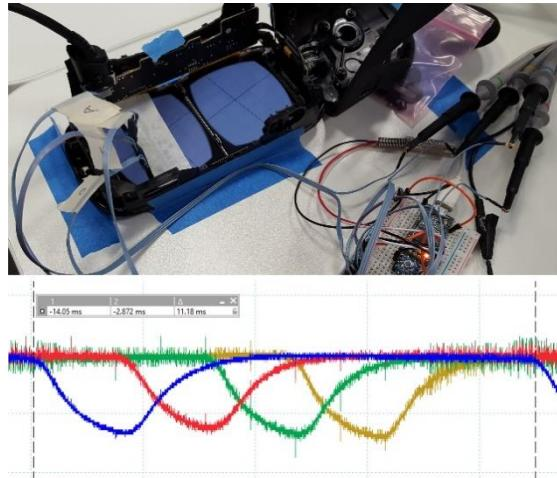
*Figure 1 – Profile of an Oculus CV1 display captured by placing four photodiodes across the screen. The horizontal axis is the distance across the display and the vertical axis is the luminance of the area under the diode.*
