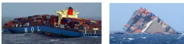
(a) MOL Comfort accident with hull girder collapse followed by sinking, occurred in June 2013
