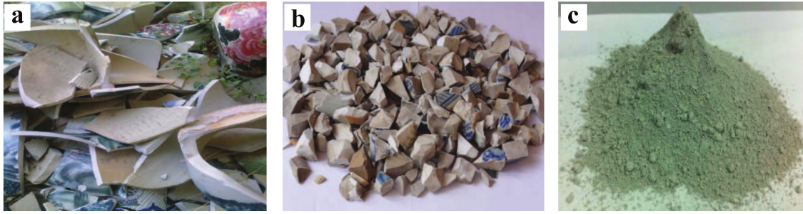
Figure 1: Ground ceramic preparation process: (a) raw ceramic products as received; (b) coarse ceramic particles ground by jaw crusher; (c) micro ceramic particles powdered by air jet mill.
