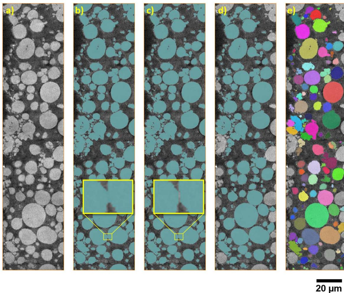
**Figure 9.** For the merged nano-CT dataset of an NMC electrode, (a) original virtual slice, (b) segmented virtual slice, (c) neighbouring particles separated, (d) border particles removed and (e) individually labelled particles.
