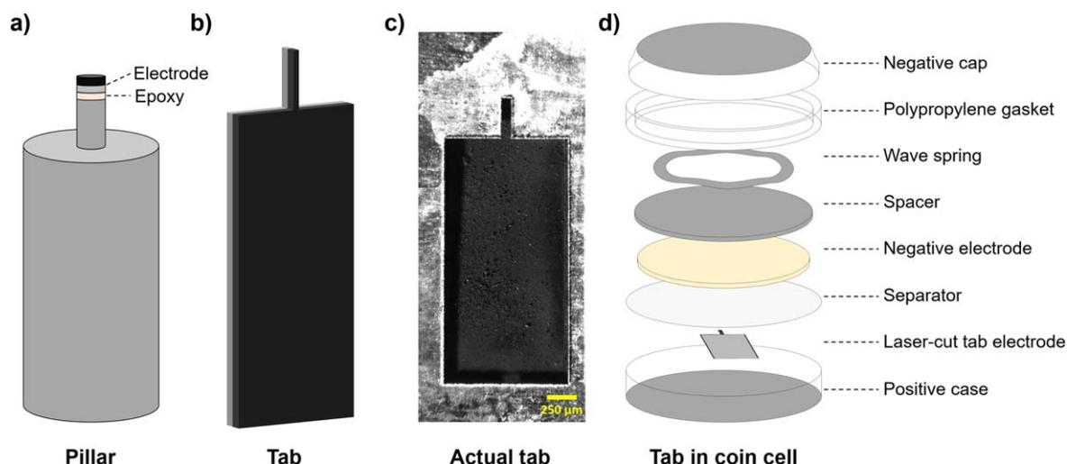
**Figure 4.** Potential sample geometries that can be achieved with laser-milling, including (a) conventional pillar-shaped electrode mounted on a dowel pin, (b) tab-shaped electrode and (c) the same tab-shaped geometry cut from an actual electrode. (d) A schematic of the tab electrode in a coin cell.
