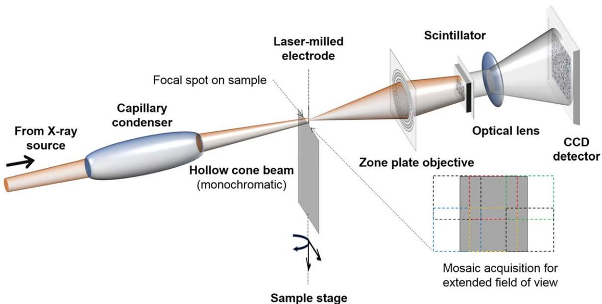
Figure 1. Transmission X-ray microscopy architecture showing Fresnel zone plate objective.
