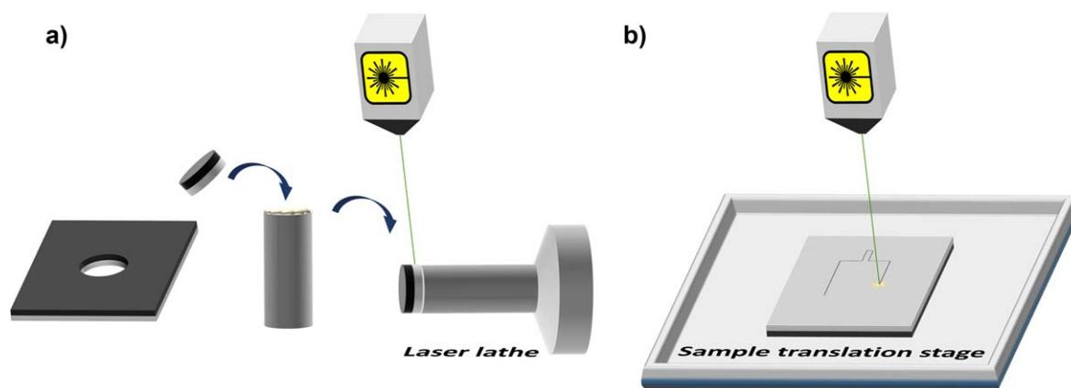
**Figure 3.** (a) Conventional electrode pillar preparation technique and (b) New electrode tab preparation technique.
