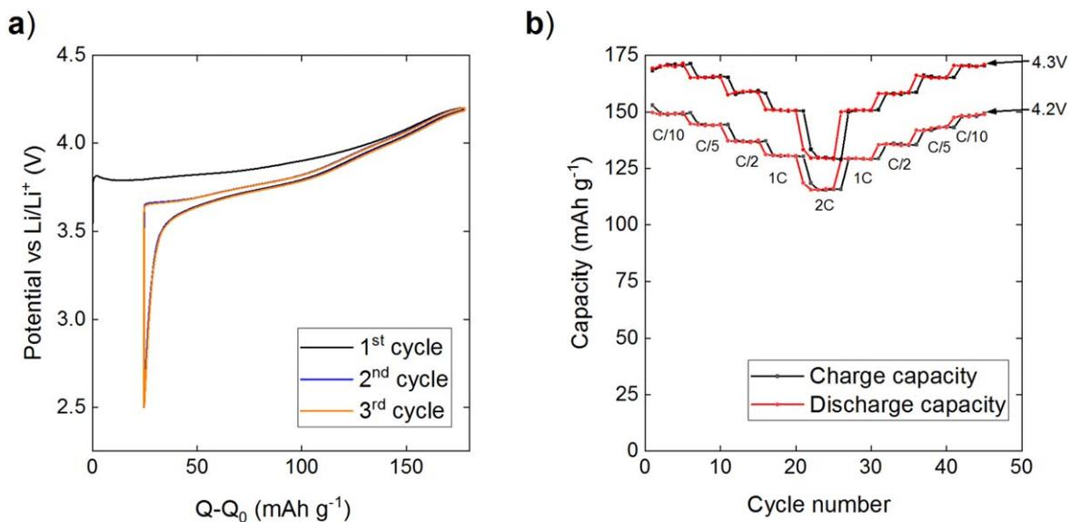
**Figure 6.** For the tab electrode assembled in a coin cell with Li metal as the negative electrode, (a) first 3 cycles conducted at C/20 and (b) rate capability test at various C-rates. All current values were calculated from an areal capacity of ca. 2 mAh cm<sup>-2</sup> and a mass loading of ca. 10.52 mg cm<sup>-2</sup>.
