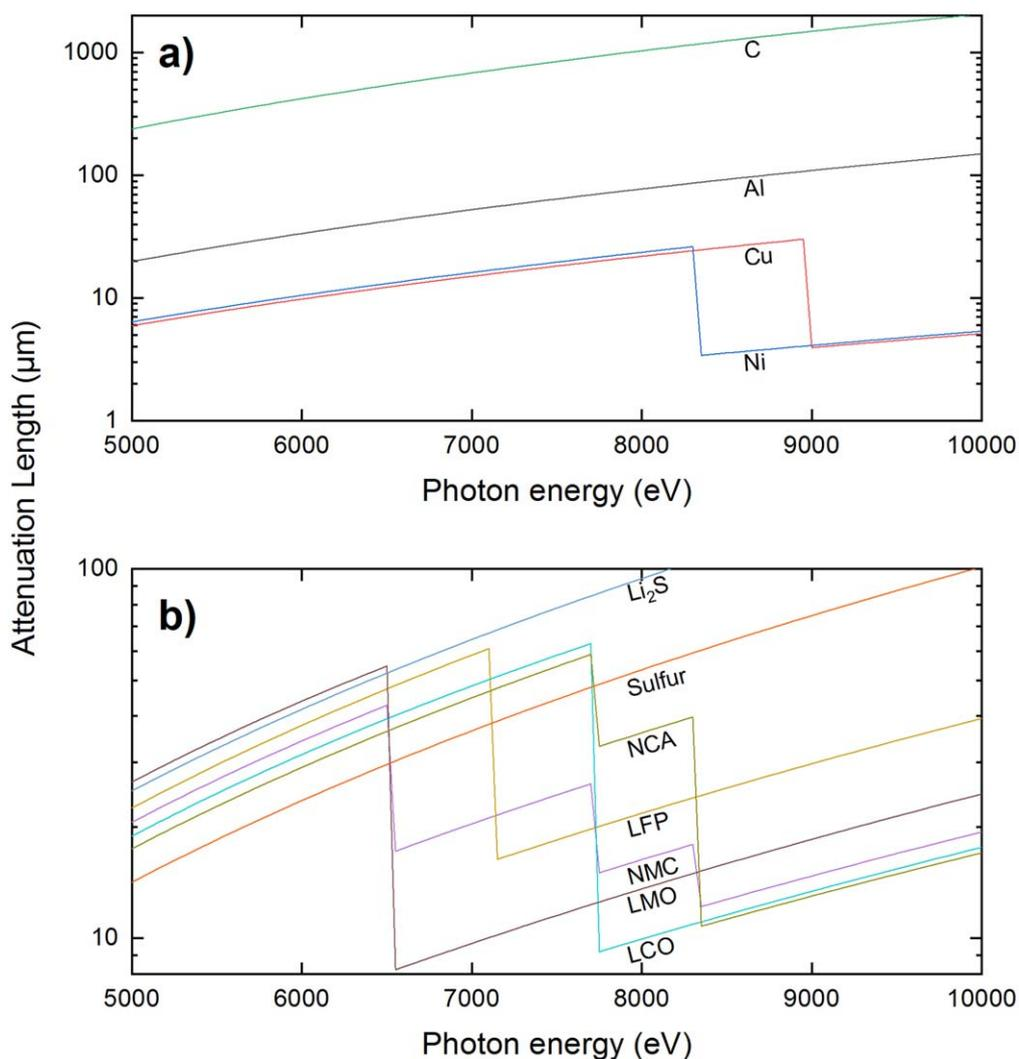
Figure 2. Attenuation lengths where the ratio between the incident beam and the transmitted beam, or transmission, falls to  $1/e$  (ca. 36.8%) for (a) common current collector materials and graphitic carbon and (b) common positive electrode materials in Li-ion and Li-S batteries.<sup>14</sup>
