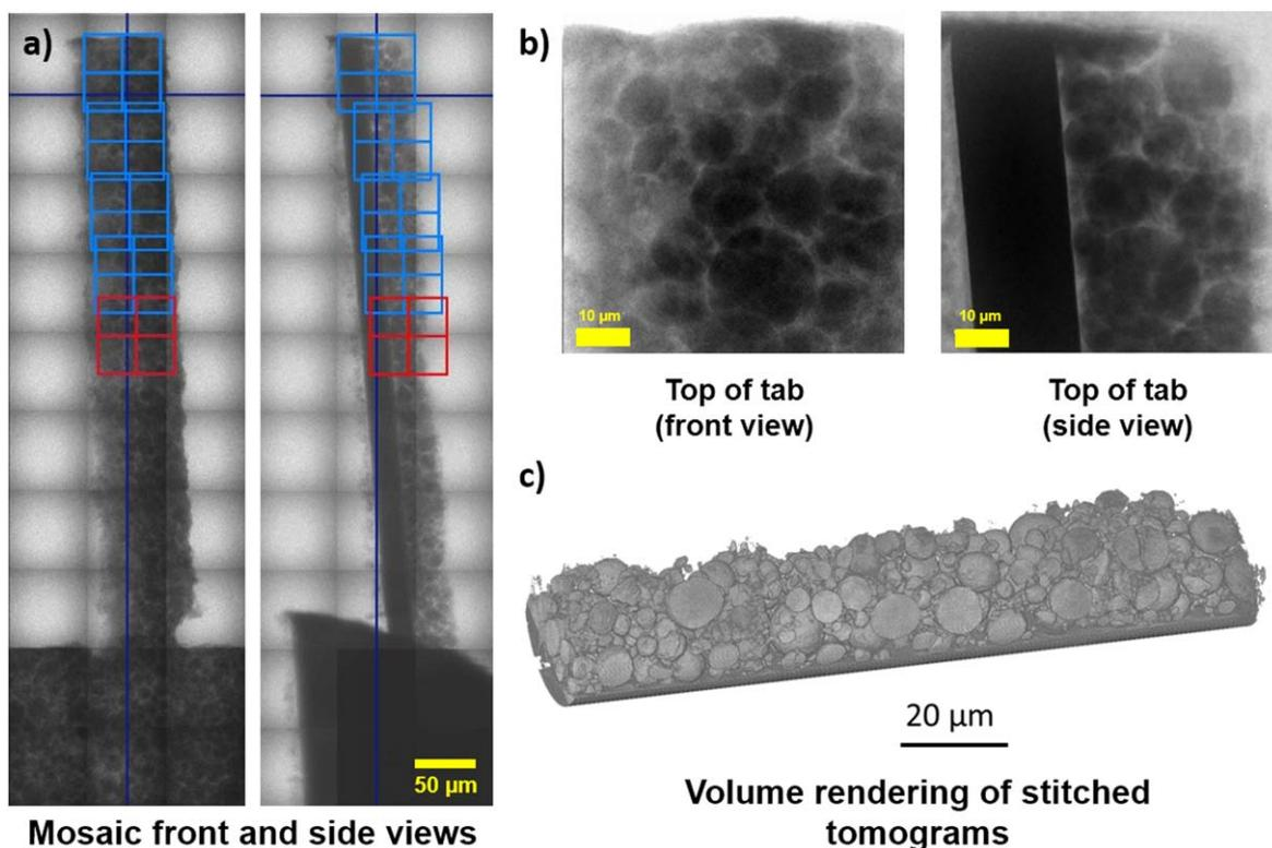
**Figure 5.** (a) Mosaic front and side radiographs of the NMC electrode tab where the field of view of each blue or red is ca.  $65 \mu\text{m}$ . (b) A front and side radiographs at the top of the NMC tab and (c) a volume rendering of the stitched tomograms acquired from the electrode.
