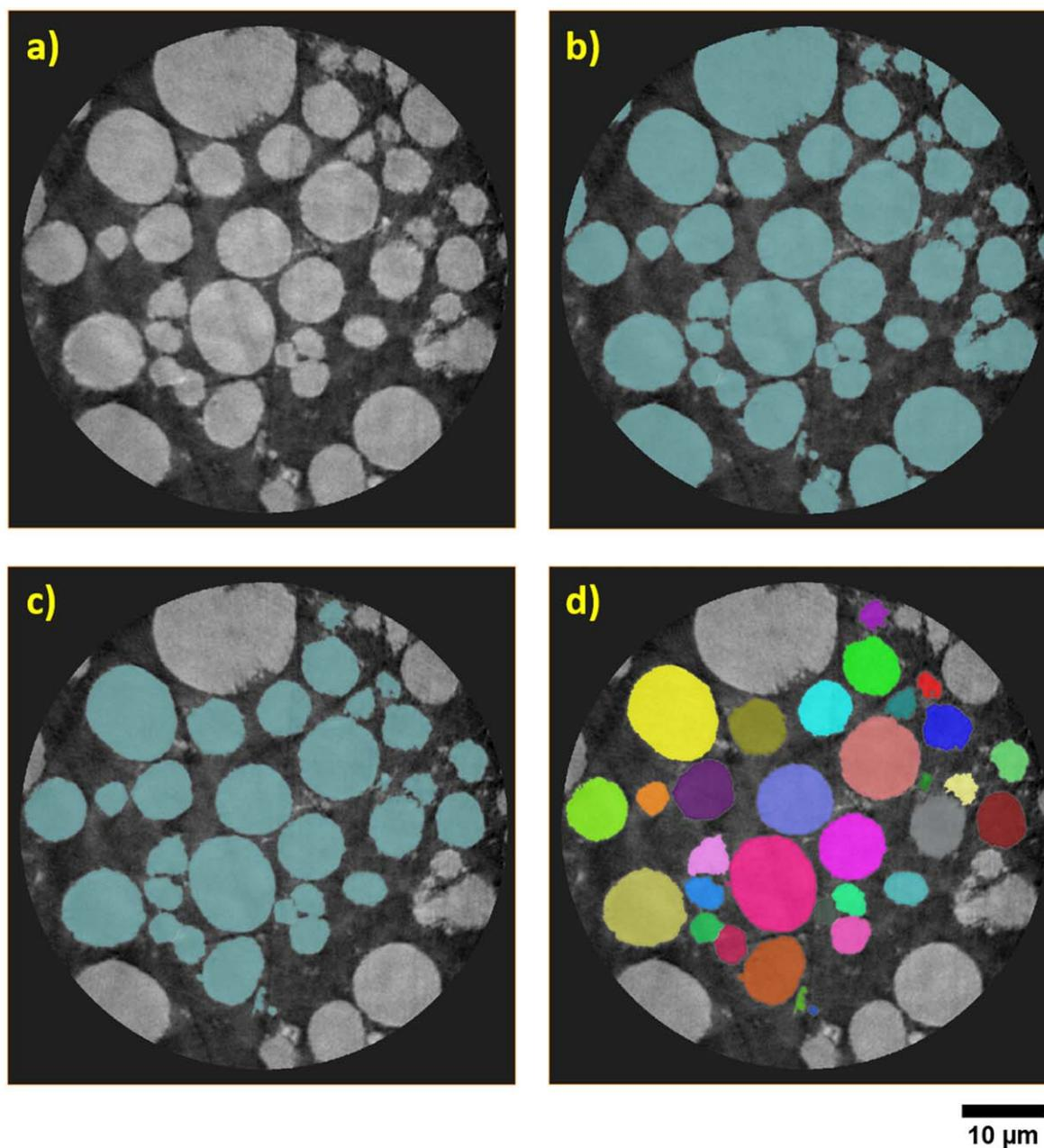
**Figure 8.** For the laser-milled pillar of the NMC electrode, (a) original virtual slice, (b) segmented virtual slice and neighbouring particles separated, (c) border particles removed, and (d) individually labelled particles.
