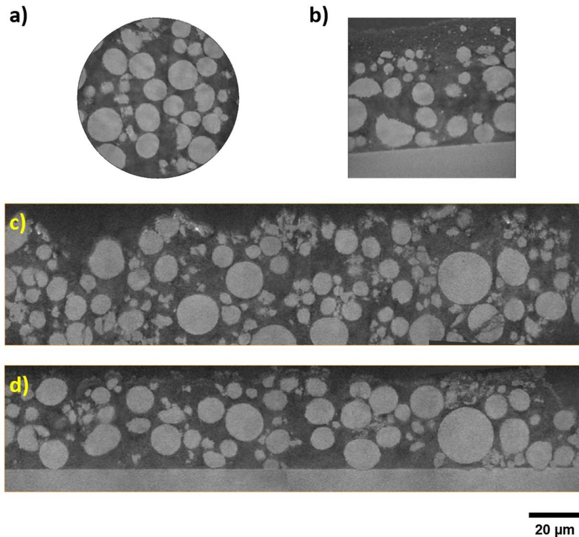
**Figure 7.** Virtual slices of the NMC electrode pillar in the (a) XY and (b) XZ orientation, and electrode tab in the (c) XZ and (d) XY orientation.
