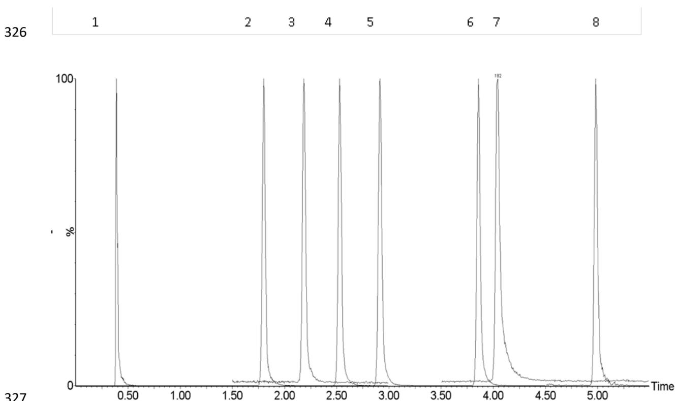
328 **Figure 2.** A reconstructed ion mass chromatogram for the standards of 1= PAP-G 2=APAP-
