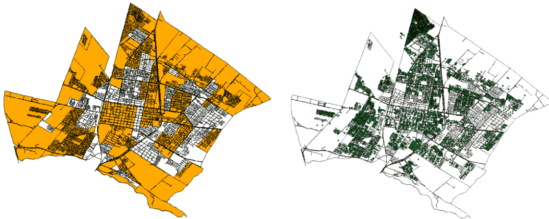
Fig. 4 – The 74.4% of Rancagua was remotely surveyed (highlighted, in the left), where 5,680 data points were collected using IDCT, corresponding to 47,220 structures (right)
