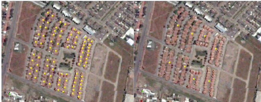
Fig. 3 – Data collection in a remote survey of a residential complex in Rancagua using house-by-house (left) and grouping (right) surveying schemes
