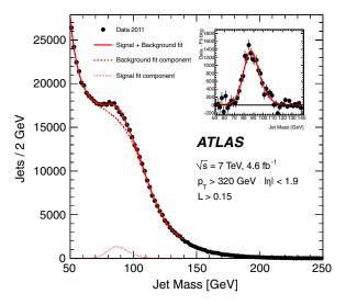
FIG. 45. Binned maximum likelihood fit to the jet mass distribution in data for selected W and Z events reconstructed as one single ungroomed anti- $k_{\rm T}$  R=0.6 jet. From Aad *et al.*, 2014d.
