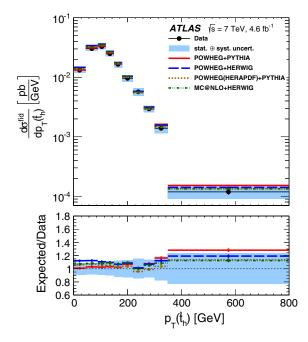
FIG. 41. The small number of top jets identified at high- $p_{\rm T}$  results in very coarse cross section measurement when using the resolved reconstruction technique. Adapted from Aad *et al.*, 2015e.
