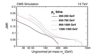
FIG. 13. The CMS jet mass resolution as a function of the ungroomed jet mass  $m_{\rm u}$  in different generated  $p_{\rm T}$  bins. Adapted from Sirunyan *et al.*, 2018o.
