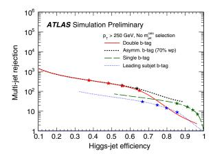
FIG. 30. The rejection of inclusive multijets vs Higgs-jet efficiency using all large-R jets with  $p_{\rm T} > 250$  GeV for single, double, asymmetric, and leading subjet b tagging requirements. From ATLAS Collaboration, 2016k.
