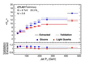
FIG. 20. The average track multiplicity in ATLAS for  $Z/\gamma+$  jets (quark-enriched) and dijets (gluon-enriched). The dashed lines indicate the measurement on the validation samples:  $Z/\gamma+$  2-jets (quark-enriched) and trijets (gluon-enriched). From ATLAS Collaboration, 2016f.
