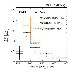
FIG. 35. Particle-level differential  $t\bar{t}$  cross section measurement as a function of the leading jet mass compared to the predictions for three different Monte Carlo event generators. From Sirunyan *et al.*, 2017e.
