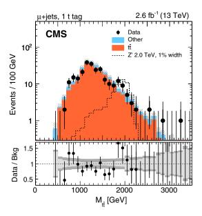
FIG. 49. Invariant mass of the reconstructed  $t\bar{t}$  pair in data and simulation for the lepton + jets channel in the category with one top-tagged jet. From Sirunyan *et al.*, 2017i.
