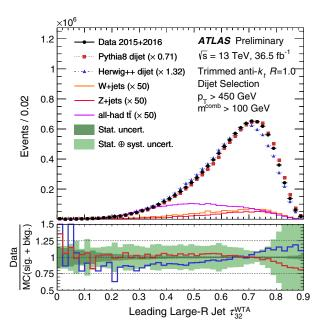
FIG. 14. Measured distribution of the *N*-subjettiness ratio  $\tau_{32}$  calculated on trimmed anti- $k_{\rm T}$ , R=1.0 jets for a dijet selection with  $p_{\rm T}>450$  GeV and  $p_{\rm T}>200$  GeV for the leading and subleading jets, respectively. The data are compared to simulated events, where the dijet samples have been normalized to the signal-subtracted data. From ATLAS Collaboration, 2017f.
