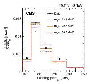
FIG. 36. Normalized particle-level differential  $t\bar{t}$  cross section measurement as a function of the leading jet mass compared to predictions using three different top quark mass values. From Sirunyan *et al.*, 2017e.
