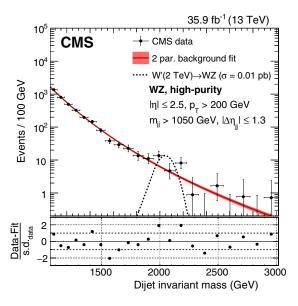
FIG. 47. Dijet invariant mass distribution in the high purity WZ category of the fully hadronic WW, WZ, and ZZ resonance search. The fit under the background-only hypothesis is overlaid. From Sirunyan *et al.*, 2018j.
