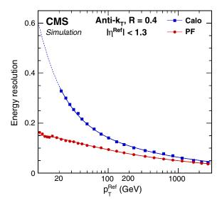
FIG. 3. Jet energy resolution for particle flow (red, lower line) and calorimeter-only (blue, upper line) jets in the barrel region in CMS simulation, with no pileup, as a function of the  $p_{\rm T}$  of the reference jet. From Sirunyan *et al.*, 2017a.
