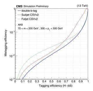
FIG. 31. The misidentification rate for inclusive multijets vs Higgs-jet efficiency using jets with  $300 < p_{\rm T} < 500$  GeV and pruned jet mass 70 < m < 200 GeV for three different b tagging requirements. From CMS Collaboration, 2016e.
