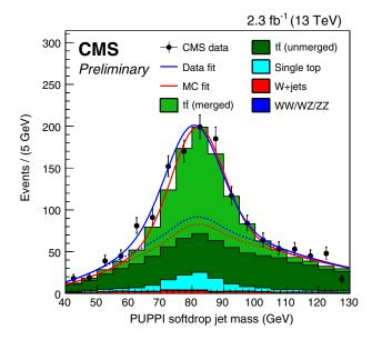
FIG. 12. Jet mass distribution in a sample enriched with lepton + jets  $t\bar{t}$  events, where the hadronic W jet with  $p_{\rm T} > 200$  GeV is selected. From CMS Collaboration, 2017a.
