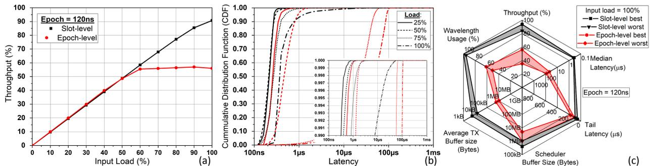
Fig. 2. Slot-level and epoch level schedulers are benchmarked against a) throughput, b) latency and c) numerous performance indicators.
