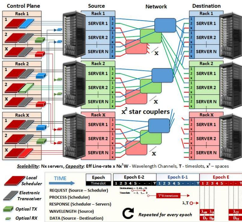
Fig. 1 PULSE network architecture.
