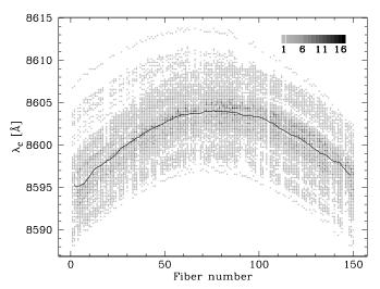
**Figure 3.** Variation of central wavelength as a function of the fiber number for data new to this release. Shades of gray code the number of spectra in a certain bin, as given in the key. The line follows half-point central wavelengths as a function of the fiber number.
