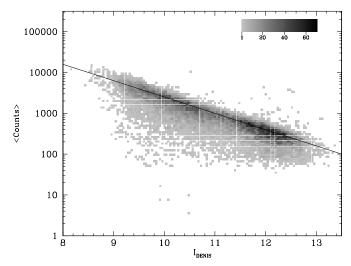
**Figure 4.** Average number of counts per pixel per hour of exposure time as a function of DENIS *I* magnitude. Shades of gray code the number of spectra in a certain bin, as given in the key. The average count level is calculated from the central part of the spectrum only (8449.77 Å  $\leq \lambda \leq$  8746.84 Å). The inclined line follows Equation (1).
