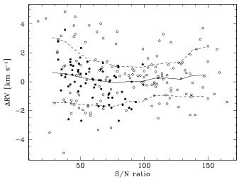
**Figure 12.** Difference of radial velocities as derived by RAVE and by the reference instruments, as a function of the S/N of the RAVE observation. Dots depict individual measurements, the solid line is a running mean (with a boxcar smoothing of  $\pm 15$  in S/N). Similarly, the area between the dashed lines includes 68.2% of the measurements, i.e.,  $\pm \sigma$ . The open symbols are measurements of the GCS stars, while the filled ones mark the other three reference datasets.
