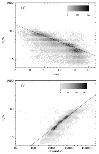
**Figure 8.** Signal-to-noise ratio (S2N) as a function of the DENIS I magnitude (a) and average level of counts per wavelength bin per hour of exposure time (b). Shades of gray mark the number of spectra in a given bin, as explained in the key. The straight line in the top panel follows relation (18), while the one in the bottom panel follows from Equations (1) and (18).
