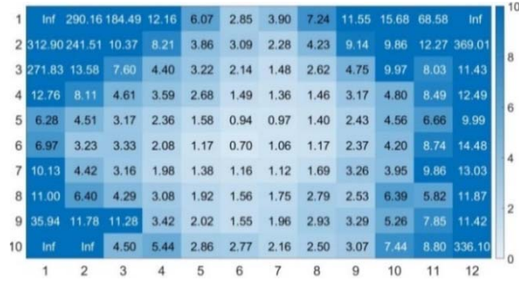
Fig. 6. Pre-Minimiser heatmap of the median localisation error (in cm) across the arena. Each cell represents a 40 cm×40 cm region in the arena,
