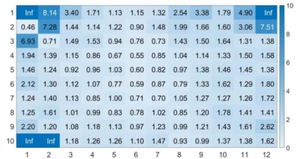
Fig. 9. Post-Filter heatmap of the arena, showing median localisation error (in cm) for 40 cm×40 cm cells.
