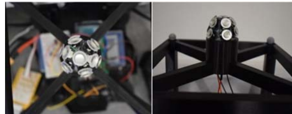
Fig. 1. 'Omnidirectional' US transducer array for the emitter.
