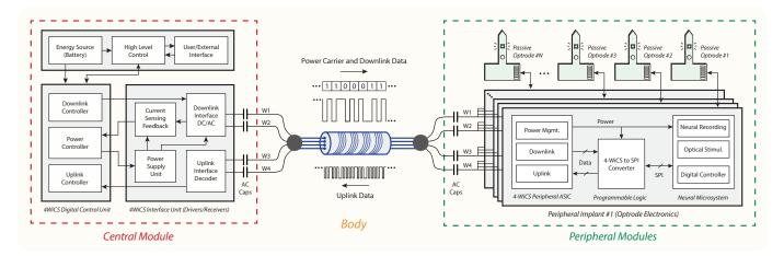
Fig. 2. Block Diagram of 4WiCS system interfacing with corresponding in-body modules at both central and peripheral end.
