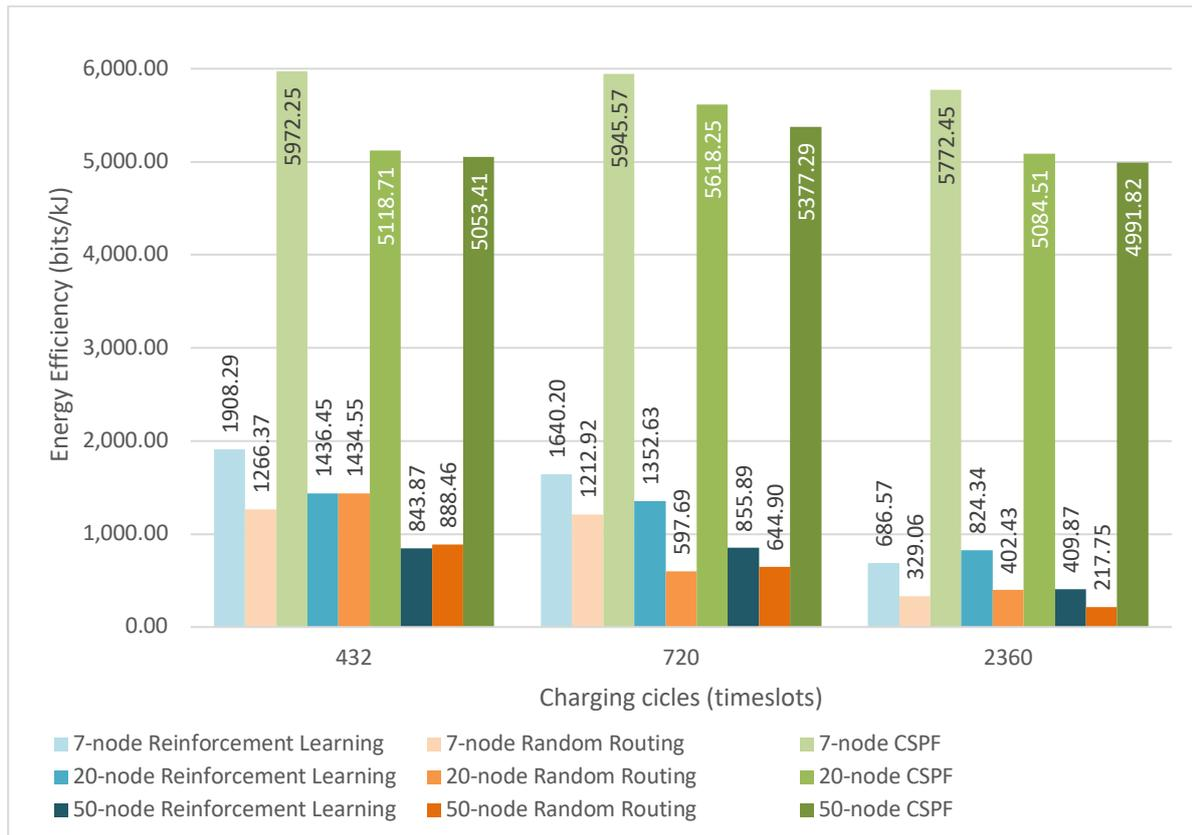
Figure 6.20 Average energy efficiency with different charging cycles
