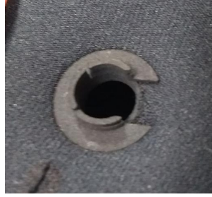
Figure 4.12: Example of 3D printed probe holder in nylon for placement in a cap
