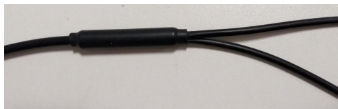
Figure 4.22: Image showing optical source fibre bundle bifurcated after 2 m, with two single fibre bundles for 0.5 m
