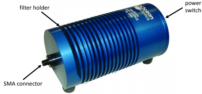
Figure 4.4: Labelled photograph of HL 2000 light source
