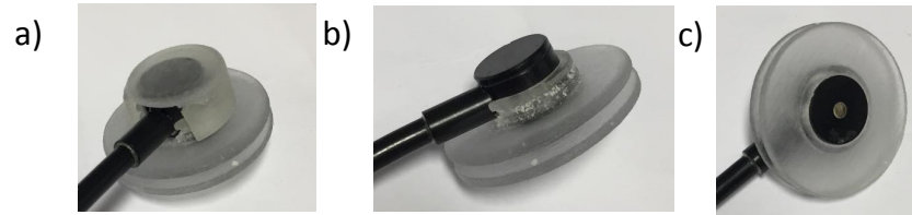
Figure 4.13: Example of 3D printed probe holder in VeroClear. Components consisted of two parts: a base to allow placement into the cap and a top to click into the base and hold the probe in place
