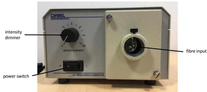
Figure 4.2: Labelled photograph of ORIEL 66088 light source
