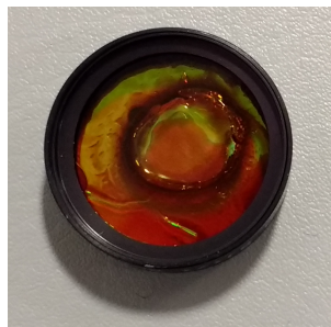
Figure 4.28: Image of high-pass filter burned by ORIEL 66088 light source
