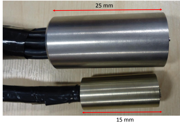
Figure 4.9: Comparison of input ferrule from above for CYRIL and the new system. Bottom shows smaller ferrule size used in CYRIL system, top shows larger ferrule size in new system
