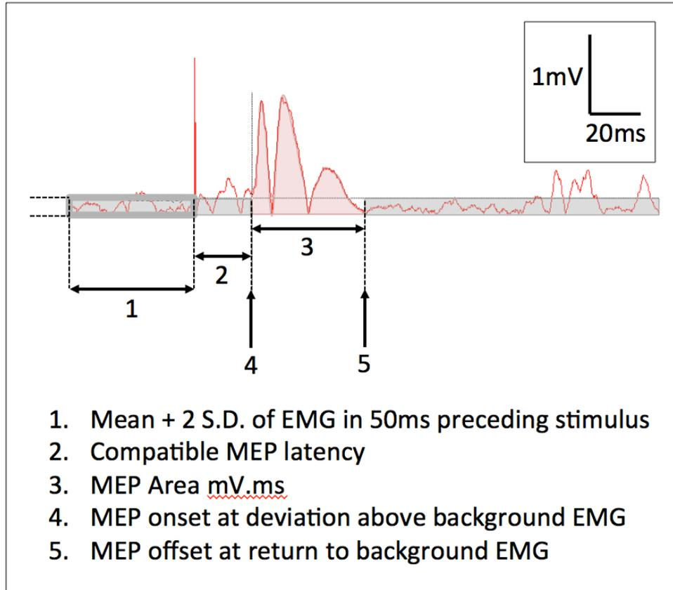
FIGURE 2.2 ILLUSTRATION OF CRITERIA FOR MEASUREMENT OF MEP AREA
