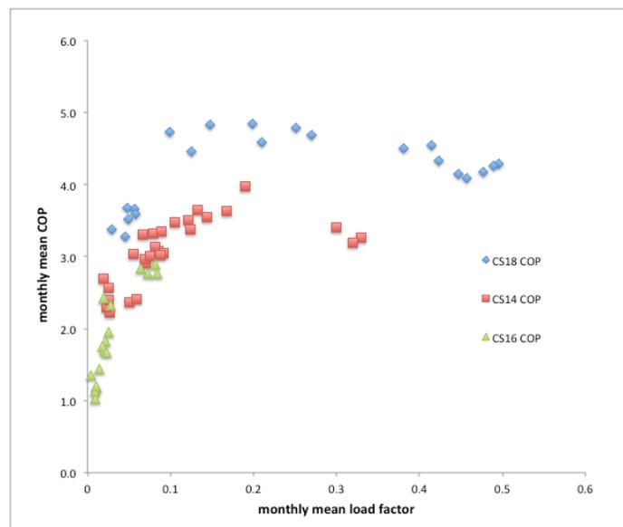
**Fig. 3.** COP versus heat load factor (monthly means) CS14, CS16 & CS18.
