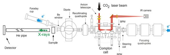
Figure 1: Schematic of the Inverse Compton source and beamline at the Accelerator Test Facility (ATF) at Brookhaven National Laboratory.
