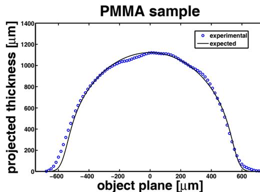
Figure 3: Reconstructed projected thickness at the object plane. PMMA wire, diameter 1124  $\mu\text{m}$ . The reconstruction after phase retrieval is compared to the reconstruction using only absorption.
