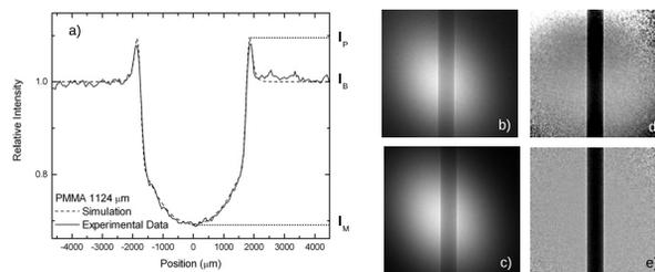
Figure 2: Experimental and simulated images for the PMMA wire. (a) Comparison of the wire profiles in a central portion of the beam. Experimental (b) and simulated (c) images, normalized experimental (d) and simulated (e) images.
