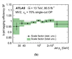
passing the signal region selection. Vertical error bars include data statistical uncertainties only while the green bands correspond to the sum in quadrature of statistical and systematic uncertainties. The dots are located at the mean of the b-jet  $p_T$  distribution in each  $p_T$  bin
