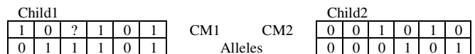
Figure 2: Creation of new binary masks if both children are good. (? denotes randomly generated).
