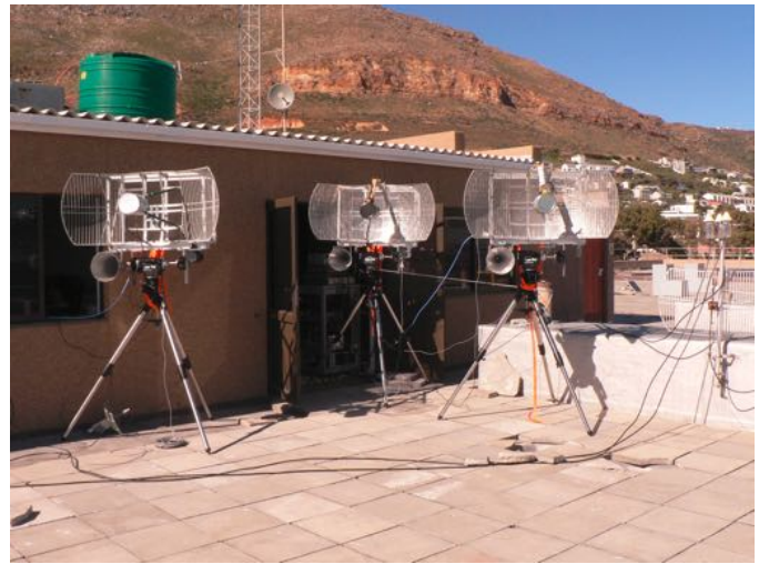
Fig. 2: Dual band radar antenna system, mounted on pedestals.
