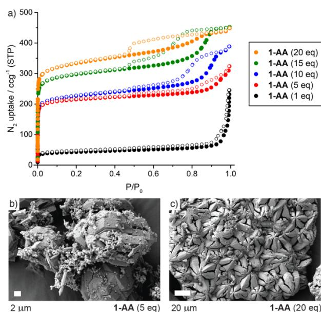
**Figure 4.** a)  $\text{N}_2$  uptake isotherms (77 K, filled symbol adsorption, empty desorption) of samples of **1-AA** prepared with different quantities of AA. SEM images of b) **1-AA** (5eq) showing the presence of large intergrown blocks of MIL-126(Fe) alongside hexagonal needles of MIL-88D(Fe), and c) **1-AA** (20 eq) showing only intergrown sheets of MIL-126(Fe).
