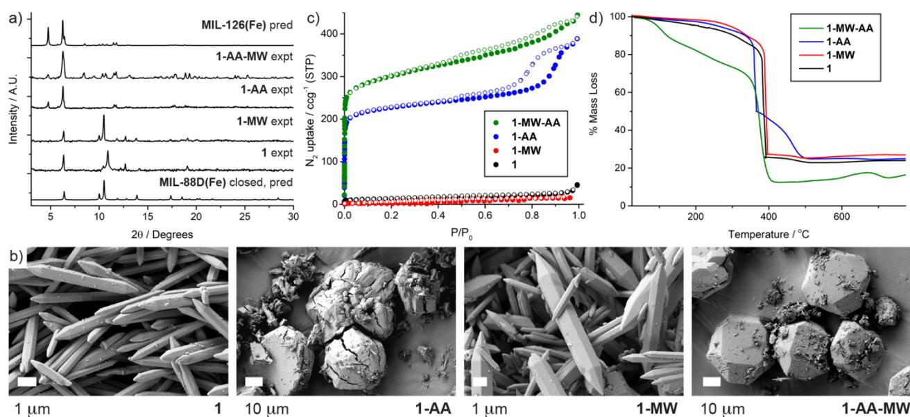
**Figure 2.** a) Stacked PXRD patterns of samples of **1** compared to predicted patterns for MIL-88D(Fe) in the closed state and MIL-126(Fe). b) SEM images of the samples of **1** showing morphology differences resulting from modulation. c)  $\text{N}_2$  uptake isotherms (77 K) for the samples of **1** (filled symbols indicate adsorption, empty symbols desorption) Interpenetration is indicated by porosity. d) Thermogravimetric analyses of the samples of **1**.
