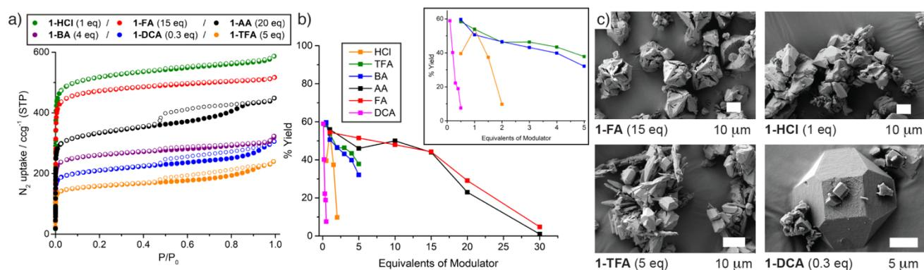
**Figure 5.** a) N<sub>2</sub> uptake isotherms (77 K, filled symbol adsorption, empty desorption) of optimal samples of **1** prepared with each modulator. b) Plot of reaction yields against modulator equivalents for each synthetic system, showing decrease in yield as more modulator is added. c) SEM images showing differing morphologies obtained with different modulators.
