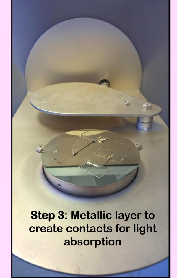
Figure 2: Fabrication Step by Step
