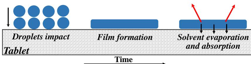
Figure 4.1: Outline of the coating application process during pharmaceutical coating.
