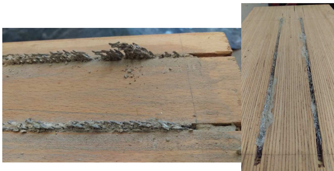
Figure 27 - Failure planes of the connectors in Specimen A at (a) the surface of the timber joist, and (b) the timber interlayer.
