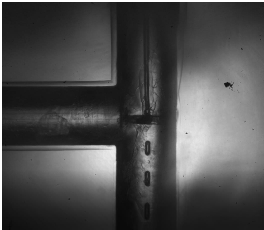
Supplementary Information 1. Microbubble formation inside T-junction channel.
