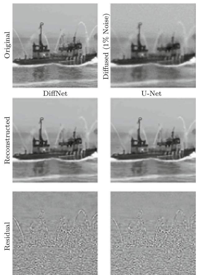
**Fig. 9** Comparison of reconstruction quality for reconstruction from 1% noise contaminated nonlinear diffused image. Both networks are trained on the full set of 90,000 images. PSNR: DiffNet 34.96, U-Net 35.27
