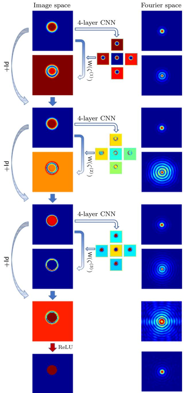
**Fig. 5** Illustration of the deconvolution process with three layers of DiffNet. The left column shows the processed image and intermediate steps. The right column shows the corresponding absolute value of Fourier coefficients. All images are plotted on their own scale
