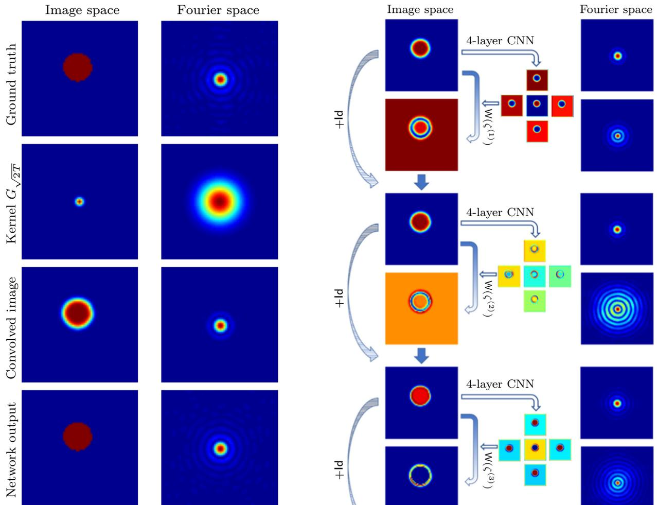
**Fig. 4** Illustration of the deconvolution problem for a simple ball. Left column shows the image space, and the right column shows the corresponding absolute value of the Fourier coefficients. All images are plotted on their own scale
