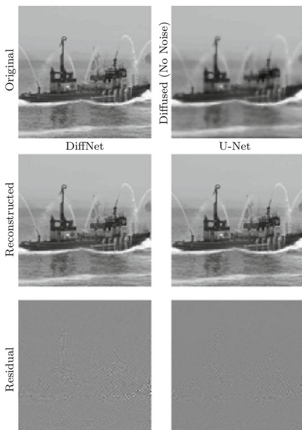
**Fig. 8** Comparison of reconstruction quality for reconstruction from nonlinear diffused image without noise. Both networks are trained on the full set of 90,000 images. PSNR: DiffNet 65.34, U-Net 61.08
