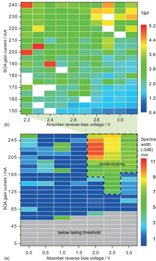
**Fig. 5.** Color-coded map of (a) optical spectral width (-3 dB) and (b) time-bandwidth-product (TBP) (within a selected biasing regime) in dependence on the injection current and absorber reverse bias.
