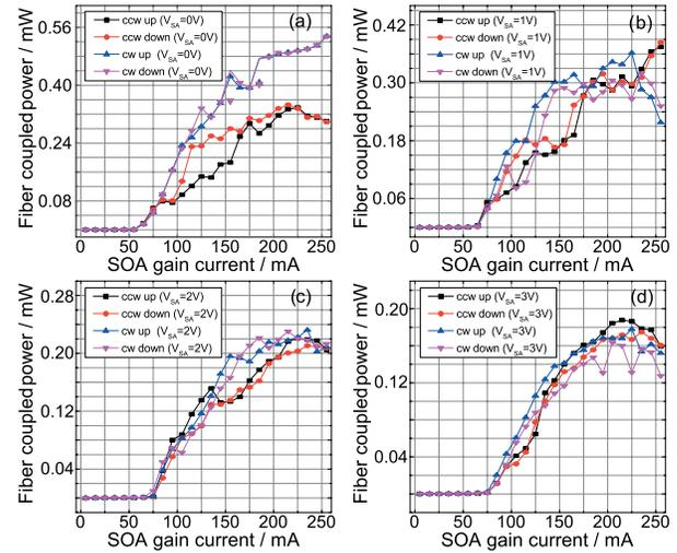
**Fig. 2.** Fiber-coupled average optical laser output power versus  $I_{SOA}$  at (a)  $V_{SA} = 0$  V, (b)  $V_{SA} = 1$  V, (c)  $V_{SA} = 2$  V and at (d)  $V_{SA} = 3$  V. Fiber coupling losses are  $\approx 5$  dB. Clockwise (CW, Out 4), counter-clockwise (CCW, Out 1) emission, „up“ denotes increasing and „down“ decreasing injection current. Note the different y-axis scaling.
