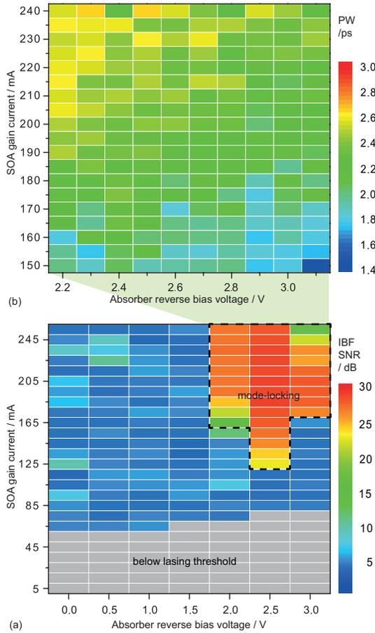
**Fig. 3.** Color-coded map of (a) Intermode beat frequency signal-to-noise ratio (IBF SNR) and (b) optical pulse width (PW) (within a selected biasing regime) in dependence on injected gain current and absorber reverse bias voltage.
