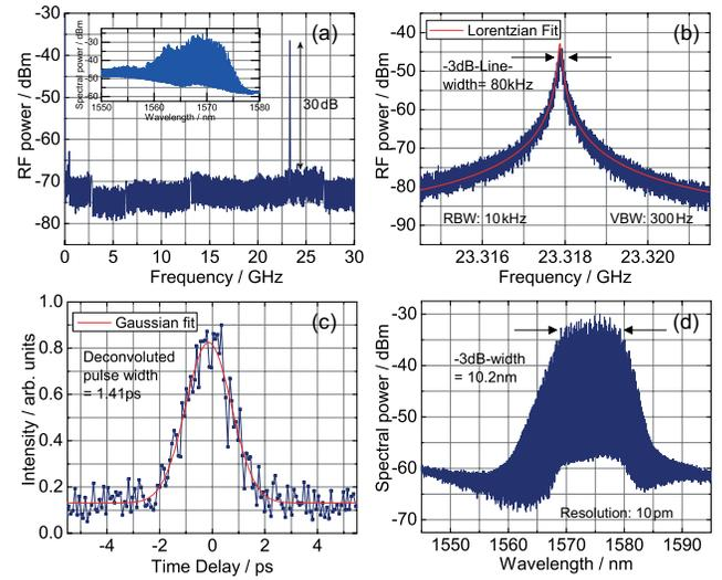
**Fig. 4.** (a) Full-span RF spectrum for  $I_{SOA} = 150$  mA,  $V_{SA} = 3.1$  V. The inset shows the optical spectrum for the same bias conditions. (b) Zoom into (a) and Lorentzian fit. (c) Auto-correlation trace at  $I_{SOA} = 150$  mA and  $V_{SA} = 3.1$  V. Scan range: 10 ps. (d) Optical spectrum at  $I_{SOA} = 215$  mA,  $V_{SA} = 2.0$  V.
