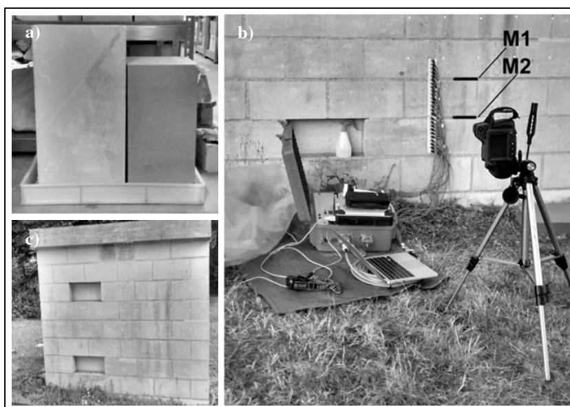
Fig. 1: The monoliths (left, limestone; right, sandstone) (a) and the traditional masonry construction (b). An example of the simultaneous instrument set-up with positions of the mortar joints: M1 and M2 (c).
