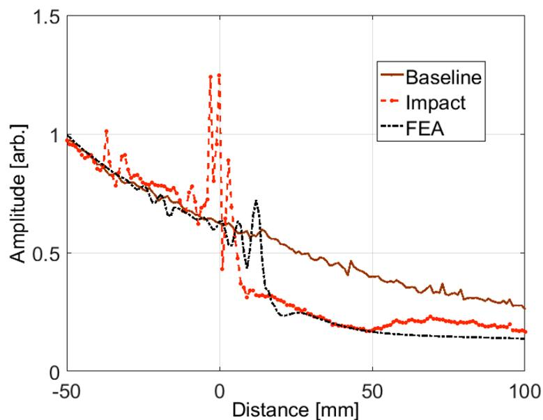
**Figure 4:** Guided wave amplitude on line across defect;  $A_0$  guided wave mode, 100 kHz excitation frequency; baseline measurement (solid, brown), measurement across impact damage (dashed, red), FE simulation for delamination (dash-dot, black).
