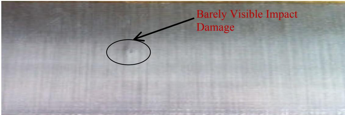
**Figure 1:** Composite specimen with barely visible impact damage (indent and fibre fracture) marked.
