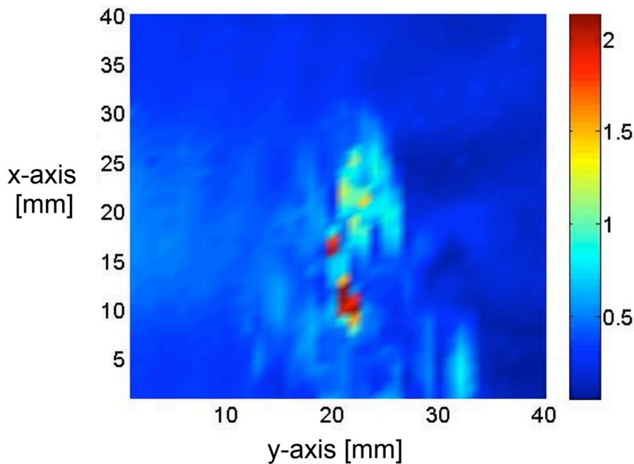
**Figure 3:** Guided wave image of area around impact damage;  $A_0$  guided wave mode, 100 kHz excitation frequency; 1 mm step size; maximum amplitude of time trace (Hilbert transform).
