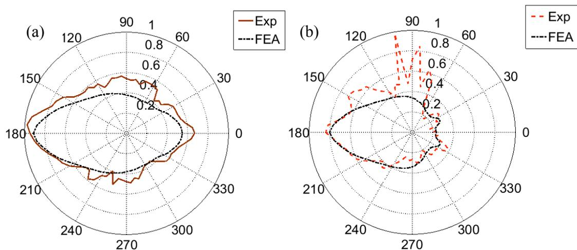
**Figure 5:** Guided wave amplitude on circle around defect;  $A_0$  guided wave mode, 100 kHz excitation frequency; (a) baseline measurement (solid, brown), FE simulation without defect (dash-dot, black); (b) measurement around impact damage (dashed, red), FE simulation for delamination (dash-dot, black).
