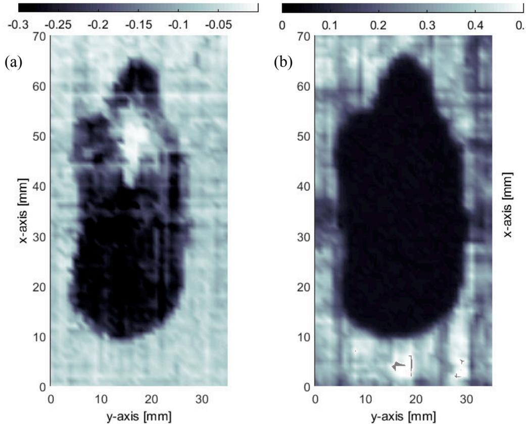
**Figure 2:** Ultrasonic immersion C-scan of damaged composite specimen (scan area: 70 mm x 35 mm, step size: 1mm); amplitude of ultrasonic signal, 10 MHz unfocussed immersion transducer: (a) pulse reflection; (b) double-through transmission.
