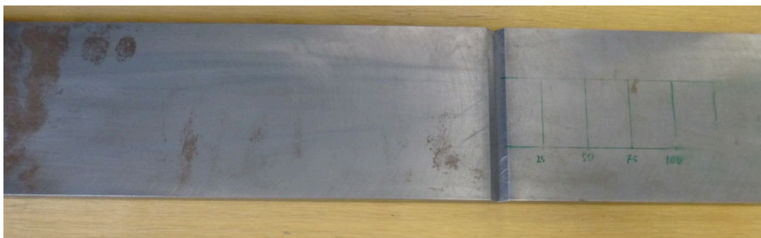
Figure 2. Photograph of steel specimen (11 mm thickness) with V-notch (maximum depth: 5 mm, opening angle: 90°).
