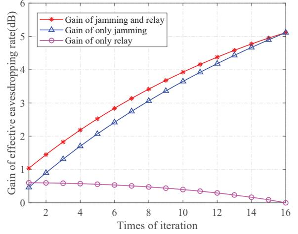
Fig. 3: The gain of effective eavesdropping rate of three schemes for each iteration when  $N = 50$ ,  $D = 1800$ m.
