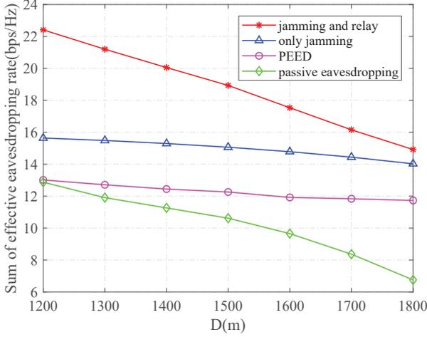
Fig. 2: The sum of effective eavesdropping rate of four schemes by beginning distance  $D$  meters between the legitimate eavesdropper and the MST( $N=50$ ).
