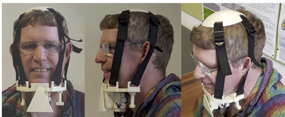
Fig. 3. (Color online) Photo of the headset in place. Left = front, middle = side, right = isometric view.
