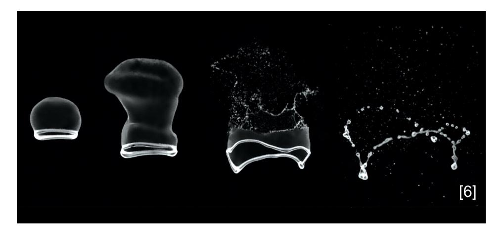
**Industrial application:** Such modelling informs the physical understanding of how particles interact with water on aircraft components and how particles progress after impact.
