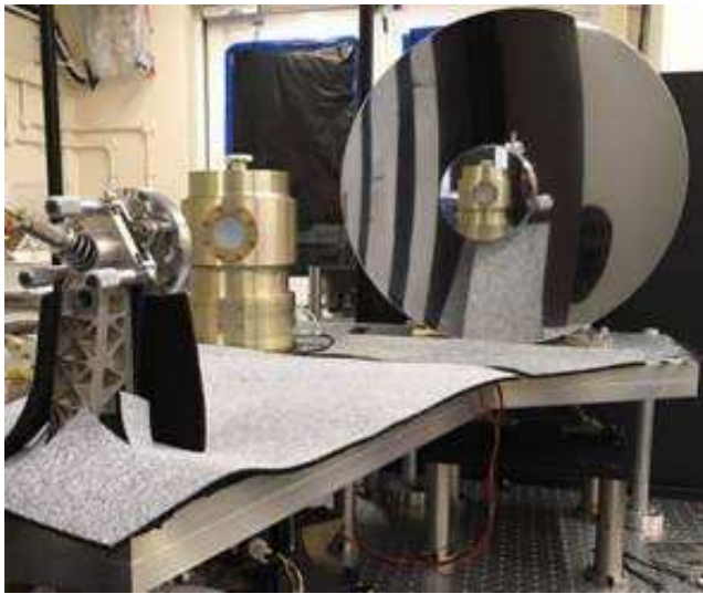
Fig. 2. (Top) Top-down CAD illustration of the LOCUS breadboard system: A, B = telescope optics, C = cryocooler. (Bottom) Photograph of fully-constructed system.
