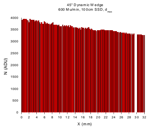
Figure 2 Dose distribution profile of a "Dynamic Wedge" created by moving MLC collimators ala dIMRT.
