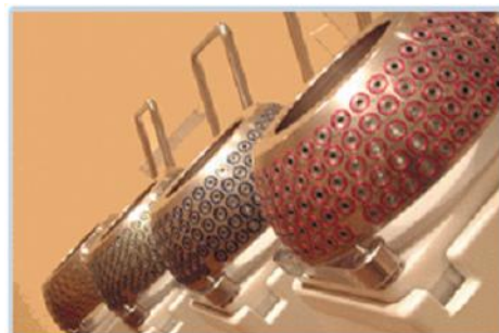
Figure 6 Detail of collimator helmets for a gamma knife system [12].
