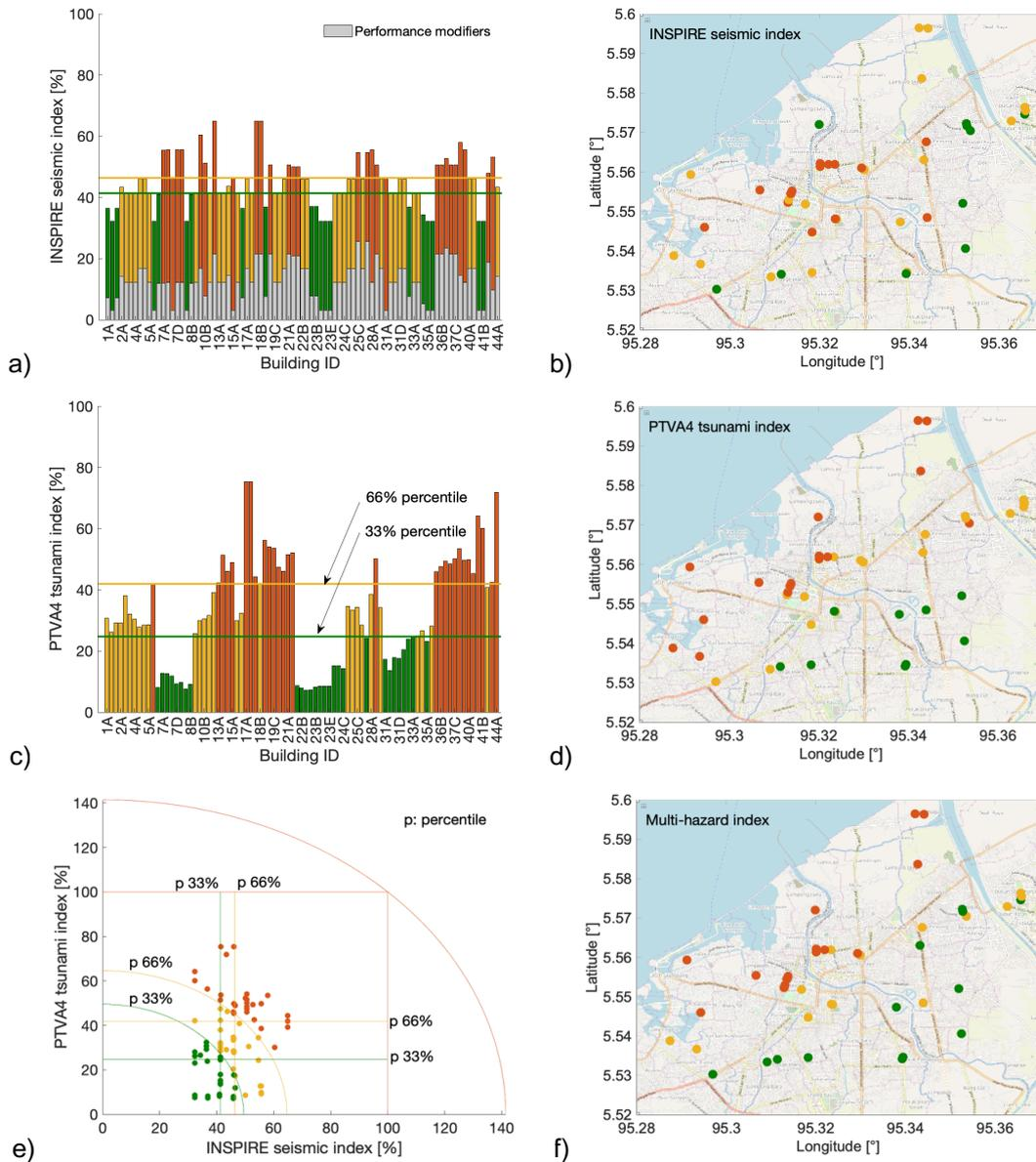
Figure 6. Application to the seismic and tsunami indices to 85 RC school buildings in Banda Aceh, Indonesia. a,b) seismic indices; c,d) tsunami indices; e,f) multi-hazard indices.
