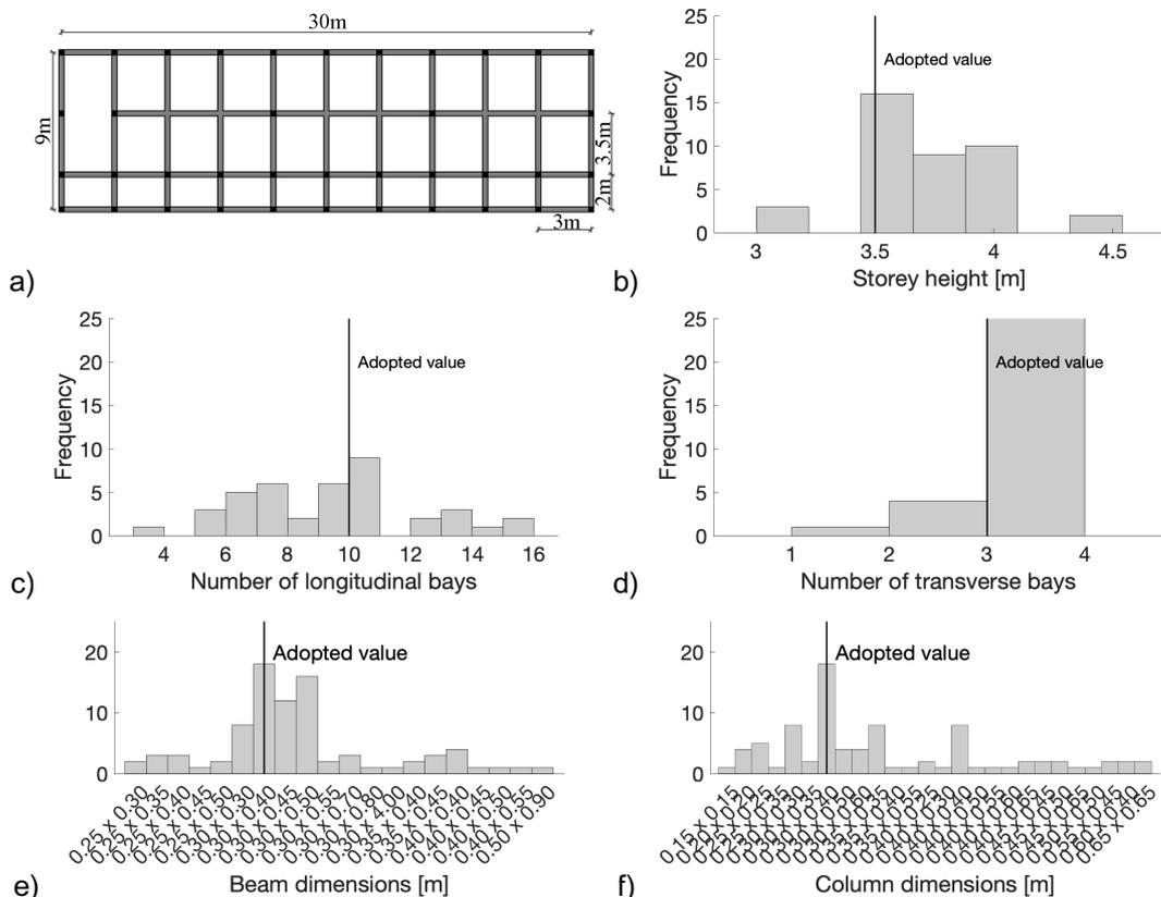
Figure 5. Two-storey, rectangular buildings: geometry trends and adopted values for the archetype building. a) plan view of the archetype building; b-h) histograms of the geometric parameters.
