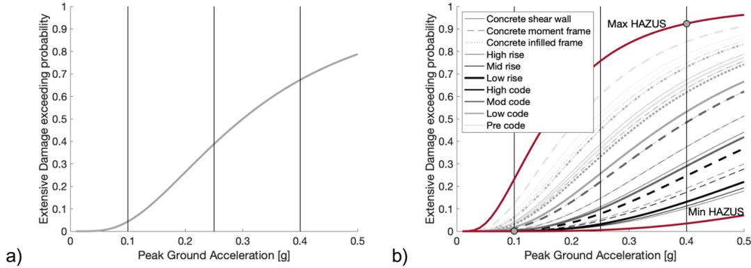
Figure 2. a) Example baseline score for a given archetype building typology. b) HAZUS fragility curve database related to the Extensive Damage limit state for RC buildings.
