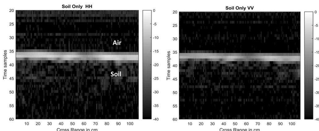
**Fig. 5** Scene 1—soil only in horizontal polarisation (left) and vertical polarisation (right)
