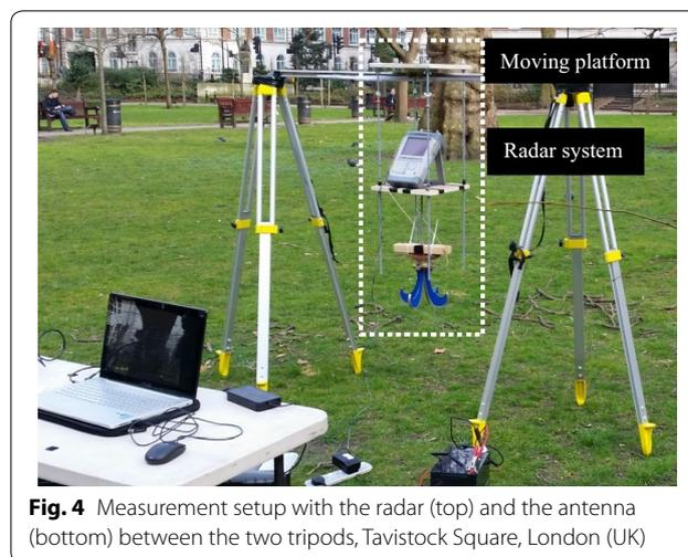
**Fig. 4** Measurement setup with the radar (top) and the antenna (bottom) between the two tripods, Tavistock Square, London (UK)
