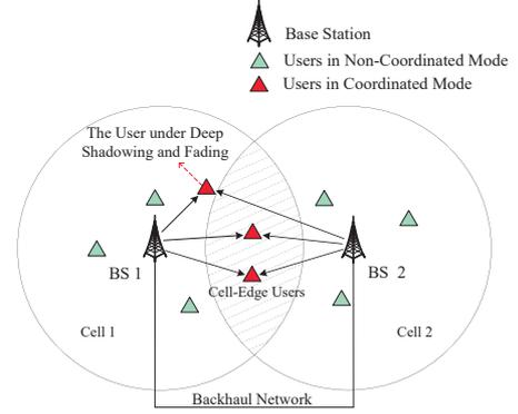
Fig. 1. System model of multi-cell coordinated NOMA systems.
