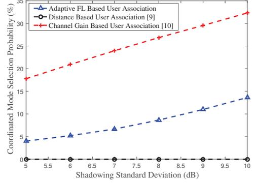
Fig. 4. Coordinated mode selection probability of cell center users under deep shadowing in multi-cell coordinated NOMA.
