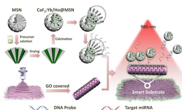
Fig. 1 Schematic illustration of the synthesis of biosensing membrane and miRNA detection.
