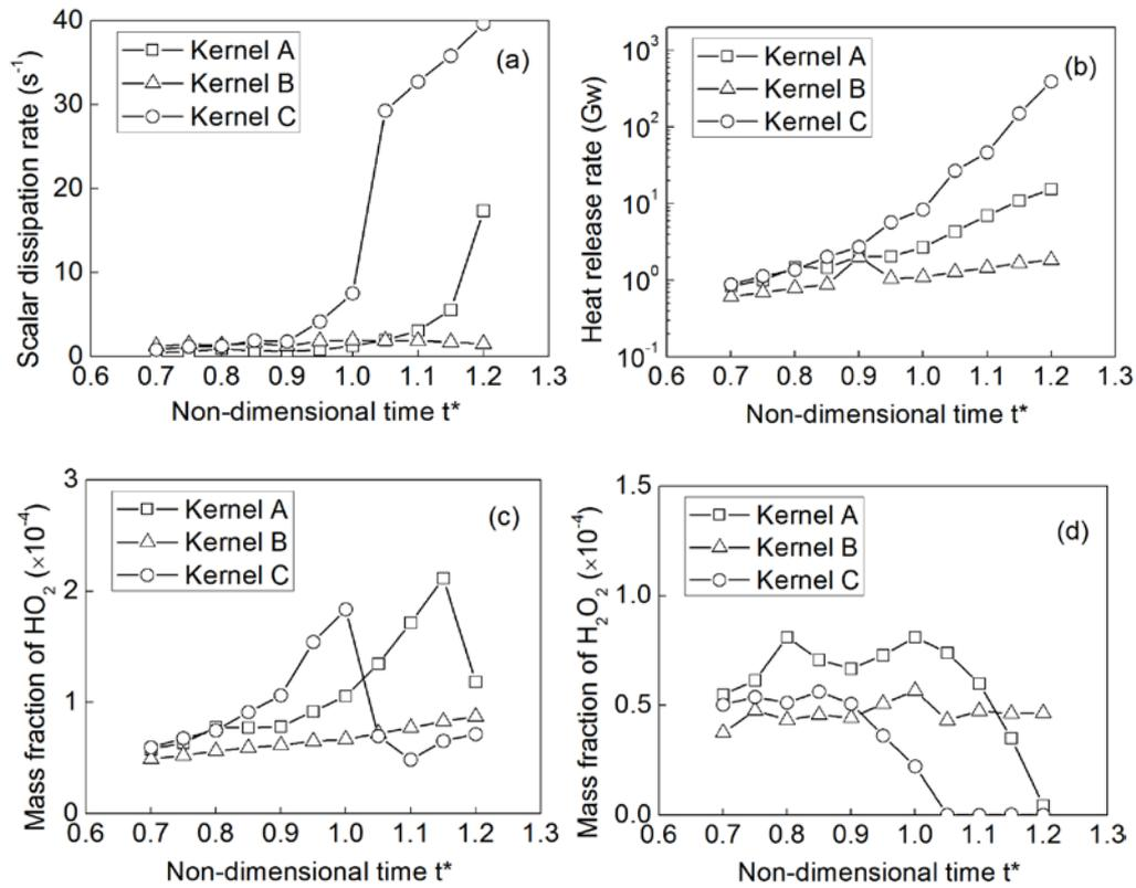
**Figure 10.** Evolution of different scalars in different ignition kernels: (a) scalar dissipation rate (b) heat release rate (c) mass fraction of  $\text{HO}_2$  (d) mass fraction of  $\text{H}_2\text{O}_2$
