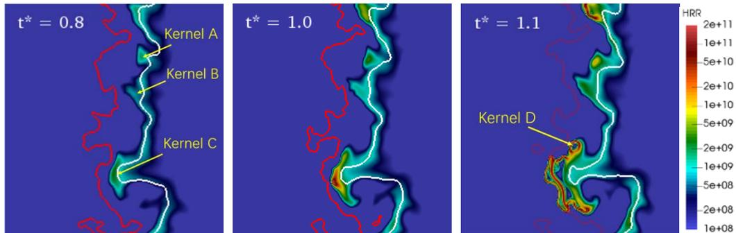
**Figure 6.** Instantaneous views of heat release rate (HRR) for a time sequence:  $t^* = 0.8$  (left),  $1.0$  (middle), and  $1.1$  (right). The white line represents the  $\xi_{MR} = 0.07$  iso-surface, while the red line represents the  $\xi_{ST} = 0.56$  iso-surface. Three ignition kernels are highlighted.
