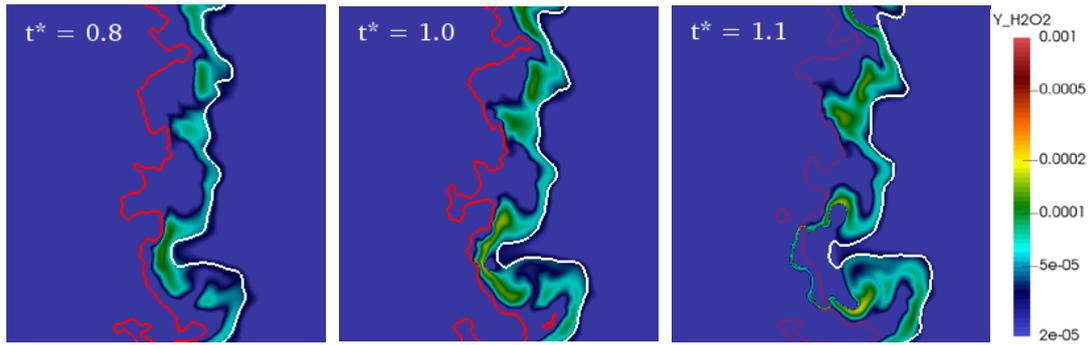
**Figure 8.** Instantaneous views of  $H_2O_2$  mass fraction ( $Y_{H_2O_2}$ ) for a time sequence:  $t^* = 0.8$  (left),  $1.0$  (middle), and  $1.1$  (right). The white line represents the  $\xi_{MR} = 0.07$  iso-surface, while the red line represents the  $\xi_{ST} = 0.56$  iso-surface.
