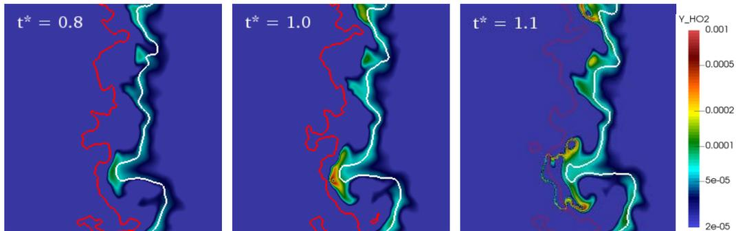
**Figure 7.** Instantaneous views of  $\text{HO}_2$  mass fraction ( $Y_{\text{HO}_2}$ ) for a time sequence:  $t^* = 0.8$  (left),  $1.0$  (middle), and  $1.1$  (right). The white line represents the  $\xi_{MR} = 0.07$  iso-surface, the red line represents the  $\xi_{ST} = 0.56$  iso-surface.
