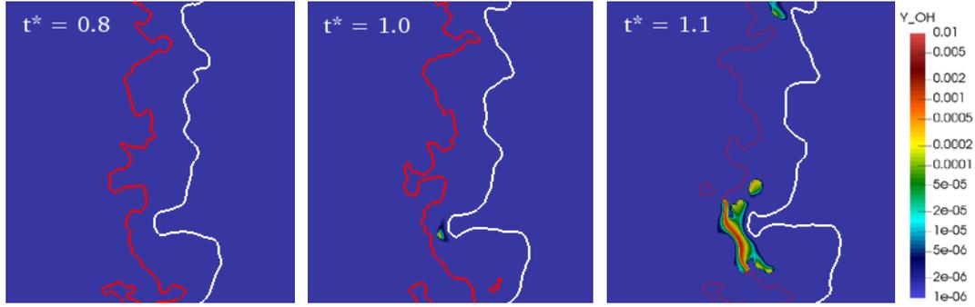
**Figure 9.** Instantaneous views of OH mass fractions for a time sequence:  $t^* = 0.8$  (left),  $1.0$  (middle), and  $1.1$  (right).
