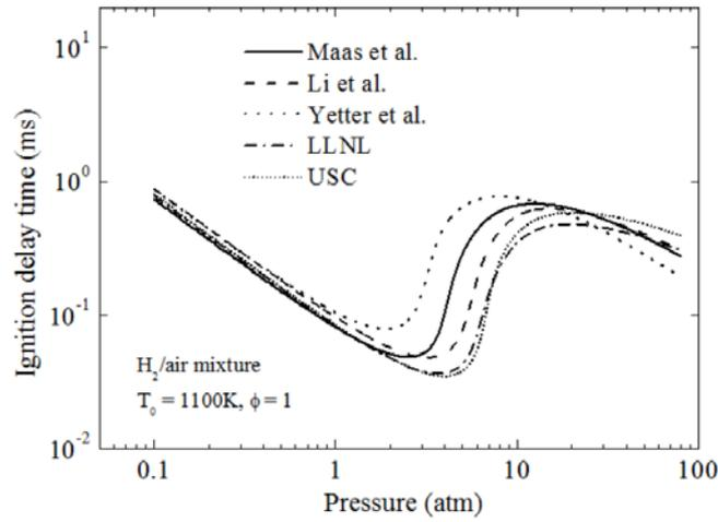
**Figure 2.** Calculations of autoignition time in homogeneous hydrogen-air mixtures at different pressures using various detailed mechanisms: Maas et al. [35], Li et al. [41], Yetter et al. [42], LLNL mechanism [43] and USC mechanism [44].
