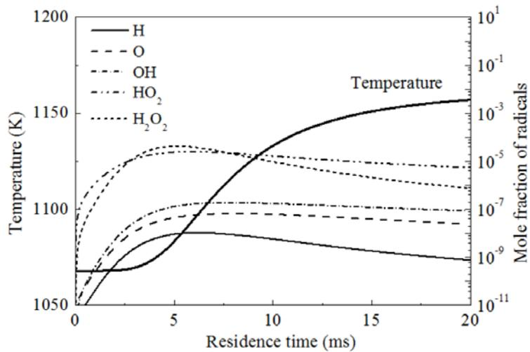
**Figure 4.** Evolution of temperature and radicals in HMI corresponding to the most reactive mixture fraction  $\xi_{MR} = 0.05$ .
