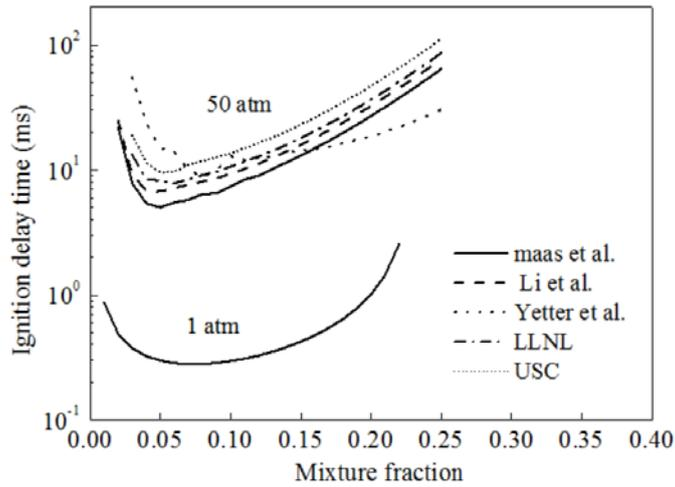
**Figure 3.** Autoignition delay time in HMI versus mixture fraction with various mechanisms: Maas et al. [35], Li et al. [41], Yetter et al. [42], LLNL mechanism [43] and USC mechanism [44].
