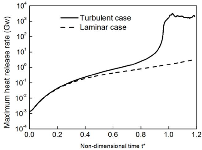
**Figure 5.** Comparison of evolution of maximum heat release rate for turbulent and laminar cases.
