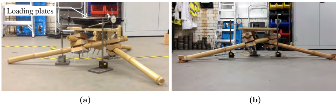
Figure 8.34: (a) Set-up of loading test 1. (b) Set-up of loading test 2.
