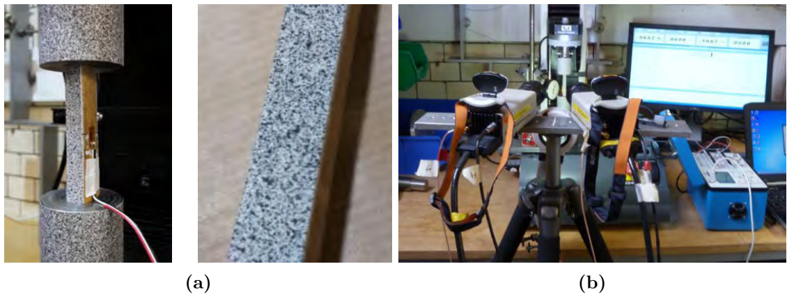
Figure 6.1: (a) Small coupon prepared with spray paint for DIC analysis. (b) Set-up of the cameras for the DIC measurements.
