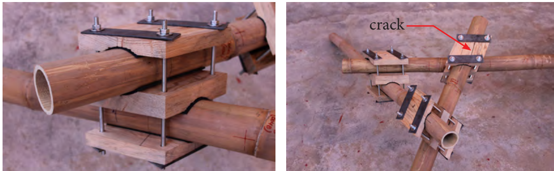
Figure 23: Assembly of timber connection with a metal sill on top of timber blocks, and crack on timber block.
