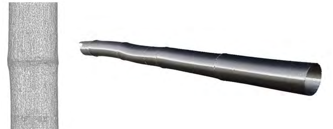
Figure 4.3: Output of the mesh of the outside geometry of the culm.
