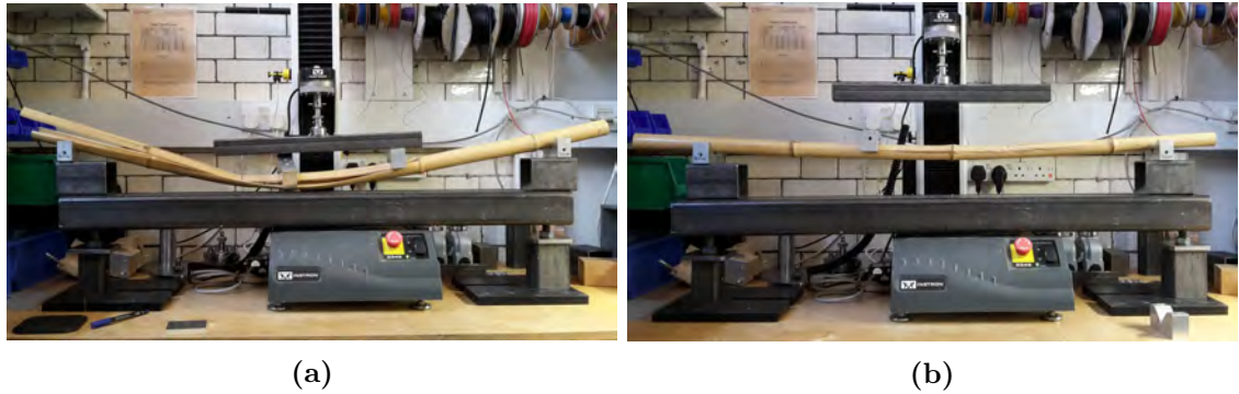
Figure 6.20: Failure of bamboo culms under 4-point bending loads(a) Bottom culm (b) Top part.
