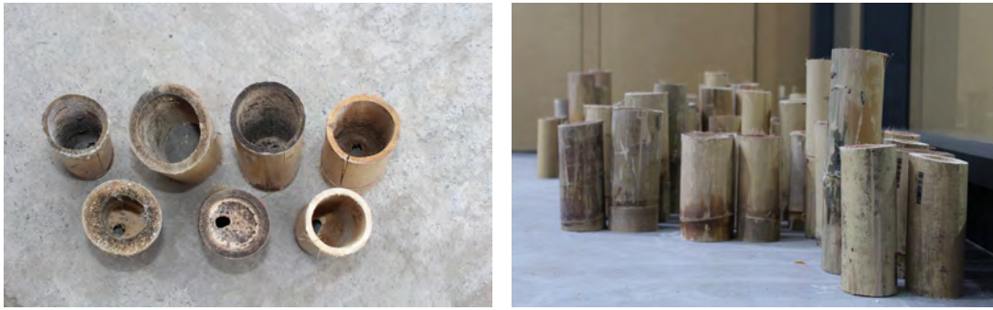
Figure 6: (a) Discarded end sections. (b) End sections ready for fabrication of samples.
