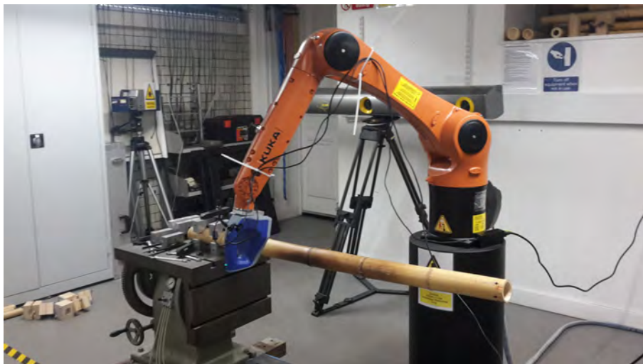
Figure 4.2: Artec scanner mounted on a kuka robot for preliminary investigations on the scanning of bamboo culms.
