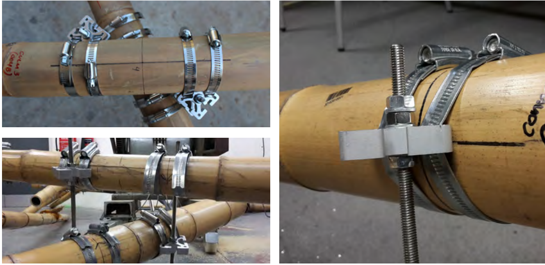
Figure 8.16: Aluminium connection assembled to assess fitting of components.
