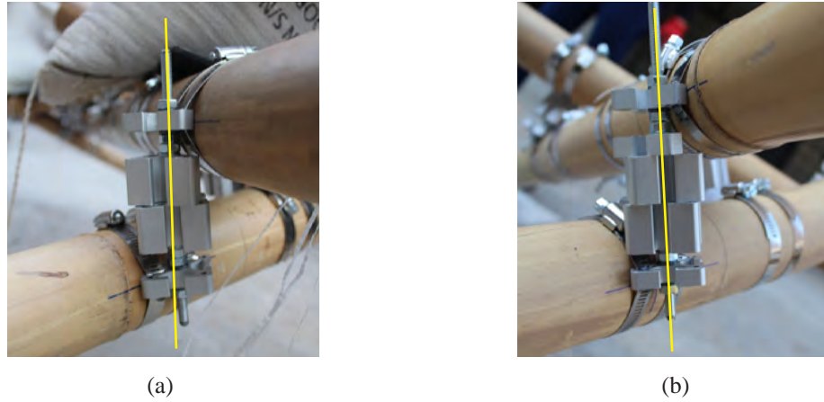
Figure 8.48: Deformations of the vertical components in aluminium connection under vertical load. (a) Loaded connection. (b) Unloaded connection.
