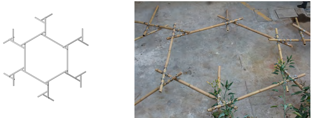
Figure 28: Reciprocal structure assembled using modular sequence.
