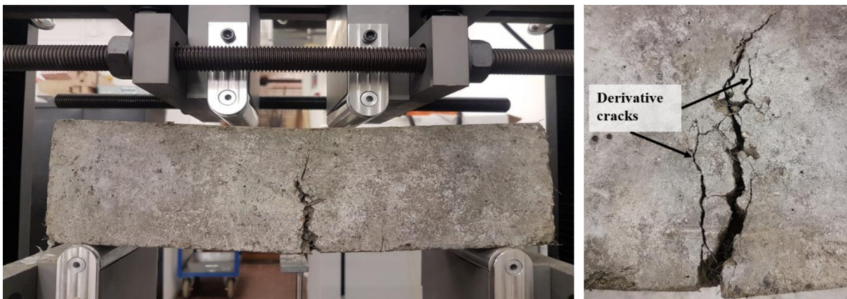
Fig. 10. Typical crack propagation of RSFRAM under four-point bending and post-failure crack pattern near midspan
