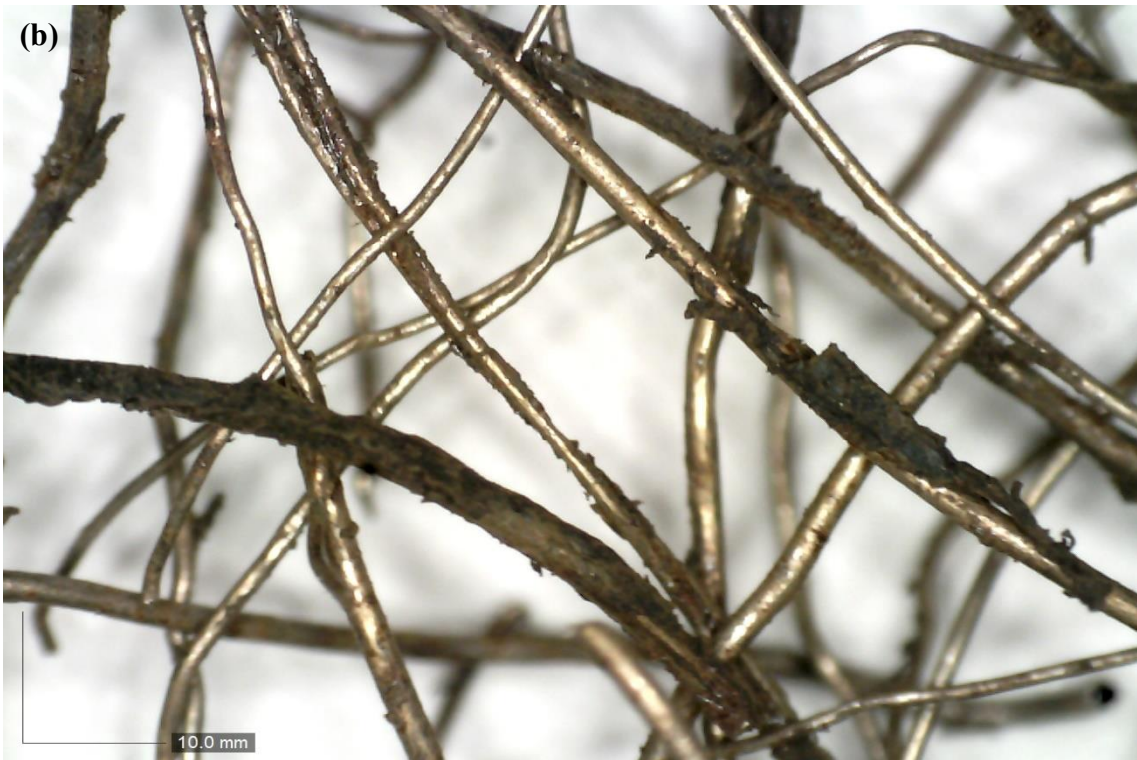
Fig. 3. Recycled tyre steel fibre (RTSF): (a) picture; (b) image taken by digital microscope (Dino-Lite Edge AM73115MZT)
