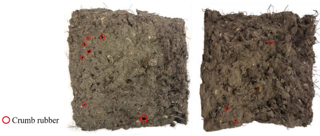
Fig. 15. Example of failed sections of a RSFRAM sample with 1.0 vol.% RTSF addition
