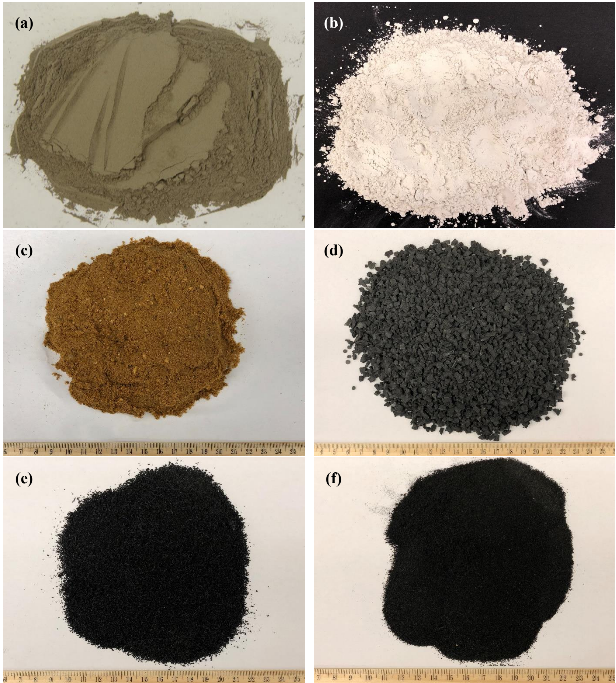
Fig. 1. Raw materials used in this study: (a) FA; (b) GGBS; (c) sand; (d) 2-6 mm CR; (e) 12 mesh (i.e. 1.68 mm) CR; (f) 30 mesh (i.e. 0.595 mm) CR
